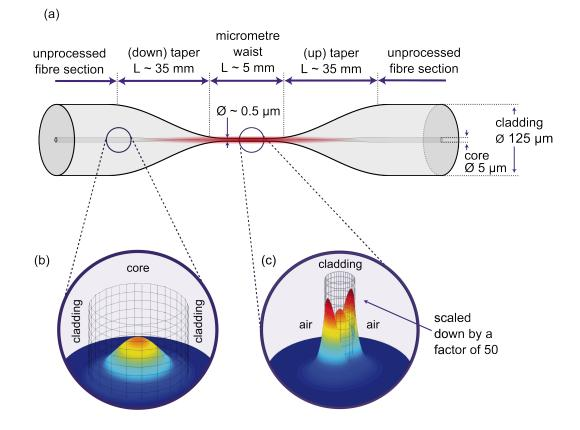
Figure 1.4: (a) Sketch of an OMF. The two bottom images show the intensity distribution of the quasi-linearly polarized  $HE_{11}$  mode in the unprocessed single-mode fibre (b) and in the OMF (c). The intensity distributions were calculated using our MATLAB toolbox [27].
