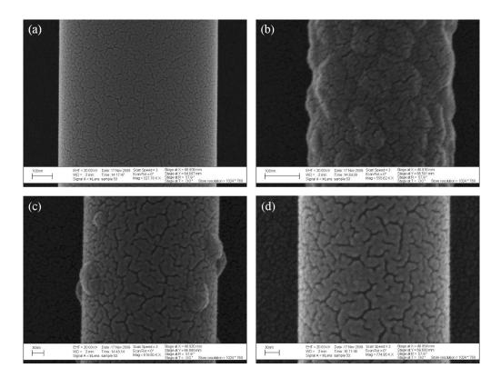
Figure 2.15: SEM images of the damaged sample G. No phase matching and therefore no harmonic light could be achieved within our laser wavelength range for (a) a very thick section of the taper ( $d = 0.790 \ \mu\text{m}$ ) and (d) for the waist ( $d = 0.319 \ \mu\text{m}$ ). Images (b) and (c) show the taper sections where harmonic light was generated ( $d = 0.430 \ \mu\text{m}$  and  $d = 0.355 \ \mu\text{m}$ , respectively). The fissures on all images are due to the gold coating.
