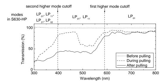
Figure 1.9: Transmission before, during and after pulling of a spliced S630-HP – SM800 – S630-HP fibre with a final waist diameter of 0.44  $\mu$ m and a waist length of 5 mm. The two vertical dashed lines indicate the higher mode cutoff wavelengths in the S630-HP fibre.
