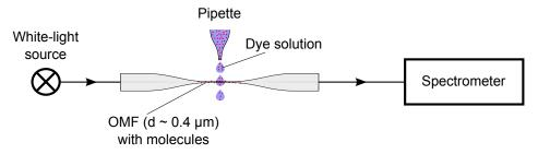
Figure 3.8: Deposition and detection of organic molecules.
