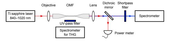
Figure 2.6: Experimental setup for SHG and THG measurement.
