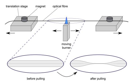
Figure 1.6: The commercial single-mode optical fibre is fixed on two translation stages with strong magnets. By heating the fibre with a moving hydrogen-oxygen flame and simultaneous pulling at both ends the optical fibre is tapered to the desired shape. The two insets show the optical fibre before and after tapering.
