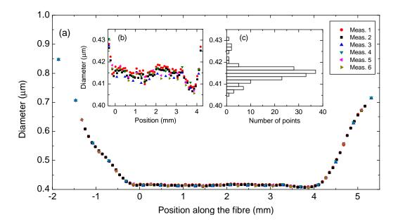
Figure 2.13: (a) Diameter profile of an OMF (sample A) obtained by SEM measurements of different beam energies and scan speeds, designated Meas. 1 to Meas. 6. The position of zero along the fibre is arbitrary. (b) Vertically enlarged picture of the waist. A short thinner region at the right end of the waist can be seen. All the individual points are measured with an accuracy of  $< 7 \times 10^{-3}$  µm. (c) Diameter histogram.
