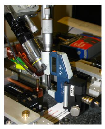
Figure 5.2. Measurement of the OMF waist diameter with the micrometer.
