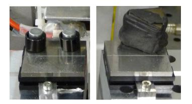
Figure 3.5. Fiber fixation mechanisms of the previously used fiber fabrication setup, strong magnets provide the clamping force.
