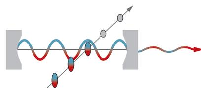
**Cavity memory effects:** Stimulated emission causes traversing atomic dipoles to deliver their radiation field into the resonator field. Subsequent atoms show collective radiation phenomena because the long-lived cavity field stores the field and thus memorizes preceding atoms.
