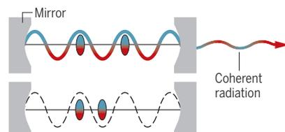
**Interfering atomic radiators:** Two phase-coherently driven atoms emit their radiation field into the cavity constructively (superradiantly) for  $2\pi$  phase difference and destructively (no emission) for  $\pi$  phase difference.
