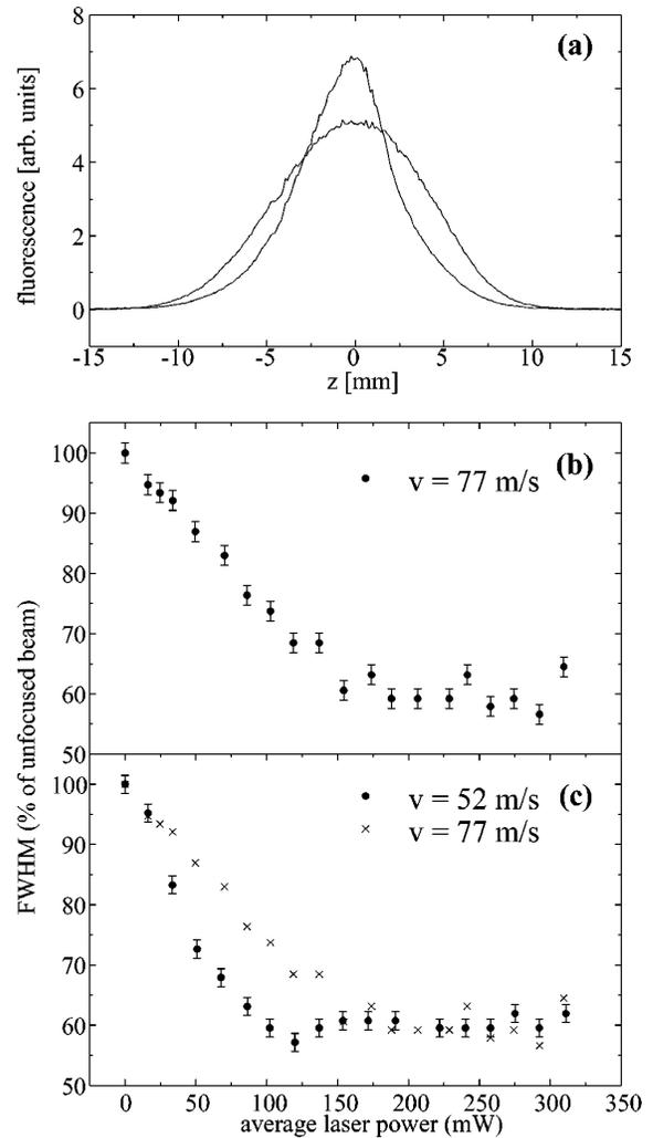
FIG. 4. Focusing of the atomic beam: (a) atomic beam profiles in the focal plane for  $v = 52$  m/s; (b) and (c) normalized widths of the atomic beam in the detection zone vs average laser power for  $v = 77$  m/s and  $52$  m/s, respectively. In (c) the data for  $v = 77$  m/s are replotted (crosses) for comparison. Error bars denote the reading uncertainty.
