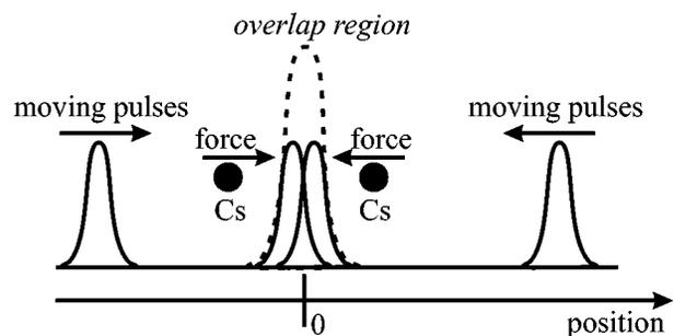
FIG. 1. Counterpropagating pulses overlapping in the vicinity of the atomic beam. Atoms at positive (negative) position experience a stimulated light force towards the left (right). In the region around zero position where the pulses partially overlap, the restoring force increases linearly with the distance to the overlap center.
