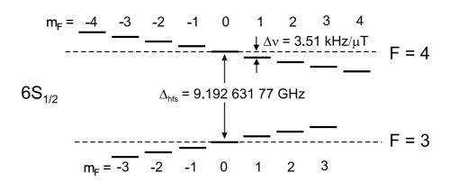
**Figure 4.7**: Zeeman splitting of magnetic sublevels of the  $6^2S_{1/2}$  ground state of cesium. The energy of the magnetic sublevels is shifted due to the linear Zeeman effect. The shift is in opposite direction for the two sublevels F = 3 and F = 4.
