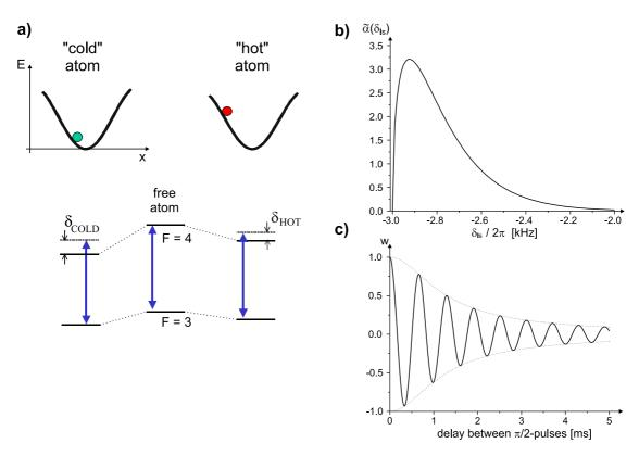
Figure 5.4: Differential light shift. (a) A cold atom experiences a stronger differential light shift than a hot one. (b) Distribution of the differential light shift,  $\tilde{\alpha}(\delta_{\rm ls})$ , for an ensemble of atoms at  $T = 100 \,\mu {\rm K}$  in a trap of  $U_0 = 1 \,\,{\rm mK}$ , according to Equation (5.11). (c) Calculated non-exponential dephasing of a Ramsey signal. The envelope is the fourier transform of  $\tilde{\alpha}(\delta_{\rm ls})$ .
