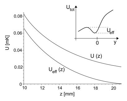
Figure 3.8: Reduction of the trap depth due to gravity. The inset shows the sum  $U_{\text{tot}}$  of the dipole potential and the gravitational potential versus the radial coordinate y for an arbitrary potential well along the optical z-axis. Below, the resulting effective potential depth  $U_{\text{eff}}(z)$  is compared to the pure dipole potential U(z) for z = 10 - 21 mm.
