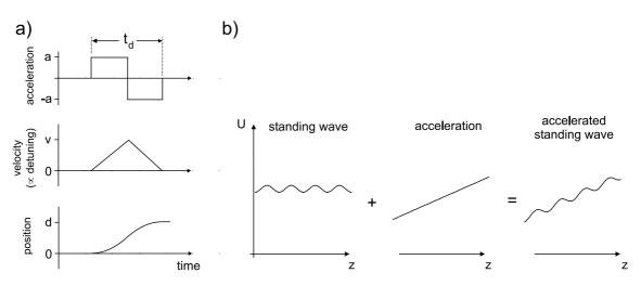
Figure 3.2: Accelerated standing wave. (a) The standing wave is uniformly accelerated and then decelerated within the transportation time  $t_{\rm d}$ . (b) In the moving reference frame, the accelerated standing wave is the sum of the standing wave potential at rest and a linear ramp.
