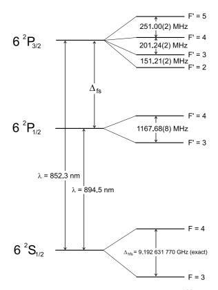
Figure 2.4: Level scheme of the D-line of <sup>133</sup>Cs.
