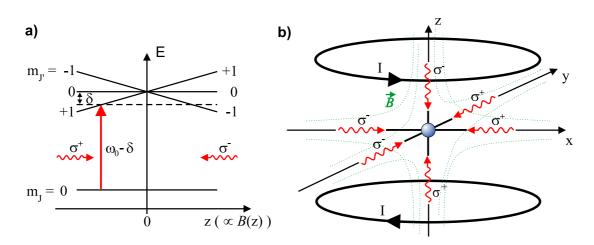
**Figure 2.1**: Magneto-optical trap (MOT). (a) Principle for the case of a  $J = 0 \rightarrow J' = 1$  transition in the one-dimensional picture. The degeneracy of the excited state is lifted due to the Zeeman effect in the linear magnetic field gradient. When the atom moves away from the trap center it becomes resonant with the laser which pushes it back to the center. (b) For three-dimensional confinement, two coils in anti-Helmholtz configuration produce a quadrupole field.
