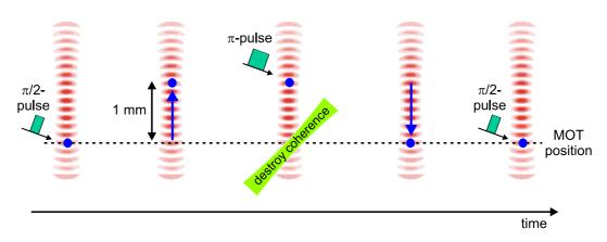
Figure 5.11: Quantum state transportation. An atom prepared in a superposition of hyperfine states is displaced by 1 mm. Synchronously to the  $\pi$ -pulse, we shine in an off-resonant state mixing laser into the initial position. After transporting the atom back to its initial position, the state superposition is analyzed by means of a second  $\pi/2$ -pulse.
