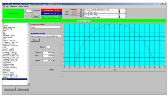
**Figure B.2**: Computer control system. (a) The "analog blocks" control the output of the 16 analog channels and are composed of "waveforms". (b) Waveforms contain arbitrary sequences of voltages which may be loaded from an external file.
