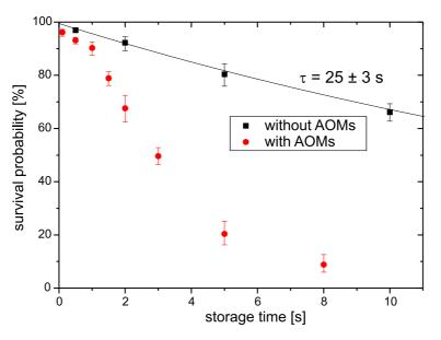
Figure 2.11: Storage time in the dipole trap with (circles) and without phase noise (squares) at otherwise identical conditions. In the latter case the decay is due to background gas collisions and purely exponential with a decay time of  $\tau = 25 \pm 3$  s.
