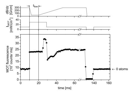
**Figure 2.8**: "Magnetic umbrella". During the loading time  $t_{\text{low}}$  the magnetic field gradient is reduced and the intensity of the MOT lasers is increased. The trapped atoms fully appear in the observation region at t = 50 ms, since the magnetic field needs 30 ms to increase to its full value. The graph shows the added fluorescence counts from 600 shots with a mean atom number  $\overline{N} = 2$ .
