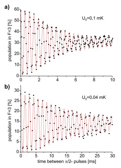
Figure 5.2: Ramsey fringes, recorded for two different trap depths. (a)  $U_0 = 0.1$  mK and (b) 0.04 mK. Their decay with time constants  $T_2^* = 4.4$  ms and 20.2 ms, respectively, is due to inhomogeneous dephasing caused by the energy distribution in the trap. Each datapoint results from 30 shots with about 50 initial atoms. The line is a fit according to Equation (5.20) (see page 80).
