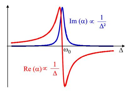
**Figure 2.2**: Real and imaginary part of the atomic polarizability  $\alpha$ . The dipole force is proportional to  $\text{Re}(\alpha)$ , which has a dispersive shape and thus changes sign when crossing the resonance. The scattering rate is proportional to  $\text{Im}(\alpha)$ , showing a Lorentzian lineshape.
