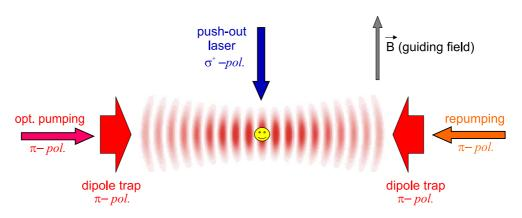
Figure 4.3: Polarization of laser beams.
