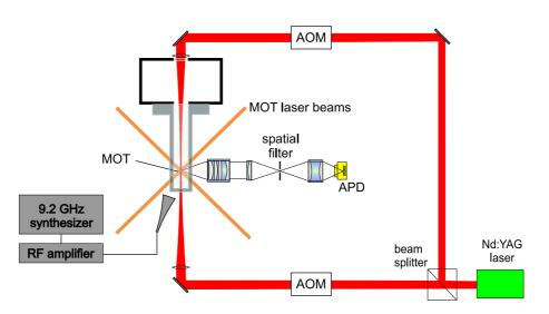
Figure 4.2: Setup for microwave spectroscopy. The atoms are exposed to microwave radiation generated by a synthesizer.
