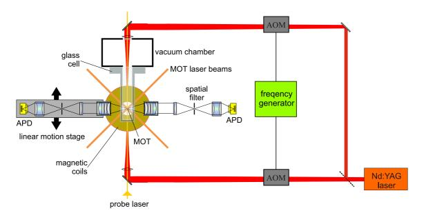
**Figure 3.3**: Experimental setup of the optical conveyor belt. AOMs are used to control the frequencies of the two laser beams that form the dipole trap. The fixed imaging optics on the right-hand side is used to monitor the fluorescence at the MOT position. The imaging optics mounted on the linear motion stage on the left-hand side is used for atom detection at any spot along the dipole trap.
