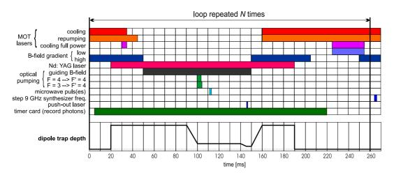
Figure 4.5: Typical timing sequence for microwave spectroscopy.
