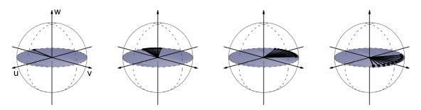
**Figure 5.3**: Inhomogeneous dephasing. The Bloch vectors precess with different angular frequencies.
