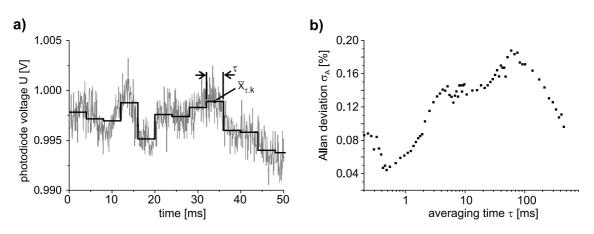
**Figure 5.9**: Measurement of the intensity fluctuations using the Allan deviation. (a) Output power of the Nd:YAG laser. (b) Corresponding Allan deviation, according to Equation (5.34).
