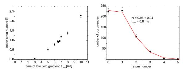
Figure 2.9: Statistics of the loaded atom number. (a) By increasing the time of low field gradient,  $t_{\text{low}}$ , we also increase the mean atom number  $\overline{N}$ . (b) Atom number statistics for  $t_{\text{low}} = 6.8 \text{ ms}$  (600 shots), resulting in a mean atom number  $\overline{N} = 0.96 \pm 0.04$  in this particular measurement. The line is the Poissonian distribution of Equation (2.45).
