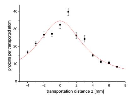
Figure 3.7: Number of fluorescence photons as a function of transportation distance z. The line is a fit with a Lorentzian according to Equation (3.11), yielding  $N_0 = 32.4 \pm 1.2$ ,  $N_{\text{offs}} = 2.2 \pm 0.8$ , and  $z_0 = 3.4 \pm 0.2$ .
