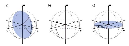
**Figure 4.1:** Bloch vector dynamics. (a) Resonant driving corresponds to a rotation around the *u*-axis. (b) A  $\pi/2$ -pulse transforms (0, 0, -1) into (0, -1, 0). (c) Free precession in the *uv*-plane.
