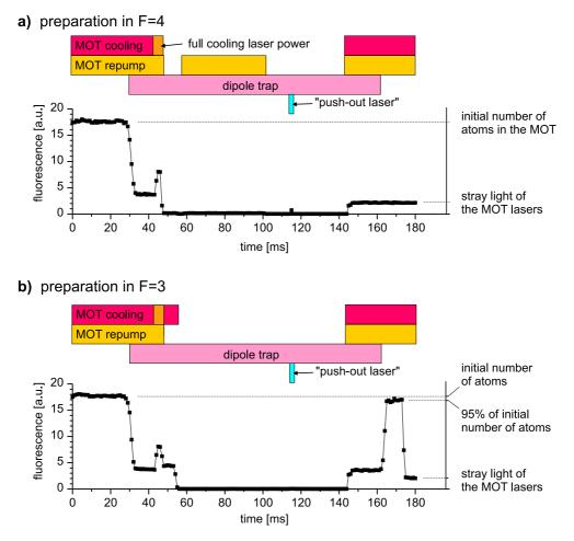
Figure 4.4: State selective detection. Shown are the integrated APD counts from the MOT region binned in time intervals of 1 ms and accumulated over 10 repetitions with 20 atoms each. The push-out laser removes all atoms in F = 4 from the trap (upper graph), whereas 95 % of the atoms in F = 3 remain trapped (lower graph).
