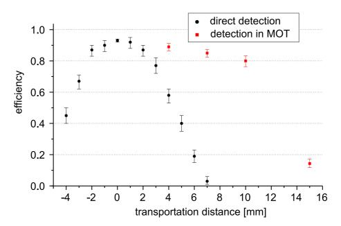
Figure 3.6: Transportation efficiency of the optical conveyor belt. Each data point results from about 100 shots performed with one atom each. Circles: The atom is detected by resonant illumination at its new position. Squares: More efficient detection by moving the atom back and recapturing it into the MOT.
