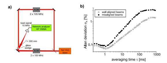
**Figure 5.10**: Measuring the pointing instability. (a) The dipole trap beams having a frequency difference of  $\Delta \nu = 10$  MHz are overlapped on a fast photodiode. (b) Allan deviation of the amplitude of the resulting beat signal.
