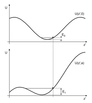
Figure 3.10: Heating due to abrupt acceleration, shown for a change of the acceleration from 0 to  $a = 0.5 a_0$ . An atom with energy  $E_0$  trapped in the potential at rest, U(z', 0), can obtain a higher energy  $E_1 > E_0$  in the accelerated potential U(z', a).
