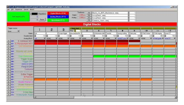
Figure B.1: Computer control system. The graphical user interface permits the rapid design of complex experimental operating sequences. The digital blocks define the sequence of the 32 TTL output channels.
