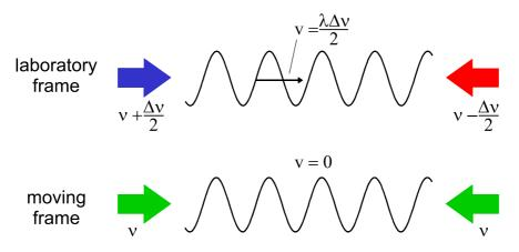
**Figure 3.1**: "Optical conveyor belt". Two counterpropagating laser beams of slightly different frequencies create a moving standing wave. In the moving reference frame both beams are doppler shifted by the same amount.
