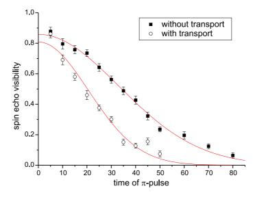
**Figure 5.13**: Visibility of the spin echo with and without transportation between the microwave pulses. The lines are fits according to Equation (5.44). The faster decay of the visibility is caused by heating of the atoms during the transportation procedure.
