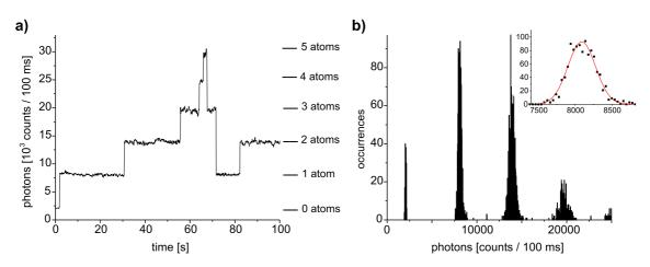
**Figure 2.7**: (a) Fluorescence signal of the MOT, integrated in time intervals of 100 ms. Each trapped atom increases the signal by the same amount, allowing us to determine their exact number. (b) Histogram of fluorescence counts.
