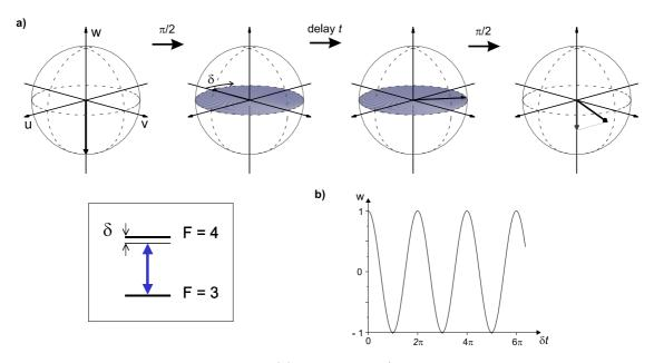
Figure 5.1: Ramsey spectroscopy. (a) Following a  $\pi/2$ -pulse, the Bloch vector precesses during a delay time t with angular frequency  $\delta$ , which is the detuning of the microwave radiation from the atomic resonance. After a second  $\pi/2$ -pulse we measure the w component of the Bloch vector. (b) Ramsey fringes. The measured w component oscillates with frequency  $\delta$  as a function of the delay time.
