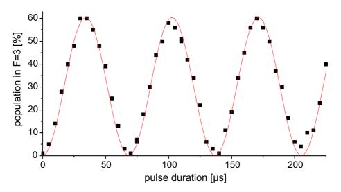
**Figure 4.10**: Rabi oscillations on the  $|F = 4, m_F = 0\rangle \rightarrow |F = 3, m_F = 0\rangle$  clock transition recorded in a trap of depth  $U_0 = 1.0$  mK. The line is a fit according to Equation (4.50).
