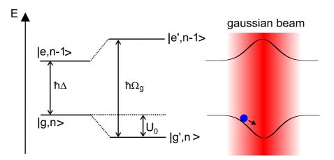
**Figure 2.3**: Schematic view of the light shift of a two-level atom in the dressed state picture. Right: The shift is proportional to the local laser intensity. For the case of red detuning the atom is pulled into the focus of the laser beam.
