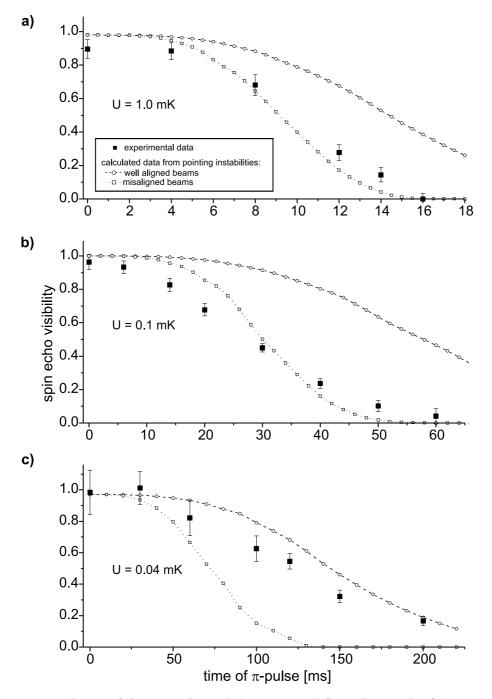
Figure 5.8: Decay of the spin echo visibility, extracted from the signals of Figure 5.7. Shown are the contributions of the dephasing due to the pointing instability of the trapping laser for the case of well aligned and of misaligned beams.
