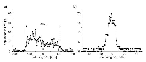
**Figure 4.8**: Magnetic field compensation using microwave spectroscopy. (a) Result of coarse compensation. The total width of the Zeeman spectrum is  $\omega_{\rm sp}/2\pi = 240$  kHz. (b) Result of fine compensation. The total width is minimized to  $\omega_{\rm sp}/2\pi = 20$  kHz by the fine compensation, corresponding to a field of  $B_{\rm res} = 0.4 \,\mu\text{T}$ .
