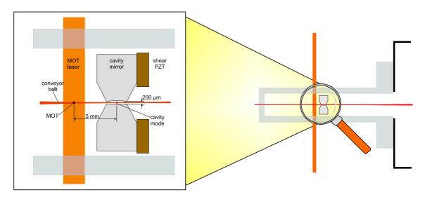
Figure 6.2: Scheme of the planned experiment. The optical conveyor belt will transport atoms from the MOT into the cavity mode.
