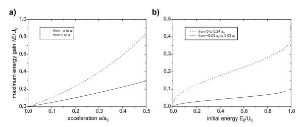
Figure 3.11: Energy gain due to abrupt acceleration. (a) Maximum energy gain  $\Delta E$  due to an abrupt change of the acceleration from 0 to a (straight line) and from -a to a (dotted line) assuming an initial energy  $E_0 = 0.2 U_0$ . (b) Maximum energy gain vs. initial energy  $E_0$  for a change from 0 to  $0.24 a_0$  (dotted line) and from  $-0.03 a_0$  to  $0.03 a_0$  (straight line). The value  $a = 0.03 a_0$  is used in Chapter 5 for the "quantum state transportation".
