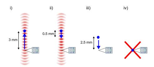
**Figure 3.12**: Ejection of a single atom into ballistic flight. (i) The atom is displaced from its initial position by 3 mm. (ii) Acceleration over a distance of 0.5 mm. (iii) Free flight over a distance of 2.5 mm. (iv) Recapture in the MOT.
