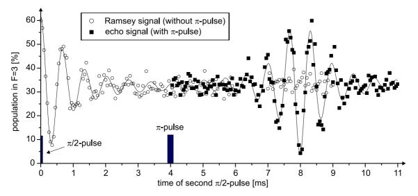
**Figure 5.6**: Experimental observation of a spin echo in a trap of  $U_0 = 1.0$  mK. The application of a  $\pi$ -pulse at t = 4 ms leads to a rephasing of the magnetic dipole moments around t = 8 ms (squares). The open circles show a Ramsey signal, obtained without a  $\pi$ -pulse, but with otherwise identical parameters. Each point results from 30 shots with about 50 atoms each. The lines are fits according to Equations (5.20) and (5.25).
