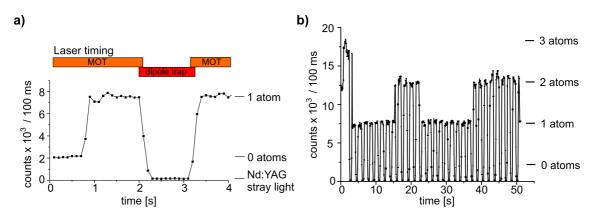
Figure 2.10: Transfer of atoms between MOT and dipole trap. (a) Storage of a single atom in the dipole trap for 1 s. The fluorescence signal (integration time = 100 ms) of the atom demonstrates the trapping in the dipole trap and recapturing by the MOT. (b) Atoms can be transferred many times between both traps without losses. The storage time is 500 ms in this case.
