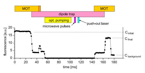
Figure 4.6: Atom counting. Initial and final number of atoms is inferred from their fluorescence in the MOT.
