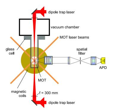
**Figure 2.5**: Experimental setup. MOT and dipole trap are overlapped in the center of a vacuum cell. Fluorescence light is collected by imaging optics with spatial filtering apertures and is detected with an avalanche photodiode (APD).
