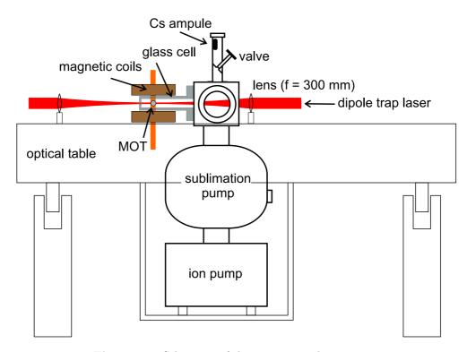
Figure 2.6: Schematic of the experimental apparatus.
