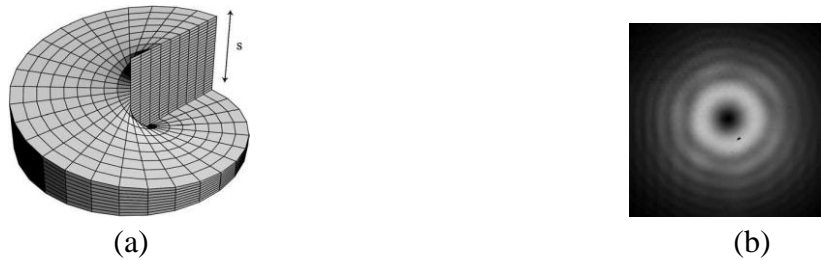
Figure 1.2: (a) The structure of a spiral phase plate. The thickness of the plate increases proportional to the azimuthal angle. (b) Beam pattern of a donut beam.
