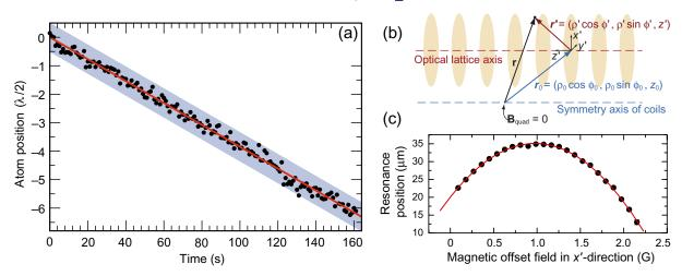
**Figure 6.** (a) Drift of the optical lattice with respect to the imaging system over long times. (b) New coordinate system for an offset between the symmetry axes of optical lattice and the center of the quadrupole magnetic field. (c) Measured quadratic dependence of the position of the microwave resonance frequency with increased offset  $\mathbf{r}_0$  along the *x*'-direction. The offset is changed by applying a homogeneous offset field along the *x*'-direction.
