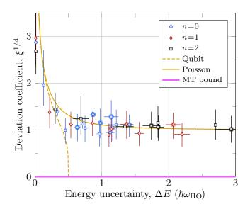
Figure 4. Deviations from the MT speed limit. The measured coefficient  $\xi$  is plotted vs  $\Delta E$  for a wide spectrum of experimental conditions, varying the initial displacement  $\Delta x$  and the wave packet shape  $n = \{0, 1, 2\}$ . The pink line indicates the MT bound. Points corresponding to  $\Delta x > 0.25 \lambda/2$  (nonharmonic regime) are highlighted by a surrounding circle. Note that for better visualization purpose the fourth root of  $\xi$  is plotted.
