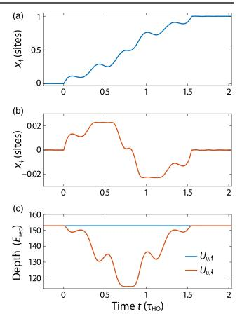
FIG. 4. Cross talk between spin-dependent potentials. Example of transport ramp as in Fig. 1(d) when varying  $x_R(t)$  without compensating  $x_L(t)$ ; i.e.,  $x_L(t) = x_L(0)$ . (a) The position of the spin-up potential only depends on the *R*-polarized standing wave,  $x_{\uparrow}(t) = x_R(t)$ . The position (b) and depth (c) of the spin-down potential are modulated because of the cross-talk contribution from the moving *R*-polarized standing wave; see Eq. (B5).
