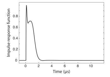
FIG. 6. Reconstructed impulse response function. The control bandwidth is mainly limited [48] by a time delay, which originates from the acousto-optical modulators employed in the optical phase-locked loop to control the phases  $\phi_{R,L}(t)$ ; see Appendix A.
