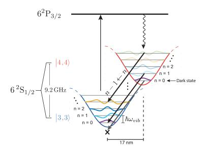
Figure 2.6: **Motional ground state cooling**. The microwave driving induces a transition from the motional level n of  $|4, 4\rangle$  to the motional level (n - 1) of  $|3, 3\rangle$ , therefore reducing the energy of the atom. The remumping beam  $(F = 3 \rightarrow F' = 4)$  transfers the atom to  $6^2 P_{3/2}$  from where it decays back to close the cycle. Once the atom reaches the ground state of  $|4, 4\rangle$  there are no resonant transitions available, making it a dark state.
