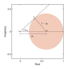
Figure C.1: **Phase bound of single-pixel images**. The phase of a complex number inside the orange circle is bounded by the expression given in Eq.(C.1).
