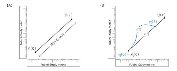
Figure 4.2: Fubini-Study metric. (A) The Fubini-Study metric provides a measure of the distance between two quantum states. (B) The quantum state  $\psi_1$  evolves along the black curve while  $\psi_2$  evolves along the blue curve. The path length is  $\ell(t)$  in both cases but the distance between initial and final states is shorter for  $\psi_2$ .
