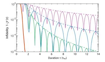
FIG. 8. Transport protocols compared. Infidelity computed numerically for the same conditions of Fig. 2 and  $T_{\perp} = 0$  using different transport protocols. From top to bottom: a linear transport ramp (purple), parabolic control (blue), adiabatic control (green), optimal quantum control (thick red). The dashed lines represent the envelope functions according to Eqs. (I1a), (I1b), and (J2).
