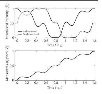
FIG. 5. Optical interferometric measurement of the trap trajectory. (a) Phase quadrature measurement of  $\phi_R(t)$ , showing the normalized intensities recorded after a Glan-Laser polarizer for the in-phase,  $\{1 + \cos[\phi_R(t)]\}/2$ , and the quadrature signal,  $\{1 + \sin[\phi_R(t)]\}/2$ . (b) Displacement  $x_{\uparrow}(t) = (\lambda/2)\phi_R(t)/(2\pi)$ of the optical conveyor belt, reconstructed from the in-phase and quadrature signals.
