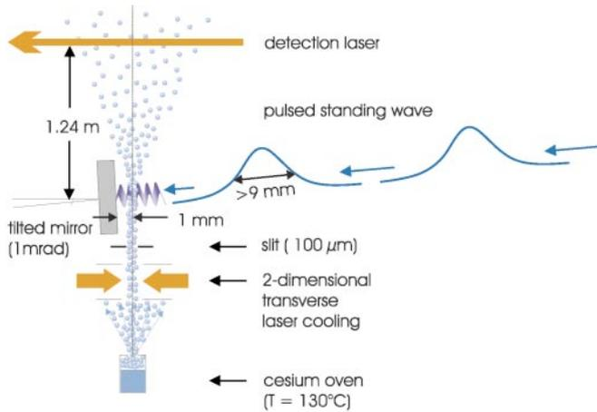
**Fig. 5.** Schematic experimental setup to measure the beam profile behind the standing wave. The pulse length is varied between 30 and 80 ps and the standing wave extends over 5–12 mm from the mirror. The atomic beam (about 1 mm distance from the mirror) thus is fully covered by the standing wave. The power of the standing wave is varied from 0 to 464 mW, the detuning of the laser from the Cs-D<sub>2</sub> line at 852 nm is set between 5 and 200 GHz
