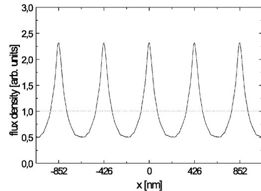
**Fig. 10.** Simulated flux density distribution of the atomic beam in the focal plane shown over 5 periods of the pulsed standing wave. Parameters:  $P = 100$  mW,  $\Delta = 2\pi \times 30$  GHz,  $\tau_p = 60$  ps. The *dotted line* indicates the flux density without standing wave
