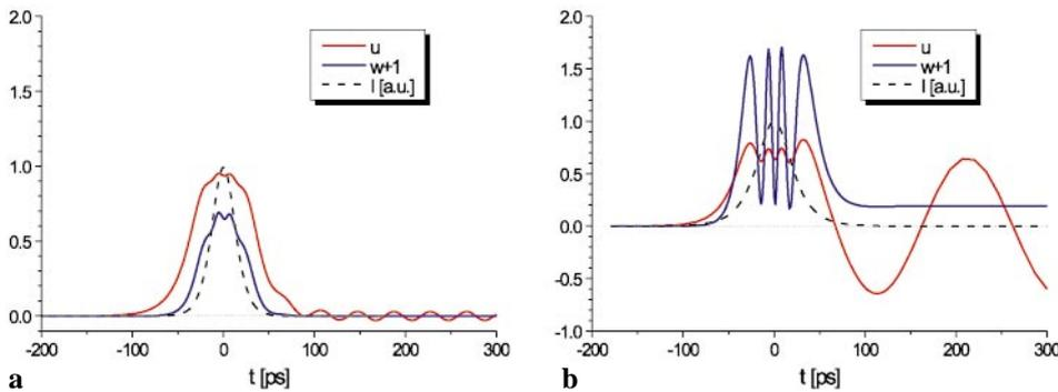
**Fig. 2a,b.** Numerically simulated evolution of the Bloch vector ( $u$  and  $w$  components). **a** Adiabatic conditions ( $\tau_p = 30$  ps,  $\Delta = 2\pi \times 25$  GHz,  $\tau_p \Delta = 4.7$ ) **b** Non-adiabatic conditions ( $\tau_p = 30$  ps,  $\Delta = 2\pi \times 5$  GHz,  $\tau_p \Delta = 0.94$ ). The dashed curve shows the laser intensity  $I$
