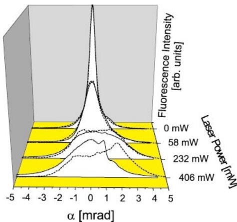
**Fig. 9.** Comparison of the measured beam profiles (*solid lines*) with simulated profiles (*dashed lines*) 1.24 m behind the interaction zone at  $\tau_p = 50$  ps ( $\Delta = 2\pi \times 30$  GHz). For large laser power (406 mW) a strong deviation of experiment and simplified theory is observed.
