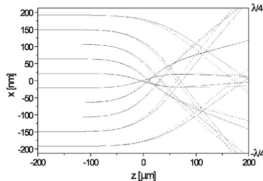
**Fig. 4.** Simulation of atomic trajectories in one period of the standing wave. *Solid line*: numerical integration of the Bloch equation. *Dashed line*: calculated with the approximated force of (13). Parameters:  $v = 300$  m/s,  $\tau_p = 80$  ps,  $\Delta = 2\pi \times 5$  GHz,  $\tau_p \Delta = 2.5$ ,  $P = 100$  mW
