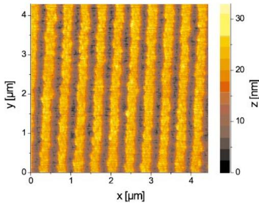
**Fig. 12.** Atomic force microscope picture of an exposed and developed substrate. The regular lines with a periodicity of  $\lambda/2 = 426$  nm result from the spatial flux density distribution of the cesium atomic beam caused by the pulsed standing wave. Parameters:  $P = 350$  mW,  $\Delta = 2\pi \times 20$  GHz,  $\tau_p = 80$  ps
