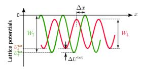
**Figure 3.** State-dependent optical lattices relatively shifted by a distance  $\Delta x$ . The total trap depth difference  $\Delta U^{\rm tot} = U_{\uparrow}^{\rm tot} - U_{\downarrow}^{\rm tot}$ , and lattice contrast  $W_s$  for spin state  $|s\rangle$  are shown. Unlike the spin  $|\uparrow\rangle$  lattice, the contrast and total depth of the spin  $|\downarrow\rangle$  lattice vary with the shift distance.
