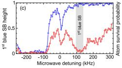
Figure 9. Microwave spectroscopy performed (a) before cooling and (b) after 20 ms of microwave cooling, with optimal experimental parameters (see table 2). (c) Blue sideband height versus detuning of the microwave cooling frequency ( $\circ$ ) and atom survival probability measured after the cooling ( $\square$ ), (data points in (a) and (b) are from [11]).
