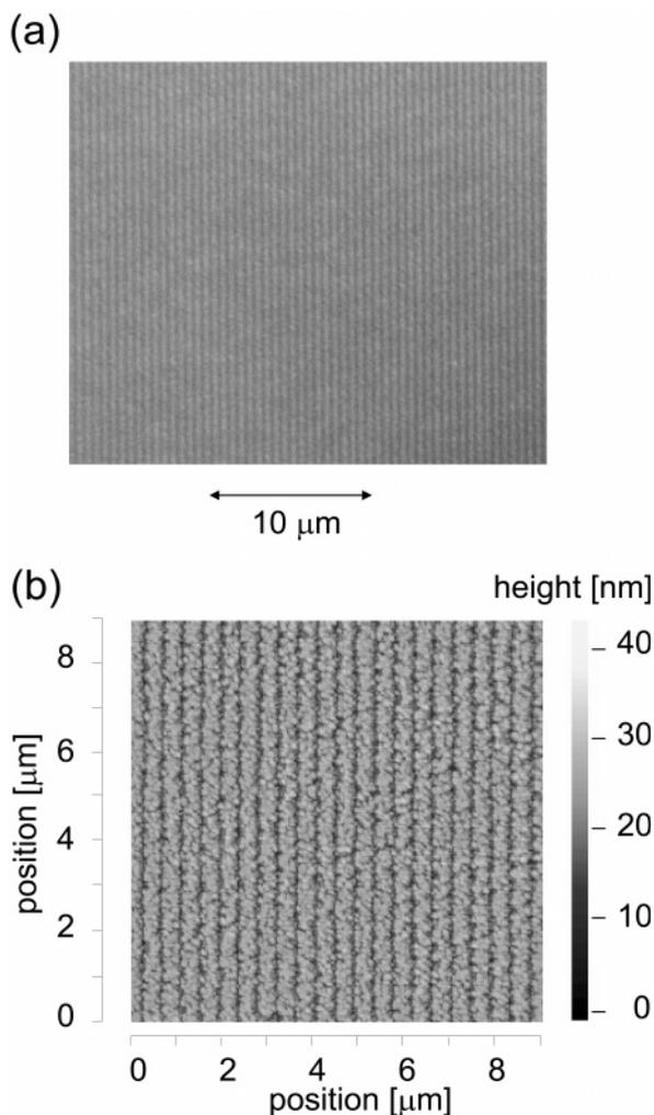
**Fig. 4a,b.** Microscopic images of the written structures. In both images, bright structures represent areas of gold, silicon is dark. **a** Light microscope image using difference interference contrast. These lines can be found in the whole region exposed to the atomic beam with a diameter of 1 mm. **b** Atomic force microscope image of a region ( $9\ \mu\text{m} \times 9\ \mu\text{m}$ ) scanned in contact mode
