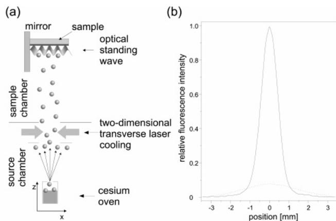
**Fig. 2.** **a** Sketch of the experimental setup housed in a high-vacuum apparatus showing cesium beam source, two-dimensional optical collimation stage (source chamber), standing-wave light field, and sample (sample chamber). **b** Beam profiles of the atomic beam with (solid line) and without (dotted line) two-dimensional optical transverse collimation. The beam profiles were taken with a CCD camera 1 m beyond the collimation stage where the atoms traverse a resonant laser beam
