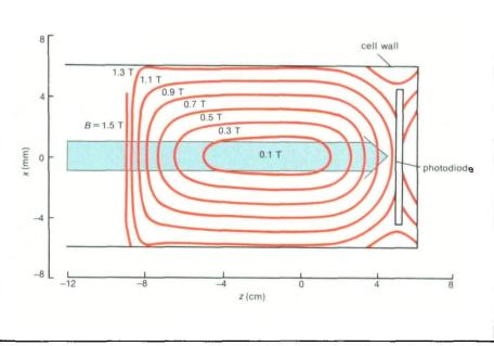
1 Schematic of a magnetic trap for hydrogen showing contours of equal magnetic potential (red). Spin-polarised hydrogen atoms are confined to the centre of the trap where the magnetic field is a minimum. The cooling laser is shown in blue
