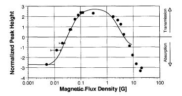
**Fig. 11.** Comparison of calculated (solid line) and measured height (dots) of the  $(F=3 \rightarrow F'=2, 3)$  crossover resonance peak for various magnetic flux densities. The error bars reflect the uncertainty in the measurement of the experimental flux density. Above 10 G, our approximation breaks down, as explained in text
