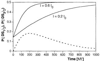
Fig. 12. Time evolution of the occupation probability of both dark states for the  $(3 \rightarrow 2)$  transition in the  $\Sigma$  system, calculated for two different laser intensities. The dashed line shows the difference of the two solid lines. Discussion in text
