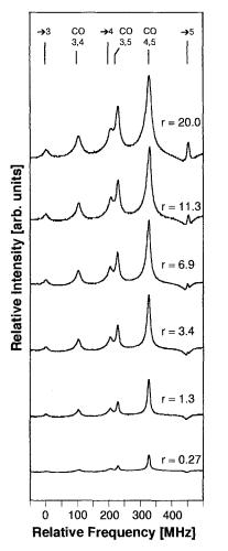
Fig. 6. Series of saturated absorption spectra starting from the (F=4) ground state taken with constant probe-beam intensity and successively weaker pump-beam intensity  $(r=I_{Pump}/I_{Probe})$ . The probe-beam intensity was of order  $I_0$ . All spectra are to the same scale. The  $F=4 \rightarrow F'=5$  transition shows a reversal of sign with decreasing pump intensity. The spectra of Figs. 2 and 10 were taken with r=3 and  $I_{Probe}=0.4 \,\mu\text{W/mm}^2$
