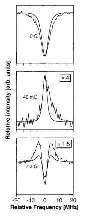
Fig. 13. Comparison of calculated (smooth curves) and experimental line shapes for the  $(F=3\rightarrow F'=2, 3)$  crossover resonance in magnetic flux densities of 0 G, 40 mG, and 7.3 G. The lower two figures were scaled by a factor of 4 and 1.5, respectively
