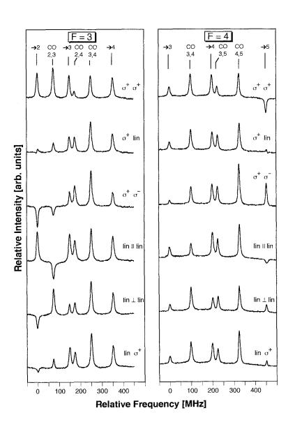
this change in atomic population. Since both beams are derived from the same laser and thus have the same frequency, the Doppler effect brings different velocity groups into resonance with each beam. Consequently, the probe beam sees the hole burnt into the population difference by the pump beam only for those atoms that fly perpendicularly to the laser beam ("v = 0"-resonance). All other velocity groups contribute a Doppler background which is electronically subtracted using the reference beam.
