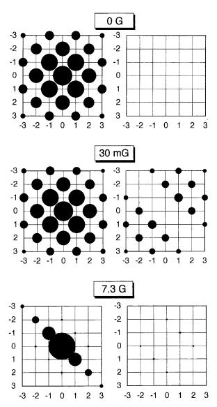
**Fig. 14.** Calculated density matrices of the (F=3) ground state for various magnetic flux densities and  $t \rightarrow \infty$ . The area of each circle is proportional to the absolute value of the corresponding density matrix element connecting two of the magnetic sublevels. The matrices on the left show the real parts, those on the right the imaginary parts
