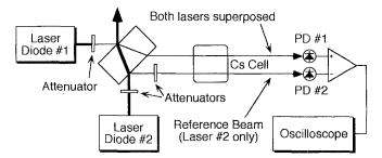
Fig. 7. Experimental setup for the observation of hyperfine repopulation pumping (PD: photodiode)
