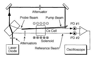
Fig. 1. Experimental setup for saturated absorption spectroscopy in magnetic fields (PD: photodiode)
