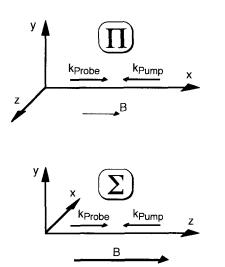
Fig. 5. Two coordinate systems used to explain the experimental spectra. The  $\Sigma$  system is most appropriate for the situation of relatively strong magnetic fields, whereas the *II* system is very convenient for linear laser polarization in the low-field case
