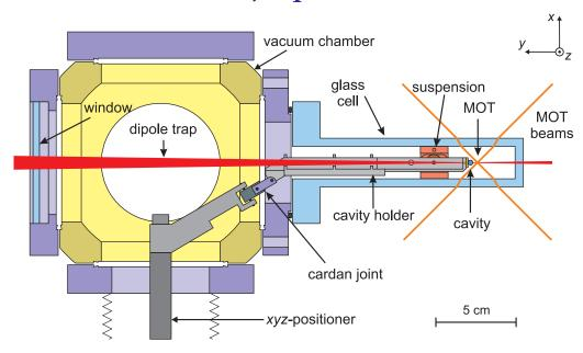
**Figure 4.** Cavity holder in the vacuum setup (top view). The adjustable holder is used for aligning the cavity position in the glass cell relative to the MOT. The resonator is placed about 4.6 mm away from the position of the MOT.
