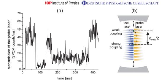
**Figure 7.** (a) Transmission signal of the probe laser beam through the cavity for the case of time-dependent coupling. (b) Due to jumps between different nodes of the repulsive lock laser standing wave, the coupling strength of the atom to the cavity changes.
