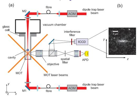
**Figure 2.** (a) Schematic view of the atom-trapping setup. Atoms are loaded from the MOT into the dipole trap and transported along the dipole trap axis into the cavity mode (oriented along the z-axis). The APD allows us to count trapped atoms and the ICCD camera provides information on their positions. (b) Fluorescence image of a single atom, illuminated for 1 s in the dipole trap.
