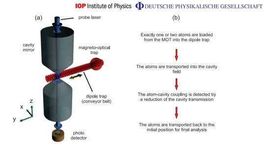
**Figure 1.** Concept of the experiment: (a) schematic drawing of the experiment and (b) outline of the basic experimental procedure.
