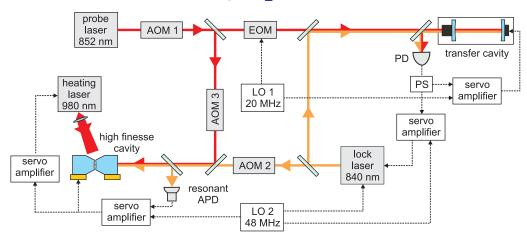
**Figure 5.** Frequency stabilization of the high-finesse cavity. Using the transfer cavity and the lock laser, the stability of the probe laser, which is stabilized to a caesium polarization spectroscopy, is transferred to the high-finesse cavity. AOM, acousto-optic modulator; EOM, electro-optic modulator; PD, photodiode; APD, avalanche photodiode; LO, local oscillator; PS, RF power splitter. The three servo loops are based on the PDH method.
