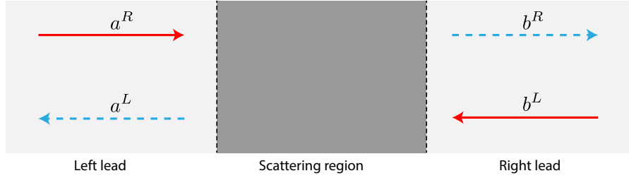
Figure 5.1: Schematic illustration of a general scattering setting. The system is a phase-coherent disorder sample (scattering region, dark grey), the transport properties of which are to be probed. This is connected to two ideal leads (light grey) on its left and right sides. The modes of each lead are labeled by a and b , and their corresponding directions by R and L . The color coding shows the incoming (red, solid arrows) and outgoing (blue, dashed arrows) modes.
