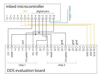
Figure A.1.: Schematics of the DDS-mbed pin connection. Detailed information about individual pins can be found in [48]. The connection to the ground is abbreviated by "gnd".
