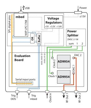
Figure 3.4.: Schematics of the home-built DDS box. The core of this box is the AD9954 evaluation board and an mbed microcontroller, allowing to control the desired RF-output by means of a USB-connection. Different colors indicate different signals and their functions.
