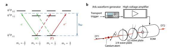
Figure 3.3.: (a) Level scheme showing the fine substructure of the caesium ground state and the first two excited states. (b) experimental implementation of the EOM. Adapted from [1].
