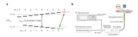
Figure 3.2.: (a) Level scheme showing the split hyperfine substructure of the two caesium ground states. (b) Experimental realisation of a microwave application to perform qubit operations. Adapted from [1].
