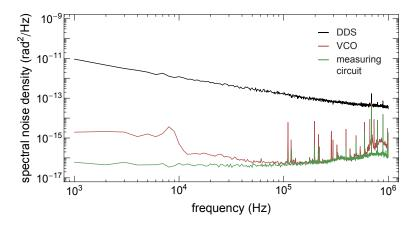
Figure 3.6.: Measured spectral noise density as a function of frequency. The  $S_{\phi}(\nu)$  of mixed DDS-box output signals (black) is compared to the previously employed single VCO source (red). The green curve represents measured noise without any input signal. The DDS phase noise follows a 1/f- relation.
