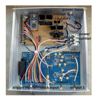
Figure A.2.: Picture showing the interior of the home-built DDS box.
