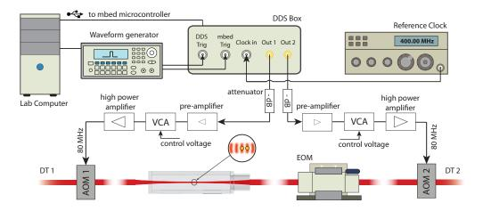
Figure 3.5.: Schematics of the AOM-circuit with the implemented DDS-box.
