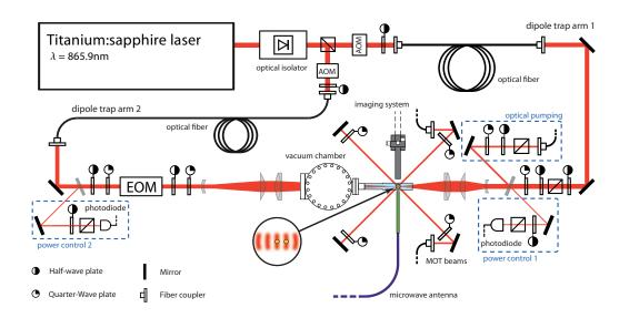
Figure 3.1.: Experimental setup. Adapted from [1].
