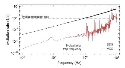
Figure 3.7.: Expected axial excitation rate due to measured residual phase noise of the two DDS output channels (black). For a typical trap frequency of 80kHz the rate is about  $0.1s^{-1}$ . The excitation rate caused by the previously installed VCO circuit is at this frequency about 5 orders of magnitude lower (red).
