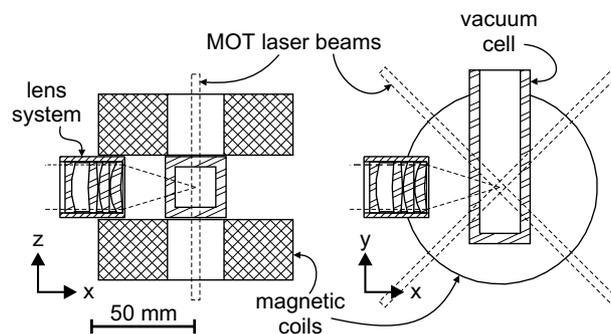
Fig. 1. Experimental geometry
