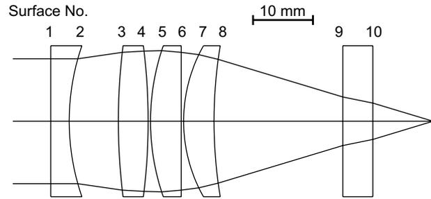
**Fig. 2.** Layout of the lens system. Surfaces 1 to 8 represent the objective itself, surfaces 9 to 10 represent the silica wall of the vacuum cell. The MOT is at the position of the focus on the right.
