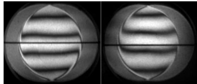
**Fig. 3.** Shear plate interferograms of the beam produced by collimating a point source with the objective lens. The shear is applied in two orthogonal directions, straight equidistant interference fringes correspond to a plane wavefront.
