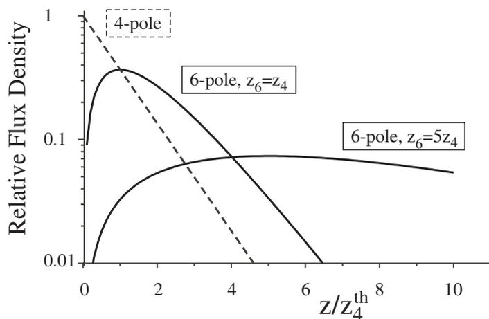
**Figure 7.** Comparison of axial flux density enhancement of a paramagnetic atomic beam by a magnetic 4-pole and a 6-pole with identical and with five times larger characteristic focal length.
