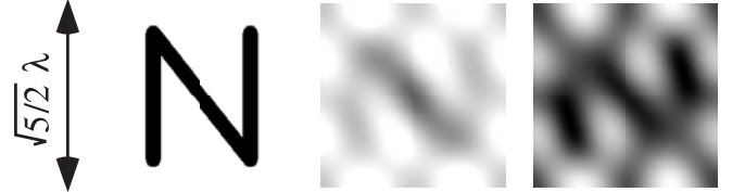
FIGURE 9 Example for N = 8 , letter 'N'. Left, original pattern I ; Middle, I_{\text{opt}} ; Right, reconstructed \tilde{I} by applying the coordinate descent method
