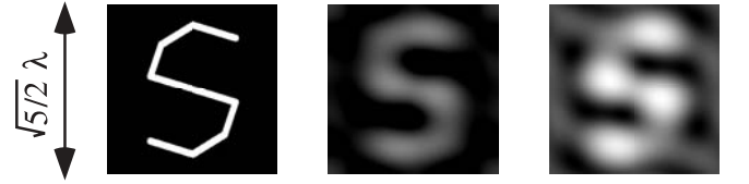
FIGURE 10 Example for N = 8 , letter 'S'. Left, original pattern I ; Middle, I_{\text{opt}} ; Right, reconstructed \tilde{I} by applying the coordinate descent method
