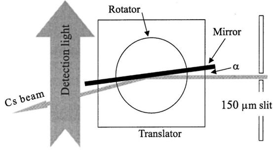
FIG. 4. Experimental arrangement for investigating reflection of atoms.
