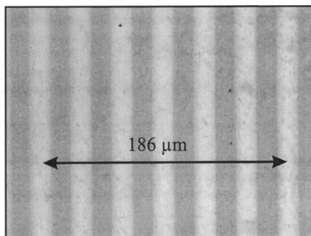
FIG. 2. Photograph of the magnetized videotape taken through a thin film of garnet with a polarization-sensitive microscope. The magnetic sine wave is clearly visible.
