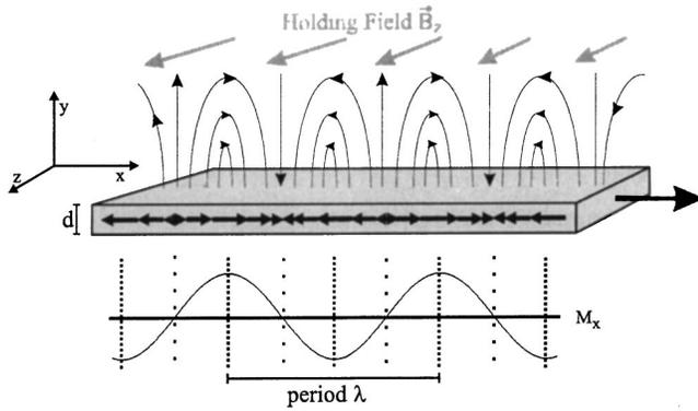
FIG. 1. Schematic of periodically magnetized videotape. The magnetization lies in the  $xz$  plane.
