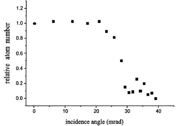
FIG. 5. Relative flux of atoms that have been reflected from the tape as a function of the angle of incidence at a longitudinal velocity of 75 m/s. The reflectivity starts to decrease for angles larger than  $\sim 20$  mrad. This provides information on the magnetic field at the surface.
