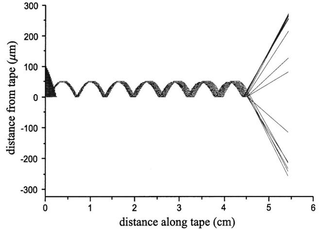
FIG. 7. Trajectories of the atoms along the reflector.
