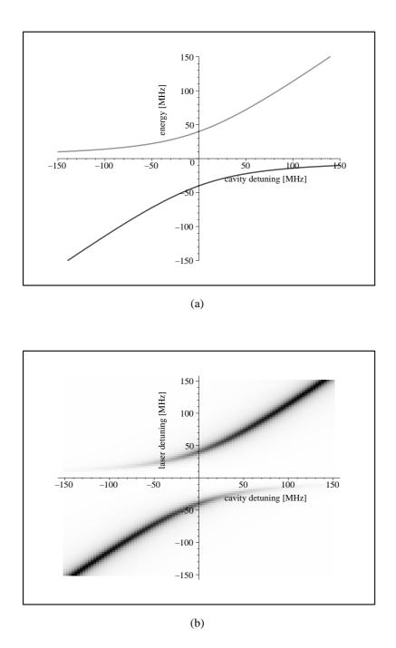
Figure 1.7: (a) Energy levels of the Jaynes-Cummings model vs. cavity detuning. (b) Cavity photon number of density matrix solution vs. cavity- and probe laser detuning. The white area corresponds to 0 photons, black area to 0.02 photons in the cavity for  $\varepsilon = 1$ . The atomic resonance is centered at the origin. The parameters are  $(g, \kappa, \Gamma) = 2\pi \cdot (40, 14, 5.2)$  MHz.
