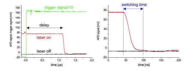
Figure 4.4: Laser switch-off behavior. Overview of the process on the left, zoom in on the right.
