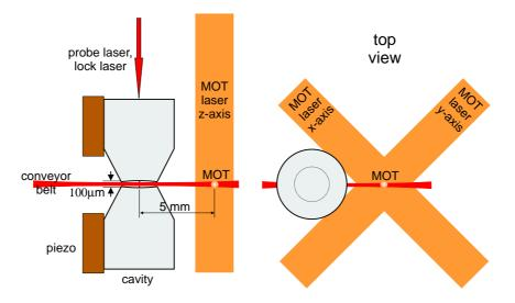
Figure 2.11: Planned setup geometry. The atoms will be transported over the distance of 5 mm from the MOT into the cavity mode through the slit between the mirrors. The conical mirror shape leaves more space for the x-y MOT laser.
