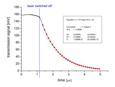
Figure 4.5: Decay of the transmission. The big points show the exponential fit.
