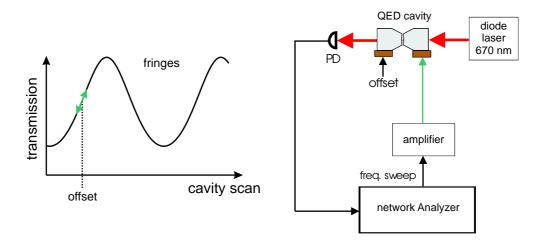
Figure 3.5: Setup for measuring the piezo resonance. The interference fringes of the cavity transmission provide a measure for the response of the piezo to a given signal.
