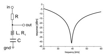
Figure 3.7: Schematic of a notch filter and calculated frequency response for the parameter set  $R = 470 \Omega$ , L = 1 mH, C = 16.3 nF,  $R_{\text{L}} = 4 \Omega$ .
