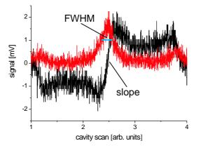
Figure 3.9: Transmission and error signal of the QED cavity at 200 nW lock laser power.
