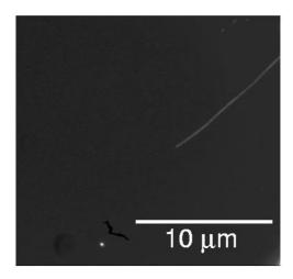
Figure 2.2: Microscope picture of the mirror surface, 500x magnification, dark-field observation. One sees a thin scratch, one clearly visible spot on the lower left and 3 smaller spots on the upper right. The dark objects in the lower part are defects of the camera.
