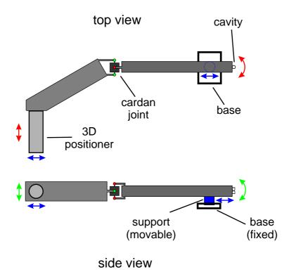
Figure 2.13: Kinematics of the cavity holder.
