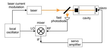
Figure 3.2: Basic PDH setup for stabilization of a cavity to a laser.
