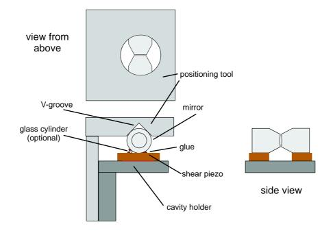
Figure 2.3: Assembly of the cavity.
