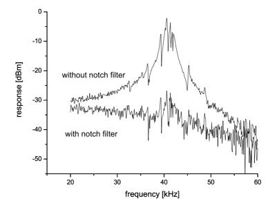
Figure 3.6: Resonance of the piezo element. The upper curve shows the response of the piezo. The lower curve shows the response compensated with a notch filter.
