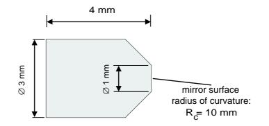
Figure 2.1: High reflectivity mirror, manufactured by the REO company.
