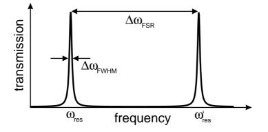
Figure 1.2: Transmission of an optical resonator.
