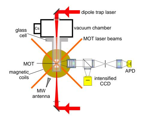
Figure 2.9: Experimental setup of our main experiment for the manipulation of single Cs atoms.
