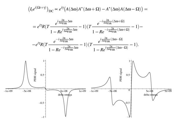
Figure 3.3: Real part of PDH signal for  $\gamma = 0.99 \cdot \pi$  (left) and  $\gamma = \frac{1}{2}\pi$  (right) vs. the relative detuning  $\Delta \omega$ .
