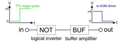
Figure 4.3: Inverter for laser switching.
