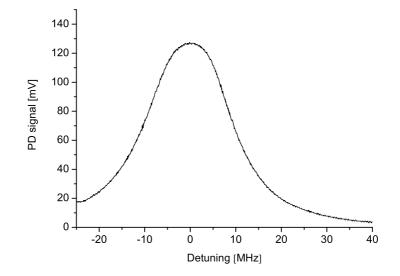
Figure 3.11: Scan of the locked cavity over the probe laser resonance. The scan rate is 100 Hz, the average of 64 tracks was taken.
