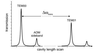
Figure 2.7: Measurement of the transversal mode distance (schematic). One sees the transmission of two neighboring transversal modes and the AOM sidebands.
