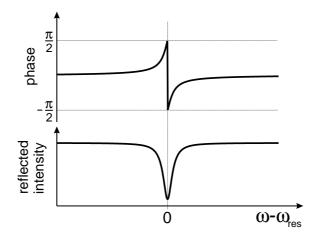
Figure 3.1: Intensity and phase of a laser field reflected from the cavity.
