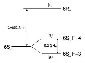
Figure 2.10: Cs atom as a three-level system. Shown are two long-lived hyperfine states and the excited state of the  $D_2$  line. Hyperfine splitting of the  $P_{1/2}$  state is omitted.
