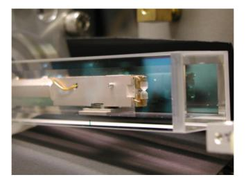
Figure 2.4: Assembled cavity in the glass cell of the test vacuum setup.
