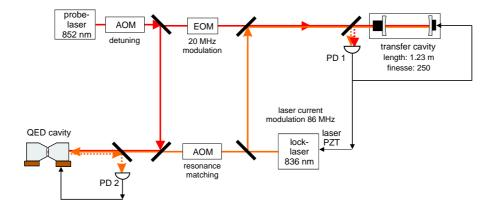
Figure 3.4: Stabilization scheme of the QED cavity using an off-resonant lock laser. PDH electronics are omitted.
