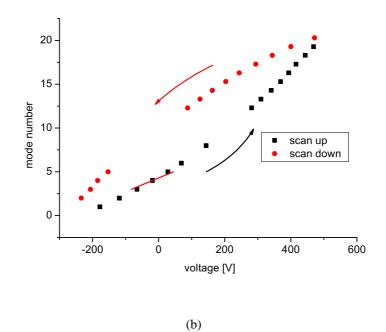
Figure 2.6: Measurement of the voltage-travel relation of the piezo elements. Figure (a) shows the transmission of transversal modes vs. mirror scan, figure (b) shows the response curve. The y-axis in (b) is proportional to the resonator length changes. For a small scan range between two neighboring modes one obtains a different response, which is also shown.
