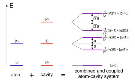
Figure 1.4: Eigenstates of the resonant atom-cavity system.
