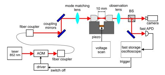
Figure 4.1: Cavity ring-down setup.
