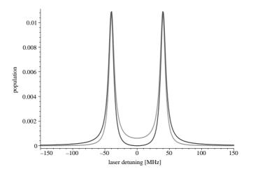
Figure 1.6: Rabi splitting in density matrix solution. Shown is the case of cavity resonant with the atom (centered at the origin). The parameters are  $(g, \kappa, \Gamma) = 2\pi \cdot (40, 14, 5.2)$  MHz. The dark curve is the cavity population vs. laser detuning, the grey curve shows the atomic excitation.
