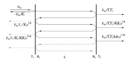
Figure 1.1: Fabry-Perot resonator. An incident electromagnetic wave leads to a series of partial reflections.
