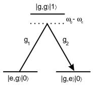
Figure 1.8: Cavity which is detuned far from the atomic resonance couples two atoms via a virtual cavity excitation.
