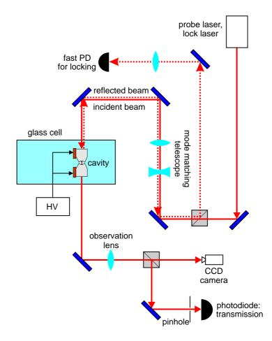
Figure 2.5: Optical setup for characterization and stabilization of the cavity.
