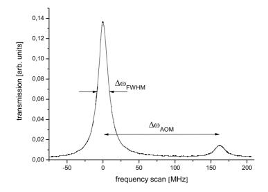
Figure 2.8: Cavity transmission showing the  $TEM_{00}$  line and its AOM sideband, averaged over 64 measurements.
