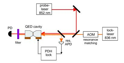
Figure 3.10: Scheme of cavity detuning. The locked cavity follows the detuning of the lock laser.
