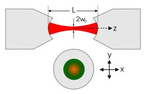
Figure 1.3: Fundamental TEM<sub>00</sub> mode.
