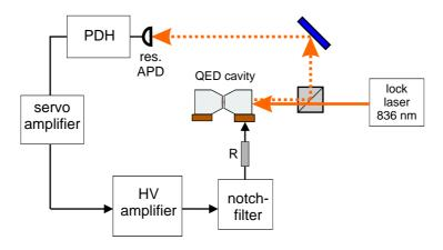
Figure 3.8: QED cavity lock with resonance compensation.
