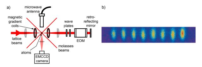
Figure 1. (a) Schematic experimental setup. (b) String of eight atoms with a distance of 17 lattice sites ( $\approx 7 \,\mu$ m). The pattern has been prepared by magnetic resonance methods [2]. From the fluorescence images, the position of the atoms can be deduced with single site resolution [1], verifying the targeted inter-atomic distance. The picture is the sum of approximately 50 single fluorescence images.
