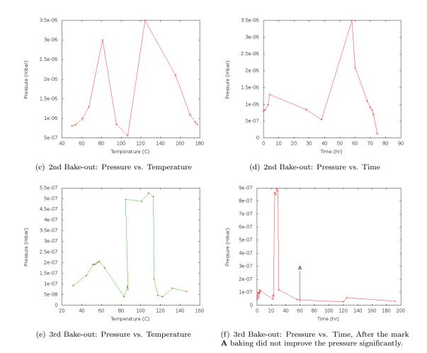
FIGURE 3.12: Pressure evolution during bake-out cycle, Two pressure peaks are visible in both measurements
