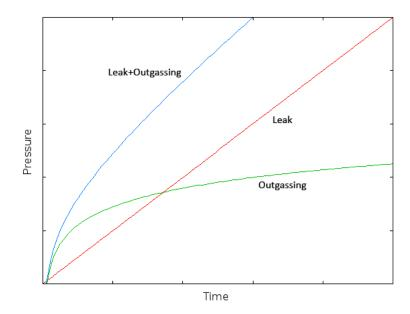
(a) A Typical rate-of-rise curve, comparison between leak and outgassing is shown
