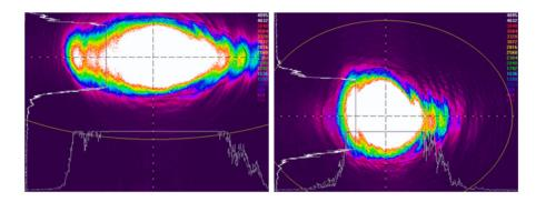
FIGURE 3.4: Beam profile before (left) and after (right) circularization, The picture is saturated but it shows the compressed beam spot. The final beam diameter about 3 mm.
