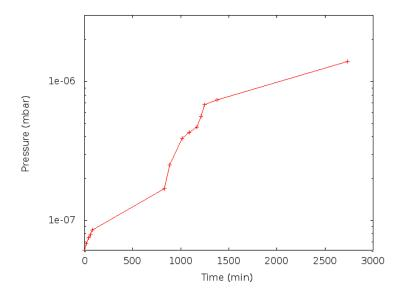
(b) Rate-of-rise curve, Pressure readings taken before bake-out. Comparing to the typical rate-of-rise curve it is clear that leakage and outgassing are both present.
