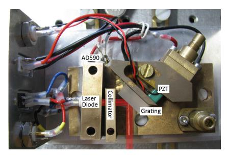
FIGURE 3.1: Laser diode in ECDL setup with Littrow configuration, Optical feedback is shown with the thinner red line.
