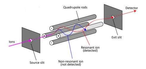
FIGURE 3.14: Quadrupole mass spectrometer principle, The ions can travel through the rods and reach the detectors only for some certain values of the applied potential on the rods [15].
