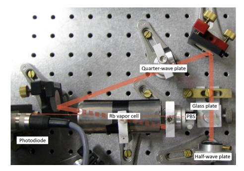
FIGURE 3.6: Polarization spectroscopy setup, the PBS before Rb vapor cell is to ensure linear polarization of the probe beam after reflection from the glass plate.
