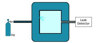
(a) Total leak test, can be used to approximately locate the leak. Dark colored box is the covering (plastic bag).
