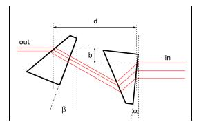
FIGURE 3.3: Alignment of anamorphic prism pair, Stencil for anamorphic prism pair (Thorlabs PS871-B) with  $0.5 \times$  magnification, two vertical lines are for guiding the laser beam (shown in red lines) in the correct angle.  $\alpha = 6^{\circ}$ ,  $\beta = 21.1^{\circ}$ , b = 20 mm, d = 5.1 mm
