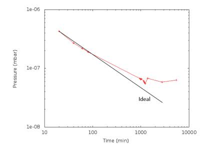
FIGURE 3.11: Pump-down curve, The curved pump-down characterizes a leaky or with outgassing system.
