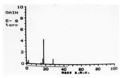
FIGURE 3.16: Mass spectrum of the vacuum system before bake-out, Water peaks at 17 a.m.u for hydroxyl and 18 for water vapor are significant.
