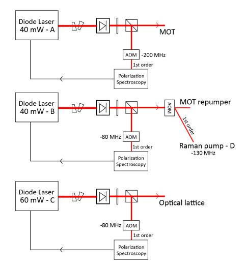
FIGURE 3.8: Complete laser system, Lasers are frequency locked to these transitions: **A**  $F = 2 \longrightarrow F' = 3$ , **B**  $F = 1 \longrightarrow F' = 2$ , **C**  $F = 1 \longrightarrow F' = 0$ , **D**  $F = 2 \longrightarrow F' = 2$
