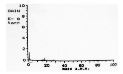
FIGURE 3.17: Mass spectrum of the vacuum system after bake-out, Water peaks are vanished.
