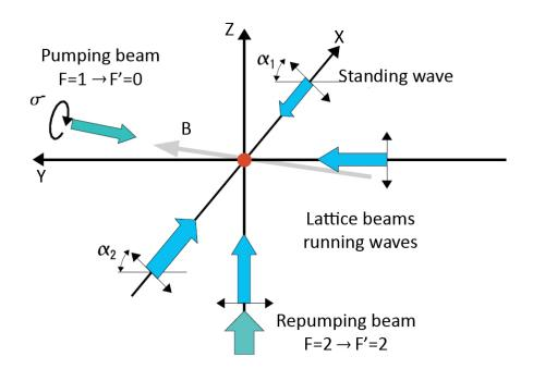
FIGURE 4.1: Laser beams setup for the 3D Raman sideband cooling, following the setup by Treutelin [29] and Fölling [13]. Two running waves and two counter propagating beams form the lattice. This configuration is more stable than 6 counterpropagating beams. All beams are polarized in the y-z plane to maximize Raman coupling for a magnetic field in that plane. [13].
