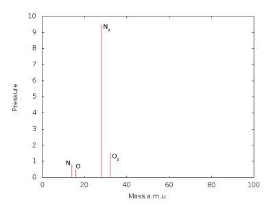
FIGURE 3.18: Fingerprint of an air leak [23]
