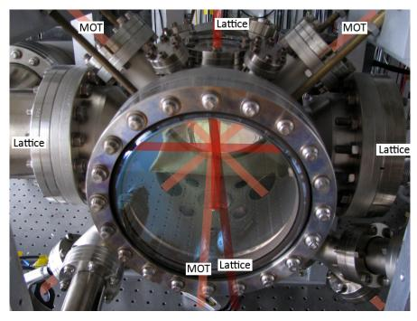
(b) Main chamber and the laser beams, MOT beams and optical lattice beams overlap in the center of the chamber.
