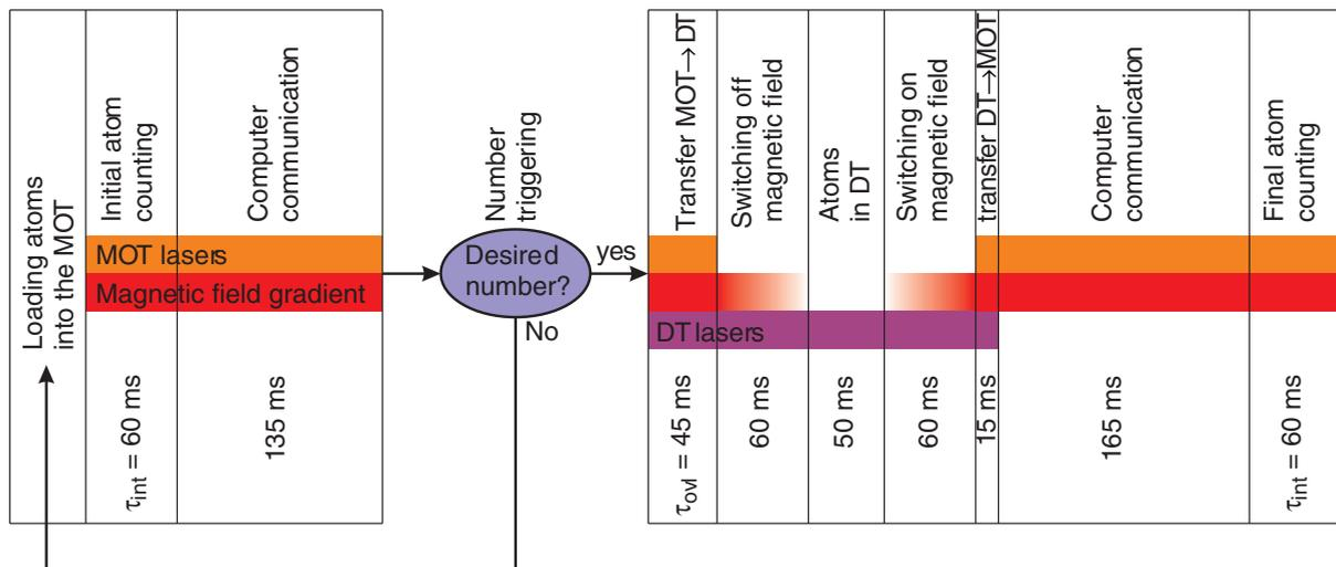
**Figure 3.** Experimental sequence for preparing a desired number of atoms  $n$  in the DT using our number-triggered loading scheme. At the end of the sequence, the atoms are transferred back into the MOT in order to measure their number.
