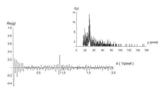
Figure 4.2: Histogram of measured distances and its fourier transform. The only one prominent contribution at  $k_0 = 0.9336$  wells/pixel corresponds to the periodicity of  $\lambda_{\text{HDT}}/2$  in the object plane of the microscope objective. The inset shows the original function f(y). Here, for presentation purposes each delta function was replaced by a Gaussian with the width of 0.05 pixel.
