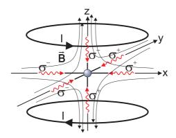
**Figure 2.2**: Three-dimensional schematic of the MOT. Two magnetic coils in anti-Helmholz configuration produce the quadrupole field. Six circularly polarized laser beams exert cooling and trapping forces.
