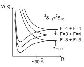
Figure 3.4: Schematic presentation of ground state collisions between two atoms. Two atoms in the ground state S + S approach each other on one of the attractive quasimolecular potential curves. If the atoms reach the separation of the level crossings (circles), the hyper fine structure state of the "quasimolecule" changes. As the result, the atoms gain the energy  $\Delta E_{\rm HFS}$  and leave the collision region on the repulsive quasimolecular potential.
