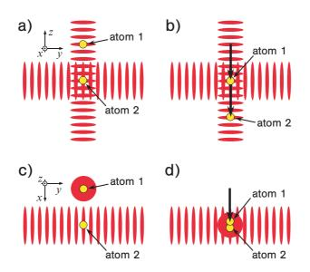
Figure 4.16: Insertion of an atom with the VDT into the HDT, which holds another atom, if the *y*-separation between atoms is smaller than the width of the optical tweezers. a)-b) During the axial insertion, atom 2 will be extracted downwards with the VDT out of the horizontal trap. c)-d) If the two traps are merged radially, both atoms will remain trapped in the HDT.
