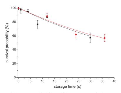
Figure 2.12: Measurement of the lifetime of the atoms in our dipole traps in presence of the optical molasses cooling. The squares present the measurement with the HDT. The solid line is an exponential fit to the experimental data. The circles present the measurement with the VDT with the corresponding exponential fit.
