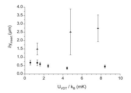
Figure 4.14: Insertion precision with and without cooling. The triangular points present the insertion precision for the experimental sequence without cooling of the atoms before re-insertion. The rectangular points are the results of the insertion precision with the cooling step. The depth of the HDT was fixed. In this experiment we have used the axial insertion method. Every point corresponds to about 25 repetitions of the experiment.
