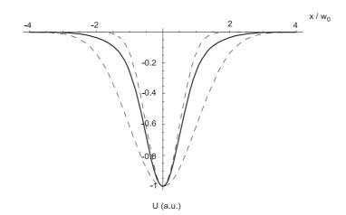
Figure C.5: Transverse shape of the standing wave dipole trap from two different Gaussian beams with the beam sizes  $w_0$  and  $2w_0$ . The profiles of the individual Gaussian beams are shown as dashed lines. The solid line presents the resulting radial shape with the width of  $1.3w_0$ .
