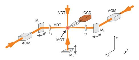
Figure 4.1: Scheme of the experimental setup for atom rearrangement. Atoms in the HDT can be moved along the y-direction using the optical "conveyor belt" technique, whereas the movement in the x-direction is realized by tilting the mirrors  $M_1$  and  $M_2$ . Atoms in the VDT can be transported along the z-direction by moving the retro-reflecting mirror  $M_3$ . The imaging optics is situated perpendicularly to the plane of the traps.
