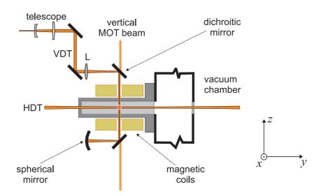
**Figure 2.7**: Beams of the HDT, VDT and the vertical beam of the MOT. Lens L focuses the incoming beam of the VDT at the position of the MOT. This beam is combined with the vertical beam of the MOT using a dichroic mirror. The spherical mirror retro-reflects the beam of the VDT to create a standing wave pattern. The beams of the HDT are focused at the position of the MOT and cross the VDT.
