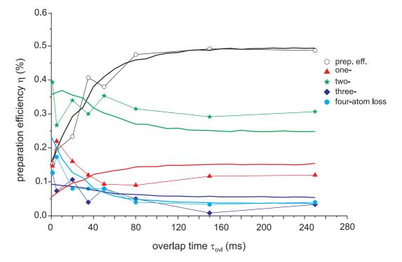
Figure 3.13: Simulation of the preparation efficiency for N = 10 as the function of the overlap time between the MOT and the HDT (open circles). Additionally, the probabilities of one-, two-, three- and four-atoms losses are shown. Solid lines show the result of the simulation.
