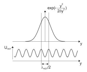
Figure 4.26: Probability distribution to join two atoms in one well. Integration of the distribution over the size of the potential well of the HDT gives the probability  $p_{\text{theor}}$  to joint two atoms in one potential well of the standing wave of the HDT.
