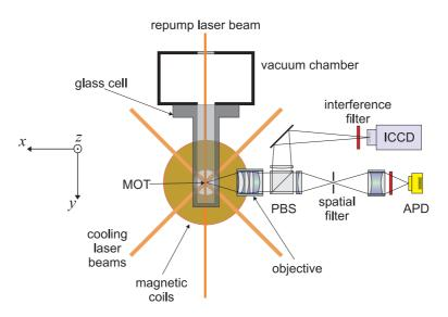
**Figure 2.4**: Experimental setup with the detection optics for the MOT fluorescence. The fluorescence light is collected and collimated by an objective. One part of the fluorescence signal is spatially and spectrally filtered and detected with an avalanche photo diode (APD). The other part is only spectrally filtered and sent into an intensified CCD camera.
