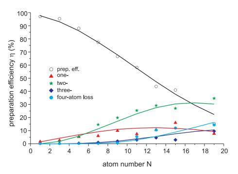
Figure 3.12: Simulation of the preparation efficiency of the atoms in the HDT (open circles). Additionally, the probabilities of one-, two-, three- and four-atoms losses are shown. The result of the simulation is shown as solid lines.
