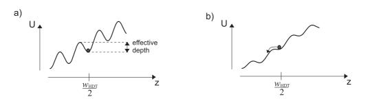
Figure 4.5: Decrease of the effective depth of the potential well. Due to the Gaussian shape of the confining potential of the HDT in the z-direction, the depth of the standing wave pattern reaches its minimum at the distance  $w_{\rm HDT}/2$  from the axis of the HDT. If the effective depth is larger than zero, the atom remains trapped in the standing wave and will be finally extracted with the VDT a). If the depth is smaller, the atom always rolls down during the extraction b).
