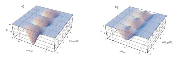
Figure C.1: Trapping potential in the x-z-plane. a) Two beams without any displacement (d = 0). b) Two Gaussian laser beams are displaced by one waist of the beam  $(d = w_{\text{VDT}})$ . The energy scale is in arbitrary units, but the same for a) and b). The scale in the z-direction is stretched by about one order of magnitude for the visualization purposes.
