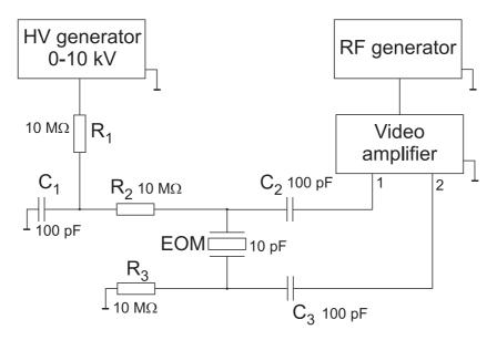
Figure B.1: Driving electronics of the EOM.
