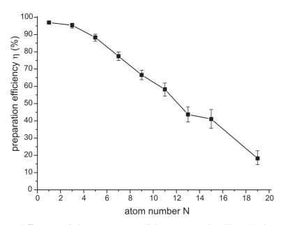
Figure 3.3: Efficiency of the preparation of N atoms in the HDT. Each point is the result of 300 successful detections of exactly N atoms by the discriminator.
