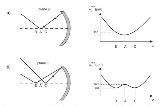
Figure C.4: Incoming and the reflected beams in planes  $\alpha$  and  $\beta$ . a) In the plane  $\beta$ , the waists of the incoming and of the reflected beams are at point A, corresponding to the center of curvature of the spherical mirror. b) In the plane  $\alpha$ , the waist of the incoming beam is at point B and of the reflected beam is at point C. On the righthand side is the profile along the beam axis z of the beam size of the resulting interference pattern in each case.
