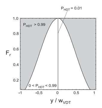
**Figure 4.9**: Contour plot for  $P_{\text{HDT}}(y_{\text{T}}^{\min}, F_{\text{r}}) = 0.99$ . Outside the white area atoms will remain trapped in the HDT with at least 99 % probability.
