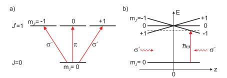
**Figure 2.1**: One-dimensional picture of the MOT. a) A model atom with J = 0 and J' = 1. The transitions with  $\Delta m_{\rm J} = -1$ , 0, 1 can only be excited by  $\sigma^-$ ,  $\pi$  and  $\sigma^+$ -polarized light, respectively. b) A magnetic field gradient shifts the Zeeman sublevels such that the laser light from the beam from the right is preferentially absorbed, pushing the atom back to the center.
