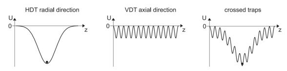
**Figure 4.4**: Trapping potentials along the *z*-axis. The trapping potential in the overlap region of the two traps is the sum of the Gaussian profile of the radial confining potential of the HDT and of the standing wave of the VDT. An atom at the bottom of the HDT experiences light forces of the standing wave, too.
