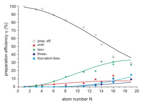
Figure 3.11: Simulation of the preparation efficiency of the atoms in the MOT (open circles). Additionally, the probabilities of one-, two-, three- and four-atom losses are shown. The result of the simulation is shown as solid lines.
