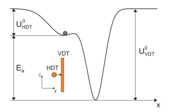
Figure 4.17: Radial potential of the two traps. During the radial merging of the traps, an atom in the radial potential of the HDT has a potential energy  $E_{\rm a}$ , relative to the bottom of the potential well of the VDT. The inset shows the respective geometry of the traps.
