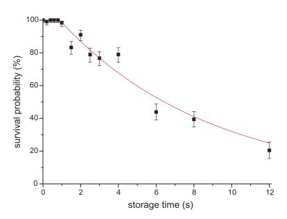
Figure 2.9: Measurement of the lifetime of the atoms in the HDT. The solid line is an exponential fit to the experimental data. Every point presents the result of about 30 repetitions of the sequence.
