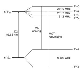
Figure 2.3: Simplified level scheme of the Cs atom. Shown are the transitions used for cooling and repumping in the MOT.
