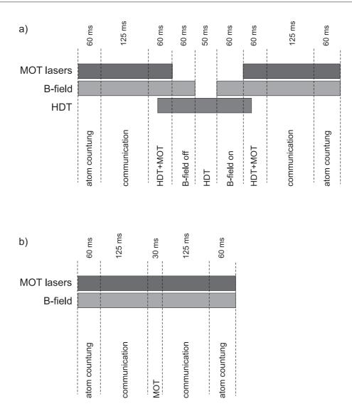
**Figure 3.2**: Experimental sequences of the preparation efficiency measurement. a) After counting the atoms, they are transferred from the MOT into the HDT and the magnetic field gradient is switched off. The atoms are then stored in the HDT. Finally, the magnetic field gradient is switched on and the atoms are transferred back into the MOT for counting. b) The same sequence but without the steps involving the HDT.
