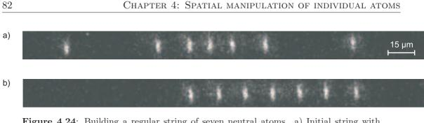
Figure 4.24: Building a regular string of seven neutral atoms. a) Initial string with randomly separated atoms. b) The same string after rearranging six out of the seven atoms with our distance control operation.
