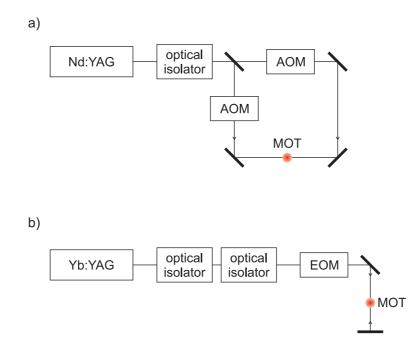
**Figure 2.8**: Block diagram of the laser systems of our dipole traps. a) The beam from a Nd:YAG laser is divided into two parts to create the horizontal standing wave dipole trap, overlapping with the MOT. b) The vertical standing wave dipole trap is created by retro reflecting the beam from an Yb:YAG laser. See text for details.
