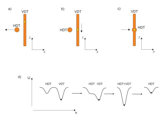
Figure 4.11: Radial insertion of an atom. a) An atom in the VDT after the extraction. The traps are separated by moving the HDT along the x-direction. b) The atom in the VDT is transported to the z-position of the HDT. c) The traps are merged by moving the HDT along the x-direction towards the VDT. d) Evolution of radial potentials of the traps along the x-axis for steps b) and c).
