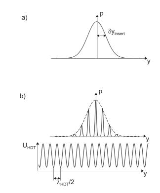
Figure 4.12: Spatial distribution p(y) with the width  $y_{\text{insert}}$  is projected onto the standing wave of the HDT as both traps are merged (a). This distribution after the projection (b). The width of the envelope remains almost unchanged, but the probability is spatially modulated with the periodicity of the HDT.
