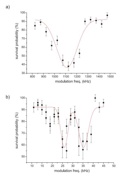
**Figure 2.10**: a) Axial oscillation frequency of the VDT. The points present the measured survival probability after parametric heating followed by the adiabatic lowering of the trap depth. The curve is a fitted Gaussian. b) Radial oscillation frequencies. The measured data (points) are fitted with a sum of two Gaussians. Every data point is the result of about 20 repetitions with on average 5 atoms per repetition.
