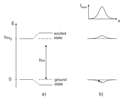
Figure 2.6: Light shifts for a two-level atom. a) Red-detuned light ( $\Delta < 0$ ) shifts the ground state downwards and the excited state upwards by the same amount. b) A spatially inhomogeneous field like a Gaussian laser beam produces a ground state potential well, where an atom can be trapped.
