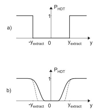
Figure 4.6: Probability for an atom to remain trapped in the HDT after the extraction. a) atoms at T = 0 K. b) atoms at temperatures  $T_1$  (solid line) and  $T_2$  (dashed line), with  $T_1 > T_2$ .
