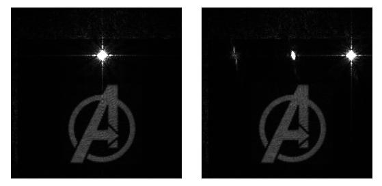
Fig. 5.1: Demo pattern "Averangers" with the zeroth-order spot untouched (left) and with attenuated zeroth-order spot (right). If the zeroth-order spot is too strong, its fringes affect the target pattern. The measured demo pattern has a size of  $1.2 \text{ mm} \times 1.2 \text{ mm}$ .
