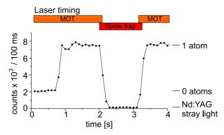
**Figure 1.7**: Transfer of a single atom between MOT and dipole trap. Once the atom has been transferred to the dipole trap, the recorded fluorescence signal drops to the stray-light background. Transfer back to the MOT reveals the presence of the atom by observing its fluorescence.
