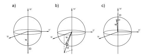
**Figure 1.25**: Adiabatic population transfer in the Bloch vector model, before (a), during (b), and after (c) the frequency sweep across the atomic resonance.
