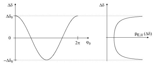
**Figure 2.21**: a) The average detuning difference  $\Delta \delta$  is shown as a function of the initial phase  $\varphi_0$ , according to Equation (2.35) and case II, see text. b) Corresponding probability distribution  $p_{\text{E,II}}(\Delta \delta)$  according to Equation (2.37).
