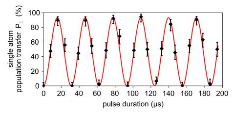
**Figure 2.11**: Demonstration of qubit rotations of individually addressed single atoms. Each point shows the averaged population transfer of approximately 40 single atom events. The Rabi oscillations have an excellent contrast of  $C = 99.1^{+0.9}_{-3.7}\%$ .
