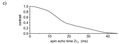
Figure 2.22: Measurement of axial position fluctuations of the dipole trap. (a) Experimental setup. The relative optical phase between the two trapping beams is measured interferometrically. (b) The Allan deviation of the phase fluctuations, calculated from the resulting data traces according to Equation (2.45), is plotted versus the averaging time on a logarithmic scale. (c) The expected spin echo contrast is shown as a function of the spin echo time according to Equations (2.28) and (2.46).
