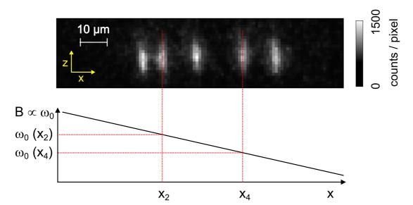
**Figure 2.1:** Image of a string of five trapped atoms. A magnetic field gradient introduces a position dependent atomic resonance frequency. As an example, addressing of the second and the forth atom of the string requires knowing the respective resonance frequencies  $\omega_0(x_2)$  and  $\omega_0(x_4)$ .
