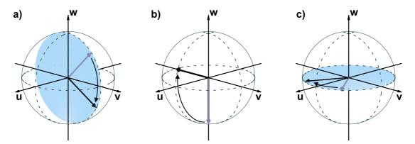
**Figure 1.18**: Bloch vector dynamics on the Bloch sphere. (a) Resonant driving corresponds to a rotation around the u axis. (b) A  $\pi/2$  pulse rotates the Bloch vector from a perfectly polarized state into the uv plane corresponding to a superposition of states. (c) If the Bloch vector is not driven by the external field, it precesses freely around the w axis.
