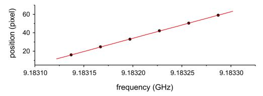
Figure 2.3: Calibration of the atomic resonance frequencies. Each data point shows the center position of a fitted intensity distribution as in Figure 2.2 (c). The error bars are too small to be displayed here. From the slope of the linear fit we infer  $\omega'/2\pi = 3.71 \pm 0.03 \text{ kHz}/\mu\text{m}$ .
