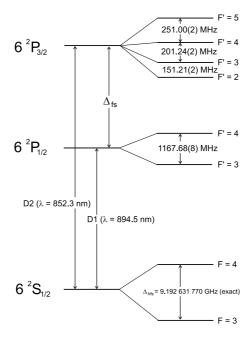
Figure 1.4: Level scheme of the cesium D-doublet.
