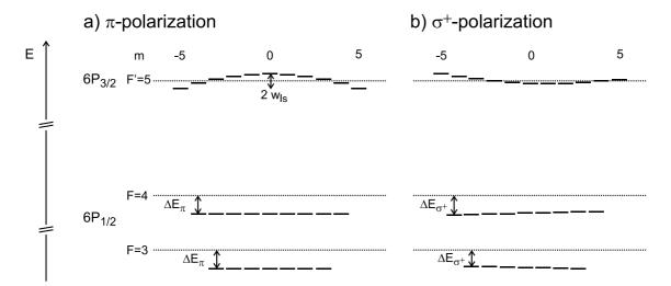
Figure A.1: Light shift of the Zeeman multiplicity of the two ground states and the F'=5 – excited state of the D2 transition for pure  $\pi$  (a) and pure  $\sigma^+$  polarization (b) of the electro-magnetic field. The maximum splitting of the Zeeman levels due to the tensorial contribution to the light shift of the excited state is denoted by  $2w_{ls}$ . The dotted lines show the unperturbed states. For illustration, the energy scale is interrupted twice.
