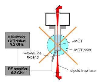
**Figure 1.19**: Setup for microwave spectroscopy. The microwave signal at 9.2 GHz is created by a synthesizer and amplified. An open X-band waveguide pointed towards the MOT is the most efficient antenna to maximize the microwave intensity at the position of the trapped atoms.
