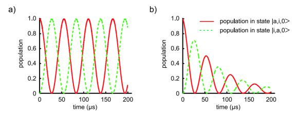
**Figure B.2**: Calculated time evolution of the four-photon Rabi oscillation. The states  $|a,i,0\rangle$  and  $|i,a,0\rangle$  coherently exchange energy at the Rabi frequency  $\Omega_{\rm eff}$ . (a) Without dissipation,  $\Gamma = \kappa = 0$ . (b) With dissipation. A list of all parameters can be found in Table B.1.
