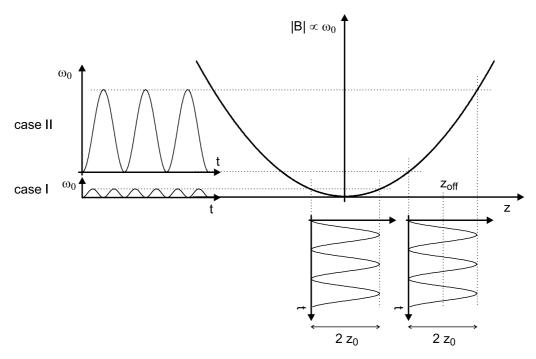
Figure 2.20: Modulation of the atomic resonance frequency  $\omega_0$  due to the radial oscillation (along z) of the atom in the dipole trap. If the trap is coaligned with the symmetry plane of the magnetic field ( $z_{\text{off}} = 0$ ), the amplitude of the frequency modulation is small (case I). In the case of a misalignment ( $z_{\text{off}} > z_0$ ), the modulation amplitude increases (case II) and the modulation occurs at half the frequency of case I.
