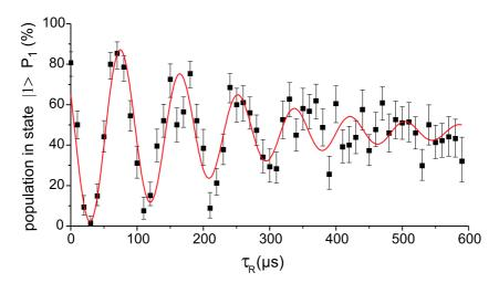
Figure 2.15: Decay of Ramsey fringes due to inhomogeneous broadening of the atomic resonance frequency. The data points show the measured population in state  $|1\rangle$  as a function of the time delay  $\tau_{\rm R}$  between the two  $\pi/2$  pulses. Every data point is averaged over 10 experimental runs with about 5 atoms each. The fit according to Equation (2.21) reveals an inhomogeneous dephasing time of  $T_2^* = 270 \pm 25~\mu{\rm s}$ .
