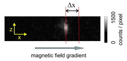
**Figure 2.7**: Measurement of the addressing resolution. A single atom in the dipole trap is subjected to a  $\pi$  pulse. The microwave frequency is set such that it is resonant with a position at the distance  $\Delta x$  away from the atom.
