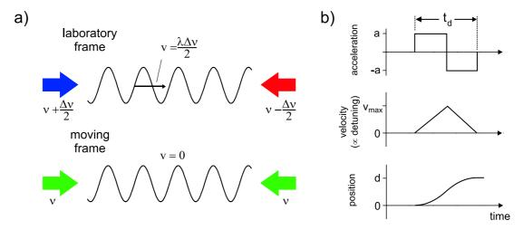
Figure 1.12: Working principle of the optical conveyor belt. (a) If the counterpropagating beams are detuned with respect to each other, the reference frame in which both beams are Doppler shifted to the same frequency is moving at the velocity v. (b) In order to transport an atom over the distance d, we expose it to constant acceleration and deceleration.
