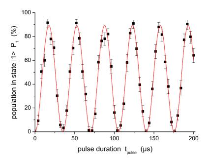
Figure 1.22: Rabi rotations between states  $|0\rangle$  and  $|1\rangle$  in a homogeneous magnetic offset field. Every data point shows the average population in state  $|1\rangle$  of 5 shots with 11 atoms each. While the maximum detected population in  $|1\rangle$ ,  $P_{\text{max}}$ , is limited by atom losses due to cold collisions, the fringe contrast  $C = 100^{+0.0}_{-1.8}$  % is excellent. The solid line is a fit according to Equation (1.24).
