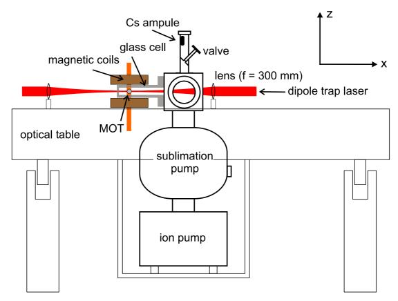
**Figure 1.2**: Side view of the vacuum system. A large cut-out of the optical table allows us to place the two vacuum pumps underneath the table surface. Cesium atoms are provided by a cesium reservoir which is connected to the vacuum chamber by a valve. For optimum optical access we perform all experiments in a rectangular glass cell which is attached to the vacuum system. All optical elements are set up outside the vacuum chamber.
