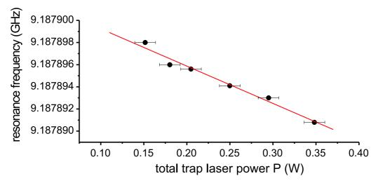
Figure 2.9: Measurement of the differential light shift of the qubit transition. We record Fourier-limited spectra with a  $\pi$  pulse time of 200  $\mu$ s for different trapping laser powers. Here, the atomic resonance frequencies obtained from this measurement are plotted. The total differential light shift obtained from the linear fit is dominated by the circularly polarized contributions of the trapping laser beams.
