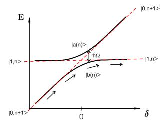
**Figure 1.23**: Adiabatic population transfer in the dressed state picture. The eigenstates  $|a(n)\rangle$  and  $|b(n)\rangle$  of the coupled atom – photon system do not intersect at the atomic resonance  $\delta=0$ . By sweeping the microwave frequency from large negative to large positive detuning, a spin flip occurs because the wavefunction adiabatically follows the eigenstate  $|a(n)\rangle$  or  $|b(n)\rangle$ .
