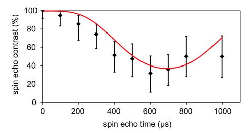
Figure 2.19: Spin echo contrast of the quantum register. Each data point is obtained from 40 single atom measurements of  $P_{\min}$ . The contrast is calculated according to Equation (2.30). The line is the result of the numerical calculation of Section 2.4.7 (Equation (2.42), Table 2.6).
