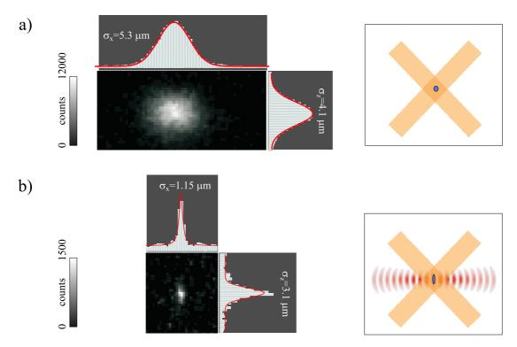
**Figure 1.10**: (a) Image of a single trapped atom in the MOT with an exposure time of 1 s. This is the same image already depicted in Figure 1.5 (b). (b) Image of a single trapped atom in a potential well of the dipole trap under continuous illumination with a 3-D optical molasses (exposure time: 0.5 s). On the right side, the respective laser configurations are shown.
