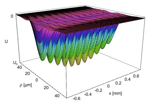
**Figure 1.6**: Three-dimensional view of the standing-wave trapping potential for  $w_0 = 19 \ \mu \text{m}$ . In x-direction, the wavelength has been stretched by a factor of 250 to visualize the individual potential wells.
