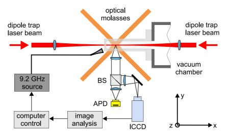
**Figure 2.4**: Experimental setup for single atom addressing. While the trapped atoms are illuminated by the optical molasses, an ICCD image is acquired. Subsequent analysis of this image determines the positions of the atoms and their resonance frequencies. The microwave source is then accordingly programmed by the computer control so that coherent manipulation of a selected atom qubit can be performed.
