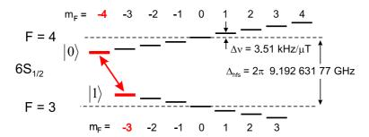
**Figure 1.15**: Zeeman splitting of the cesium ground state. By optically pumping the atom to the stretched Zeeman level  $|F=4, m_{\rm F}=-4\rangle$ , we can perform all coherent operations on the effective two-level system denoted by  $|0\rangle$  and  $|1\rangle$ .
