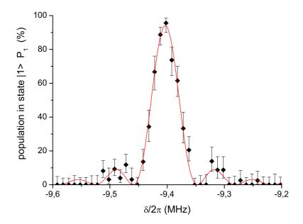
Figure 1.21: Fourier limited spectrum of a rectangular  $\pi$  pulse of 16  $\mu$ s duration. Every data point shows the average population in state  $|1\rangle$  of 5 shots with 5 atoms each. The solid line is a fit corresponding to Equation (1.23), with the fit parameters summarized in Table 1.1.
