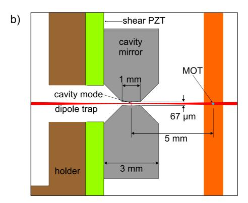
**Figure 3.1**: a) Picture of the high-finesse resonator which is set up in our laboratory. b) Planned experimental geometry for the deterministic transport of atoms from the MOT inside the cavity mode using our optical conveyor belt.
