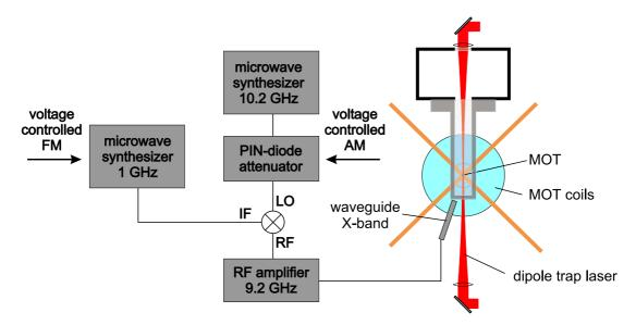
Figure 1.26: Setup for microwave spectroscopy using an adiabatic passage technique. The frequency modulation (FM) for the adiabatic frequency sweep is performed by an externally modulated synthesizer at 1 GHz whose signal is mixed with the microwave radiation at 10.2 GHz. The amplitude modulation (AM) is performed by a PIN-diode attenuator. Both FM- and AM-pulse shapes according to Equation (1.30) are controlled by the computer control.
