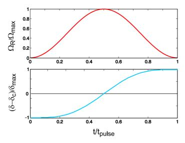
Figure 1.24: Microwave pulse shape for adiabatic population transfer. While the frequency detuning is symmetrically swept around a central detuning  $\delta_c$ , the microwave intensity is increased and decreased.
