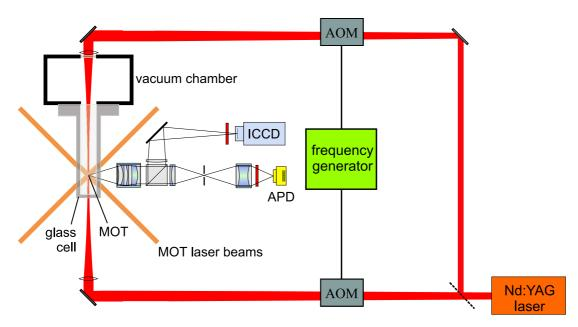
**Figure 1.13**: Experimental setup of the optical conveyor belt. Each beam of the standing-wave dipole trap is frequency shifted by an acousto-optical modulator (AOM). Both AOMs are driven by a phase-synchronous dual frequency RF-generator.
