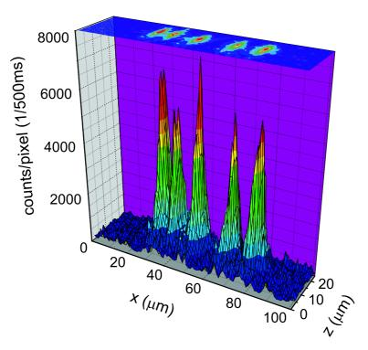
**Figure 1.11**: Image of a string of five trapped atoms. The atoms are trapped in separate potential wells and have an average separation of  $10 \mu m$ .
