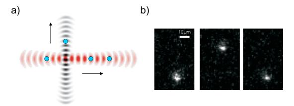
**Figure 3.2**: Single atom sorting with a vertical conveyor belt. a) Working principle. A selected atom is pulled out of the string of atoms, so that the horizontal conveyor belt can shift the relative position of the other atoms before the selected atom is placed back into the quantum register. b) First pictures of a single atom being transported up and down using the vertical conveyor belt.
