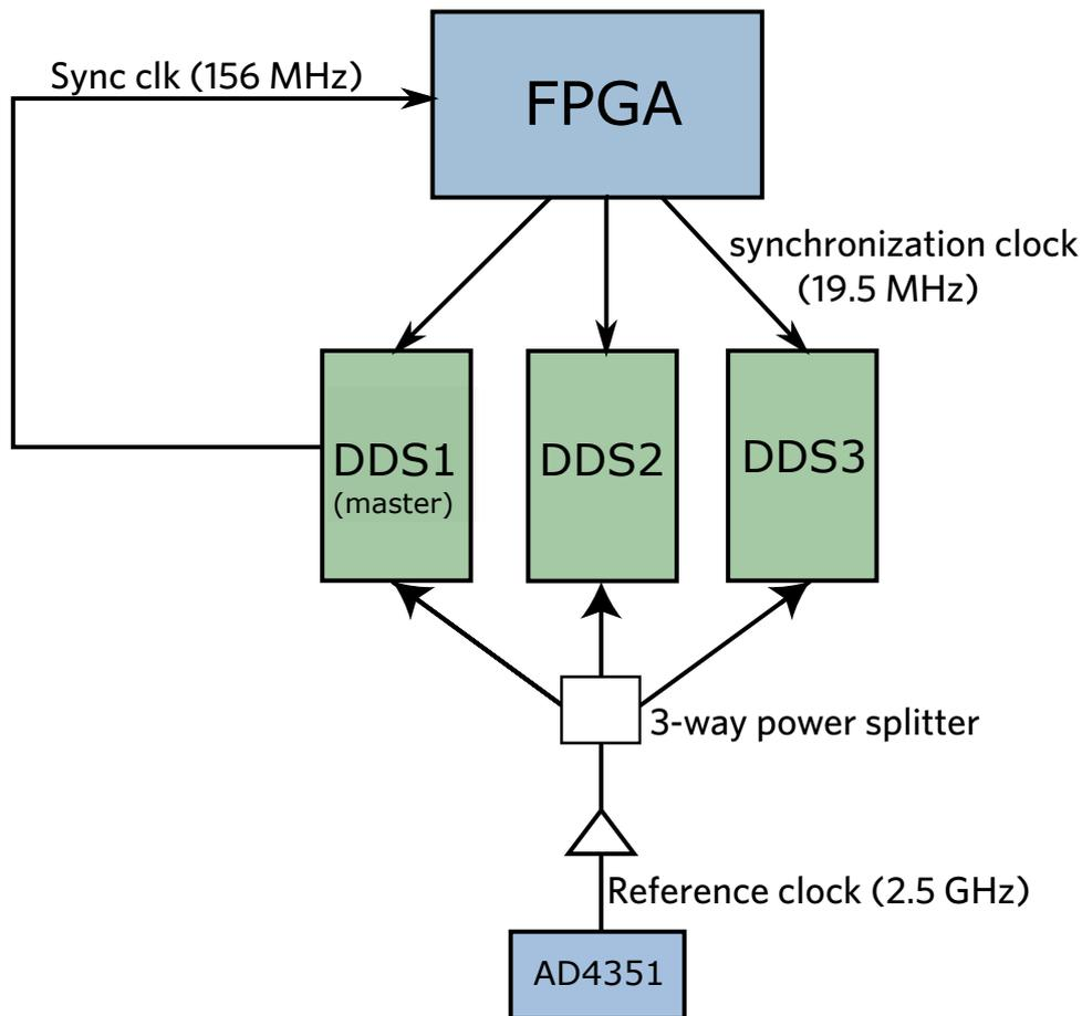
Figure 3.6: Block diagram of the different clocks and components used for synchronizing the DDS chips.
