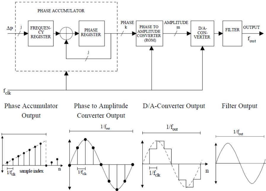
Figure 2.7: Block diagram of a direct digital synthesizer with the corresponding signal flow. Figure taken from [37]
