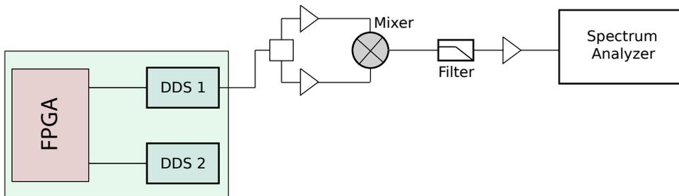
Figure 4.4: Setup for measuring the noise contribution from amplifiers. Here one signal is split in two and sent to the mixer. The phase noise measured only corresponds to phase noise contributed from other components in the setup.
