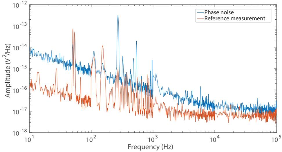
Figure 4.5: The curve on top shows the power spectral density of the phase noise measured using the setup shown in figure 4.1, before subtracting the reference. The bottom curve is the power spectral density of the reference measurement that originates from noise produced by the amplifiers shown in figure 4.4. The power measured in the reference setup needs to be subtracted to get the phase noise contribution of the DDS boards.
