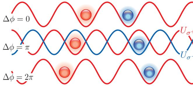
Figure 2.4: Illustration of state-dependent transport where the red-coloured (on the left-hand side) and blue-coloured (on the right-hand side) atoms constitute the two spin species of cesium. A  $2\pi$  optical phase difference between the two circular polarizations corresponds to transport over one lattice site.
