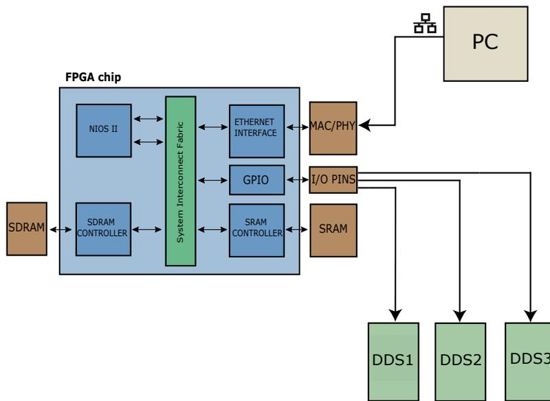
Figure 3.5: Schematic of the different modules used on the FPGA chip to communicate with the external peripherals. The double-sided arrows denote data transfer and the additional arrow for NIOS is the instruction set.
