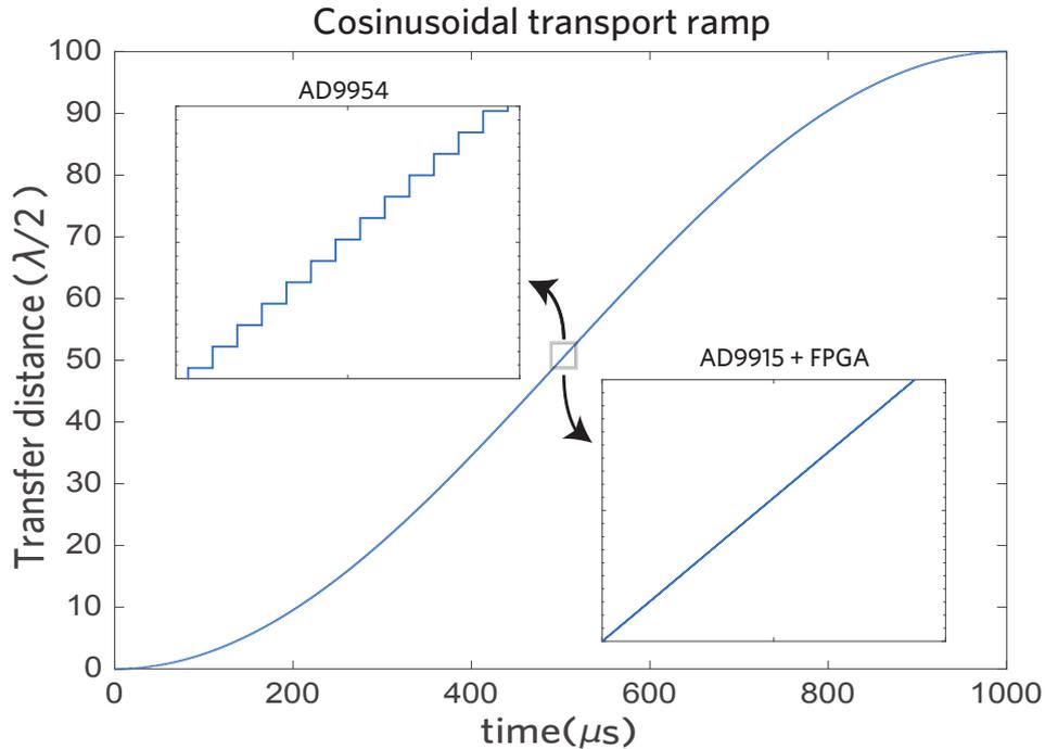
Figure 2.10: Phase ramp for transport over 100 lattice sites. Comparison of the AD9954 DDS chip with the versatile digital frequency synthesizer (AD9915+FPGA).
