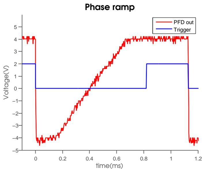
Figure 4.9: Phase ramp generated by a test setup consisting of a DE0-Nano FPGA board interfaced with an AD9910 DDS chip.
