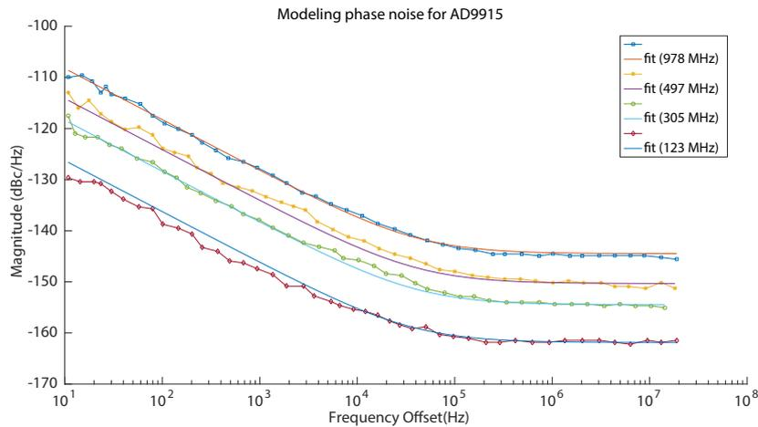
Figure A.3: Fitting phase noise data for AD9915 with equation A.1.
