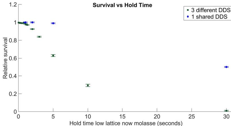
Figure 2.8: The relative survival of atoms for different hold times in two configurations. Data points shown as  $\square$  correspond to the case where all three DDS boards are used while in  $\diamond$  is the case where one DDS output is split into three instead. A significant increase in the survival time is noticeable when the lattice originates from the same RF source.
