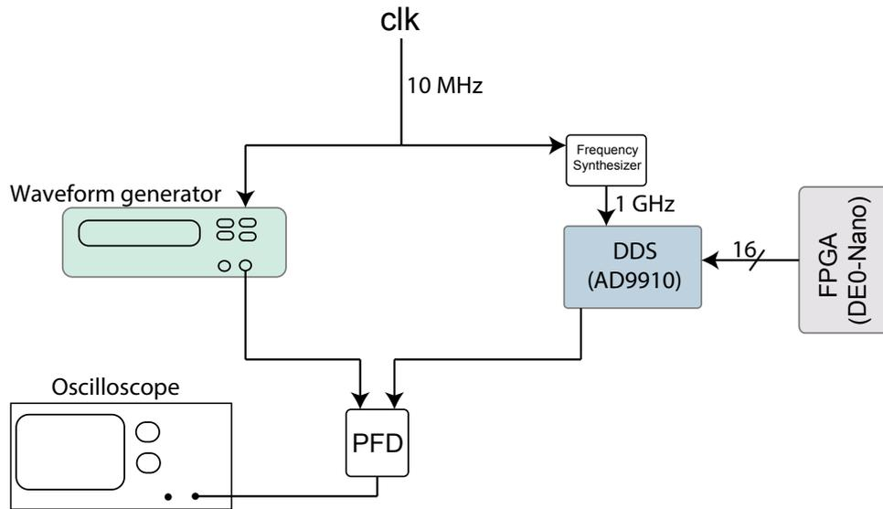
Figure 4.8: Setup for measuring the phase ramp generated by the test setup. The phase ramp of the DDS output is compared with a stable signal from a waveform generator, using a phase frequency discriminator.
