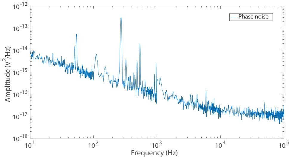
Figure 4.3: The curve shows the power spectral density of the two DDS boards measured using the setup shown in figure 4.1, before the reference is subtracted.
