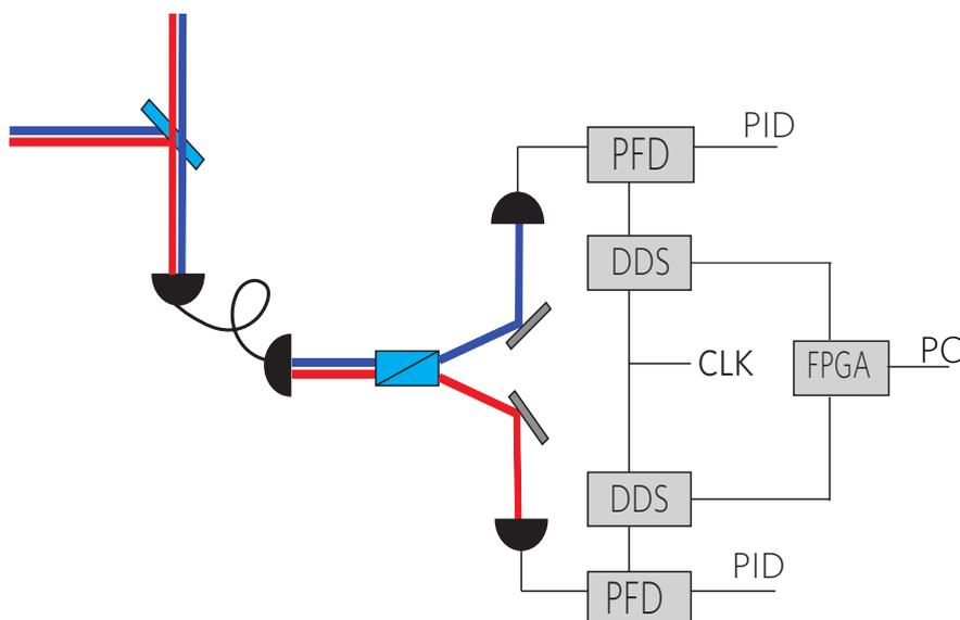
Figure 3.1: Schematic of the optical phase lock loop with the proposed control of DDS boards using an FPGA
