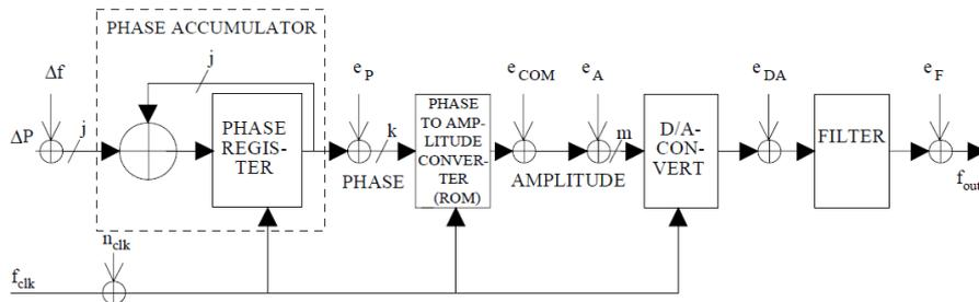
Figure 2.11: Block diagram showing the noise contributions to the DDS. Figure taken from [37]
