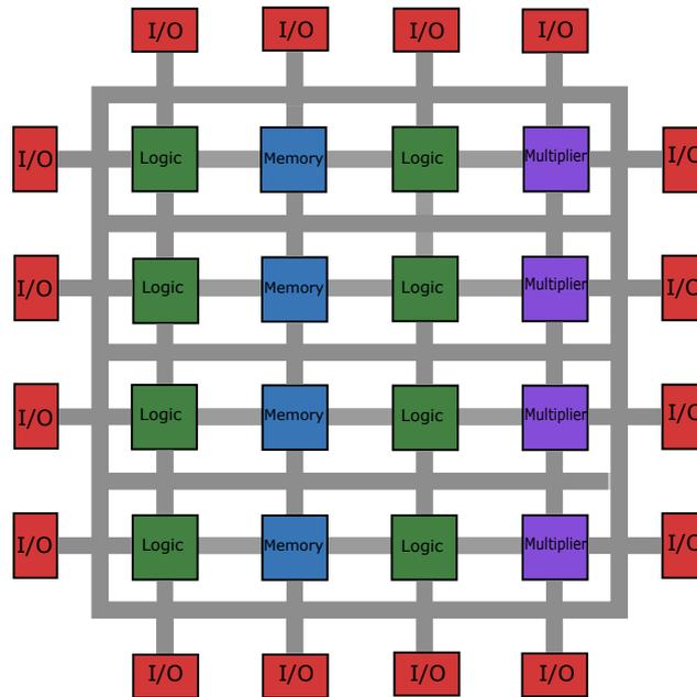
Figure 3.2: A simple schematic showing the basic architecture in an FPGA. All the different components are interconnected by programmable routing fabric
