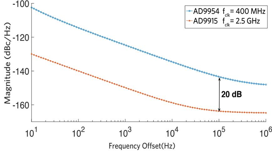
Figure 2.12: Extrapolated single sideband spectrum for the two DDS chips: AD9915 and AD9954. There is a suppression of noise by around 20 dB at an offset of 100 KHz. The reference clocks for the two are different.
