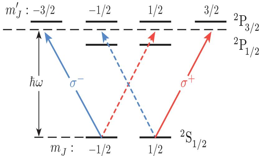
Figure 2.3: Fine structure representation of the cesium ground state.  $\omega$  is the frequency of the laser between the  $D_1$  and  $D_2$  transitions for the case where the potential contributions from the  $m_J = \pm 1/2$  magnetic sublevels of the two excited states cancel each other out.
