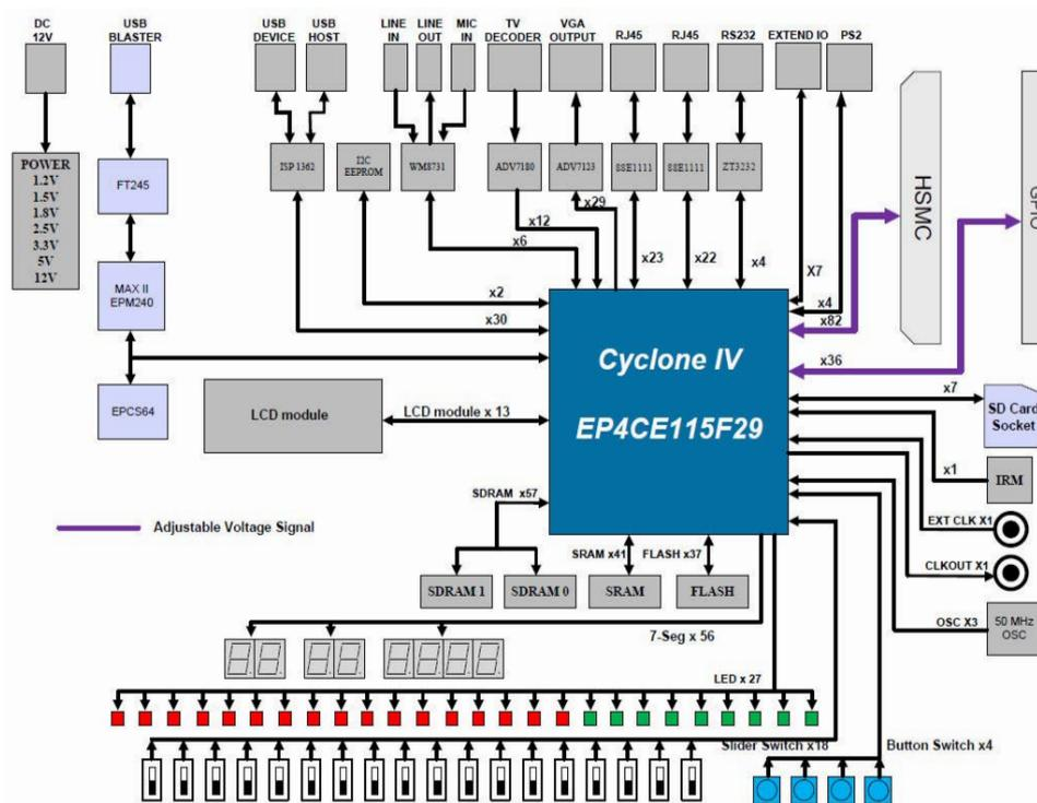
Figure 3.4: Block diagram of the FPGA board used, the DE2-115. Figure taken from [54].
