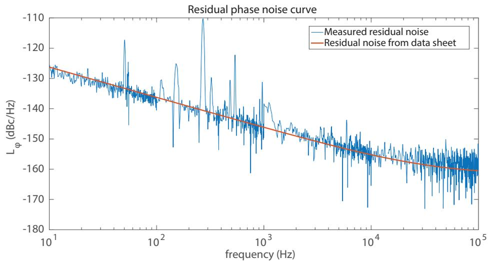
Figure 4.7: The residual phase noise from one output of the versatile digital frequency synthesizer is plotted against the residual phase noise of the AD9915 DDS chip. The carrier frequency is 123 MHz.
