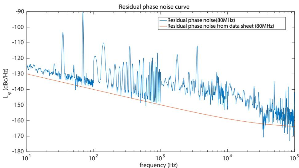
Figure A.1: Residual phase noise of versatile digital frequency synthesizer at 80 MHz. The phase noise from the data sheet is extracted for comparison.
