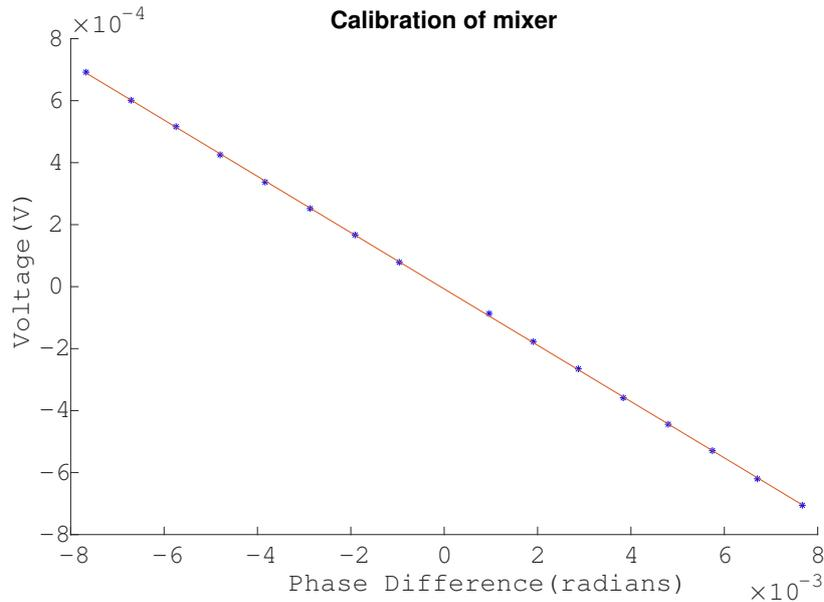
Figure 4.2: Calibration of the mixer constant. The phase difference of one of the DDS boards is incremented and the corresponding output voltage of the mixer is noted. The slope gives the mixer constant  $K_\phi$  which is 0.91 V/rad.
