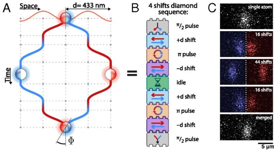
Figure 1.1: Digital atom interferometer. (A) A spin dependent optical lattice coherently transports the atom depending on its spin state,  $|\uparrow\rangle$  (red) or  $|\downarrow\rangle$  (blue), in opposite directions and finally recombines the two states, creating a diamond interferometric geometry. (B) Digital block representations of the operations mentioned in A. (C) Fluorescence images of atoms illustrate the splitting achieved. Figure taken from [12]
