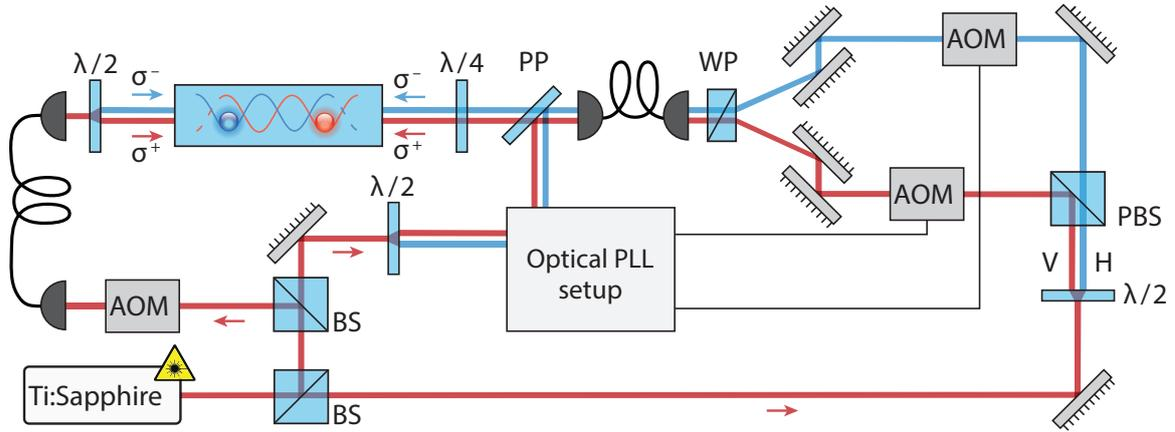
Figure 2.5: Schematic of the experimental setup. This sketch gives a simple overview of the beam paths and a few components of importance to this thesis. Several optical components needed for beam alignment are omitted, and so are the coils required to produce the magnetic fields. For a detailed sketch of the entire setup, see [33]. Figure taken from [33]
