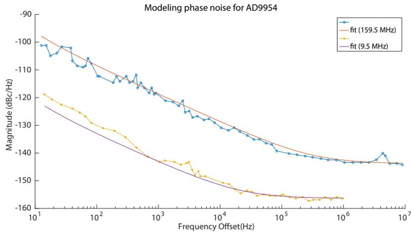
Figure A.2: Fitting phase noise data for AD9954 with equation A.1.
