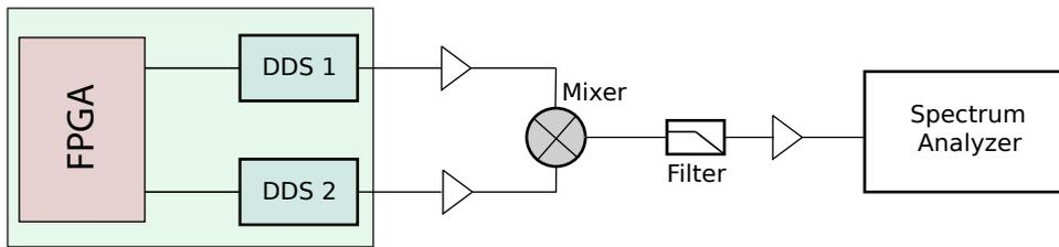
Figure 4.1: Setup for residual phase noise measurement. Two signals with equal amplitude and frequency but  $90^\circ$  phase difference are mixed using a mixer which generates a voltage proportional to the phase fluctuations between the two signals. The high frequency product from the mixer is filtered out using a low pass filter.
