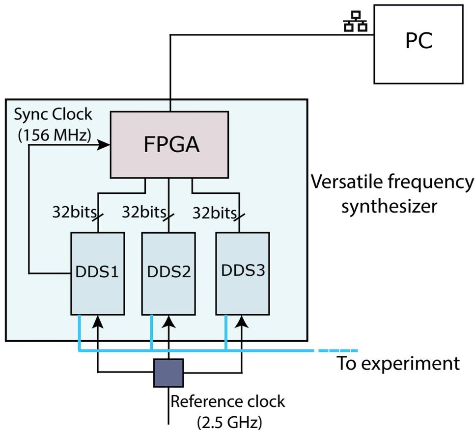
Figure 3.3: Block diagram of the versatile digital frequency synthesizer.
