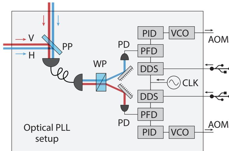
Figure 2.6: A simple schematic showing the basic components of the optical phase lock loop. Detailed working of the OPLL is explained in the text. Figure taken from [33]
