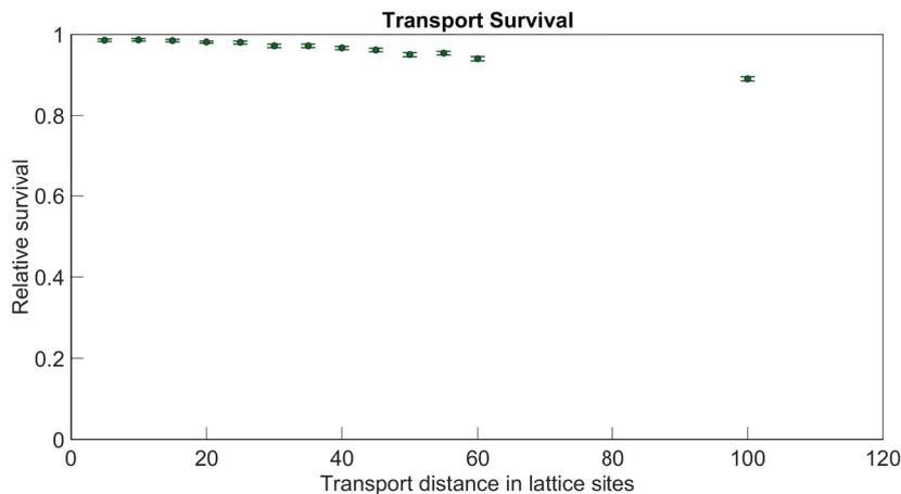
Figure 2.9: Transport survival for different transport distances. The survival probability drops as the transport distance is increased.
