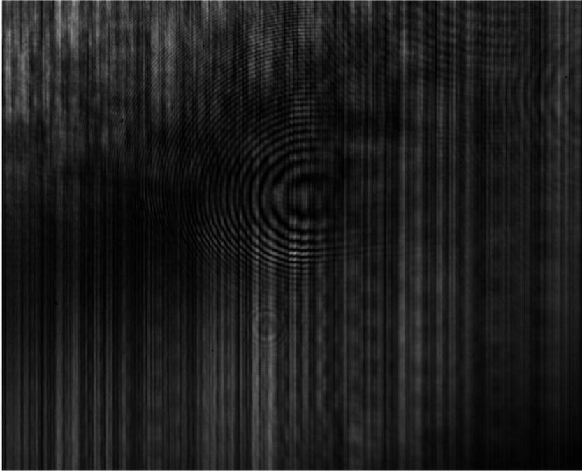
Figure 36: Intensity distribution on objective for diffraction grating (and phase correction)
