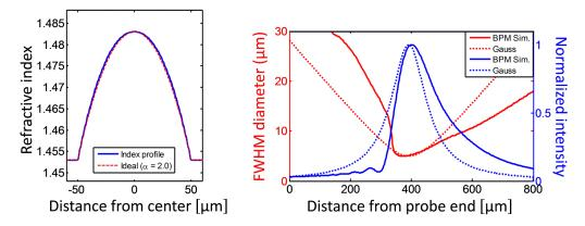
Figure 2.3: On the left-hand side, the refractive index profile of a GRIN fiber with  $\alpha = 2.15$  is shown (blue) with a comparison to a profile with  $\alpha = 2$  is shown. On the right, the beam widths and normalized on-axis intensities are given as a subject to the distance from the probe end. They reveal the typical behavior for a beam passing a lens with strong positive spherical aberration. The figure is taken from [26].
