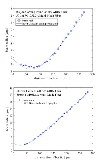
Figure 5.11: This figure shows measured output mode propagations of fiber assemblies made of single-mode, GRIN and multi-mode fibers. The upper beam propagation is measured for a Corning InfiniCor 300 fiber lens of  $380 \,\mu\text{m}$  length. The lower assembly is equipped with a Thorlabs GIF625 fiber lens of  $380 \,\mu\text{m}$  length.
