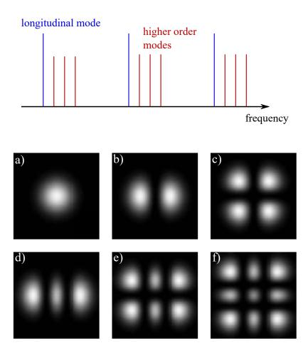
Figure 2.8: The upper part shows a cavity spectrum with longitudinal and higher order transversal ( $\text{TEM}_{nm}$ ) modes. In the lower one intensity distributions of higher order transversal modes are presented:
