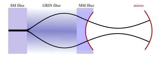
Figure 5.1: This figure shows the approach to install mode-matching optics into fiber cavity assemblies. The laser light is mode cleaned in a single-mode fiber, before its mode is conversed by GRIN fiber lens. The mirror is machined onto a piece of multi-mode fiber.
