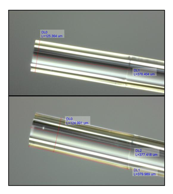
Figure 5.5: This figure illustrates the reproducibility of cleave lengths by showing two examples. Deviations at the given setting of  $380 \,\mu\text{m}$  are less than  $3 \,\mu\text{m}$ . The length calibration is done by measuring the fiber diameter, which is specified as  $(125 \pm 1) \,\mu\text{m}$ . Due to the finite size of the white colored joint region, discrepancies of the length measurements are expected. Due to the narrow joint region, they are well below  $5 \,\mu\text{m}$ .
