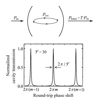
Figure 2.7: This figure illustrates the definition of the incoming power  $P_{in}$ , from which a part is coupled into the cavity. The power circulating in the cavity is called  $P_{circ}$  and the transmitted one  $P_{trans}$ , which is spectrally depicted in the lower part. Parts of this figure are taken from [2].
