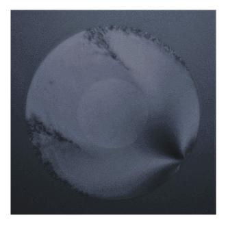
Figure 5.3: This figure shows an interferogram of a fiber cleaved with a too strong tension taken with the microscope introduced in section 3.4. On the lower right, the position of the blade impact and on the top and left the hackle is can be seen. The image is taken from [36].
