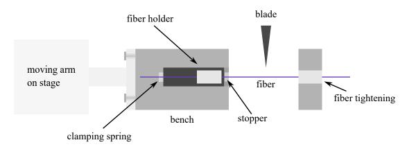
Figure 5.4: This figure illustrates the cleaver setup for cleave length control.
