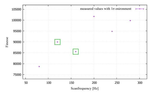
Figure 4.4: Estimated finesse values for different scan frequencies. The errors denoting the  $1\sigma$  uncertainty are solely given by the fit and are on the order of 4%, so that the errorbars are hardly visible.
