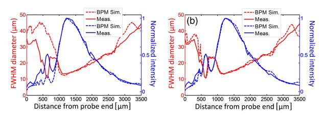
Figure 2.6: Prediction and measurement of the beam propagation after a fiber lens from 100/140 MMF POFC GRIN fiber. The prediction without a long ripple is displayed on the left, the one with it is on the right. The image is taken from [26].
