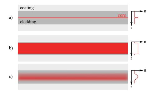
Figure 2.1: This sketch illustrates the structure of fibers with their refractive index profile. The light is guided in the core, which is surrounded by the cladding to create a refractive index transition. Around the fiber, a coating is applied for protection.
