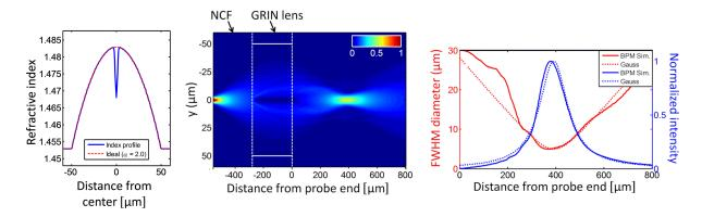
Figure 2.5: On the left, a refractive index profile is presented with  $\alpha = 2$  and a central dip of width  $w_{dip} = 1.5 \,\mu m$  $h_{dip} = 0.5$ . The central figure shows the spatial light intensity distribution illustrating the donut shape of the mode inside the GRIN fiber. The beam diameter at different distance from the fiber tip and the normalized on-axis intensities are displayed on the right. The image is taken from [26].
