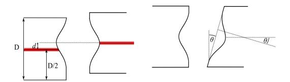
Figure 2.10: This figure illustrates the definition of decentrations of mirror and core (marked in red) d, as well as angles of the mirror with respect to the fiber axis normal  $\theta$ .
