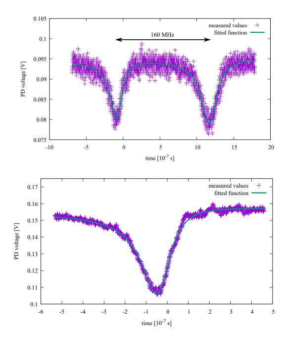
Figure 4.3: This figure shows measurement data to determine the resonance width and finesse with a scan frequency of 120 Hz.
