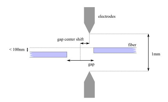
Figure 5.6: This figure illustrates the fiber alignment inside the fusion splicer used for this project. Among others the gap between the fibers and the position of the gap center are adjustable. Displacements of the fibers with respect to each other are less than 100 nm.
