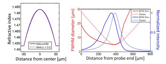
Figure 2.4: Here, similar to figure 2.4 an index profile of a GRIN fiber is displayed with  $\alpha = 1.85$ . Additionally, the beam widths as well as the normalized on-axis intensities are shown with respect to the fiber probe distance. As an exponent of  $\alpha = 2.15$  shows positive spherical aberrations, this one shows a strong negative one. This picture is taken from [26].
