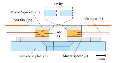
Figure 4.5: This figure shows a sketch of the cavity design. The image is adapted from [18].
