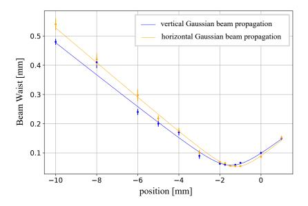
Figure 3.2: This figure shows the beam widths around the waist of the laser beam measured with the knife-edge method. A low ellipticity due to a slight mismatch of the waist positions is ascertainable. The image is taken from [36].
