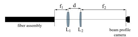
Figure 6.1: This figure illustrates the first attempt to measure a beam propagation with a beam profile camera and a system of lenses magnifying the beam by a factor of 25. To measure a complete propagation, the fiber assembly is pulled backward in steps of  $10 \,\mu\text{m}$ . For every step an image is taken, from which the brightness of every pixel is extracted. An elliptic Gaussian function is fitted to the brightness values to determine beam widths and ellipticities.
