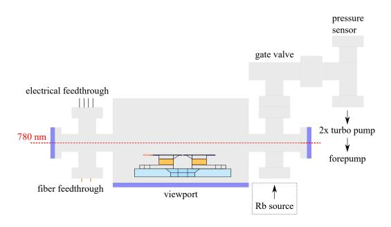
Figure 4.7: This figure shows a sketch of the assembled vacuum system for glue curing. In the future, it can be extended with a rubidium source to investigate the cause of finesse degradations.
