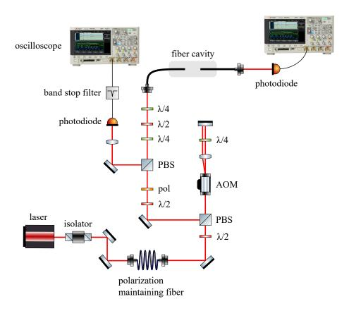
Figure 4.1: Optical setup for cavity alignment and lineshape observation.
