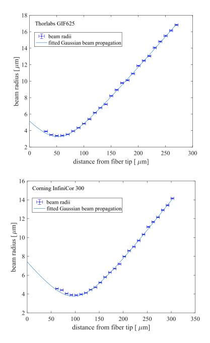
Figure 5.10: Measured output mode of a 780HP single mode fiber equipped with GRIN fiber lenses of  $380 \,\mu m$  length made of the Corning InfiniCor and the Thorlabs GIF625 fiber.
