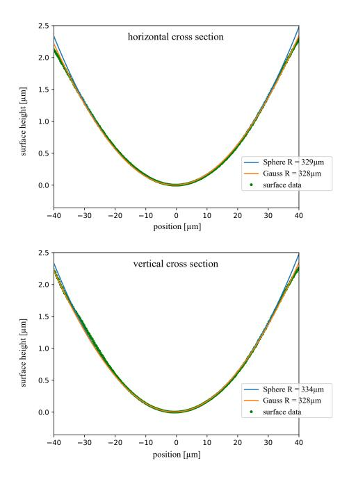
Figure 3.6: This figure shows the reconstructed cross-section in horizontal and vertical axis as well as the Gaussian and spherical fit with their corresponding radii of curvature. An excellent agreement between the radii of curvature is noticeable. The conformity of the parameters in horizontal and vertical direction indicates a low ellipticity. The image is taken from [36].
