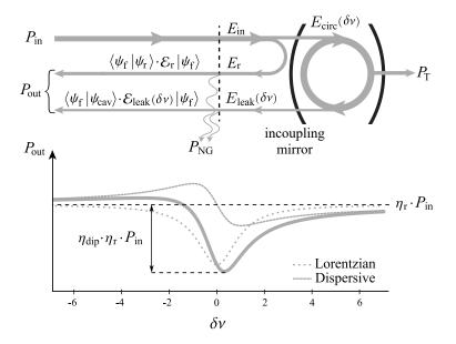
Figure 2.11: This figure illustrates the origin of the asymmetric reflection lineshape of fiber Fabry-Perot cavities. The light power propagating in reflection direction,  $P_{out}$ , is built up by the interference of  $E_r$  and  $E_{leak}(\delta v)$ , whereas some part of the power  $P_{NG}$  is not guided by the single-mode fiber. The image is adapted from [18].
