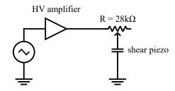
Figure 4.2: Electrical circuit for piezo high voltage supply.
