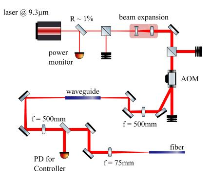
Figure 3.1: Sketch of the new fiber shooting setup.
