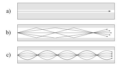
Figure 2.2: This figure shows ray tracing pictures of modes in a): single-mode fibers, b) multi-mode fibers and c): graded-index fibers. The image is taken from [22].
