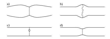
Figure 5.7: In this figure, different shapes of splices with unfavorable arc powers or durations are illustrated.:
