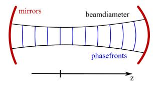
Figure 2.9: Fundamental Gaussian mode in a cavity.
