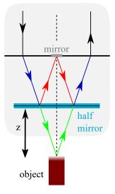
Figure 3.5: This figure shows the light paths in a Mirau objective. The image is adapted from [22].
