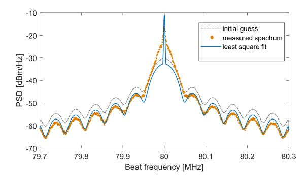
Figure 3.4: DSH spectrum at p = -44.4 dB fitted using the analytical expression (Eq. 3.3) which includes contributions from white frequency noise only. The estimated Lorentzian linewidth based on the fit is 5.093 kHz
