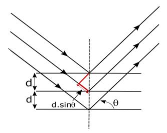
Figure 2.2: Bragg reflection from a periodic structure [29].
