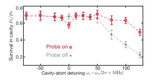
Figure 3.13: Relative survival rate  $(p_1/p_0)$  for atoms under continuous monitoring (red) or in the darkness (gray); the error bars represent the Clopper-Pearson confidence intervals (each data point corresponding to measurements of 300 to 1000 traces). The comparison is done for several frequencies of the monitoring cavity field. We attribute the discrepancies for far blue detunings to technical reasons (see text).
