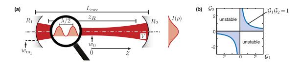
Figure 2.2: (a) Geometry of the fundamental  $\text{TEM}_{00}$  cavity mode. The radius of the Gaussian intensity profile diverges from the waist  $w_0$  and reaches a value  $w_m$  at the position of the mirrors. A standing-wave is formed due to the interference between counter-propagating circulating fields. (b) Stability diagram of an FP resonator. The colored region represents cavity geometries that allow the hosting of a stable mode.
