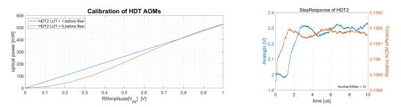
Figure 2.14: What we see is on the left is that the linearization of the AOM response works. On the right, we see a step response recorded using the internal data acquisition of the M3300A. This can be used to tune the feedback parameters automatically. Recording the traces of both the input and the output is helpful for debugging.
