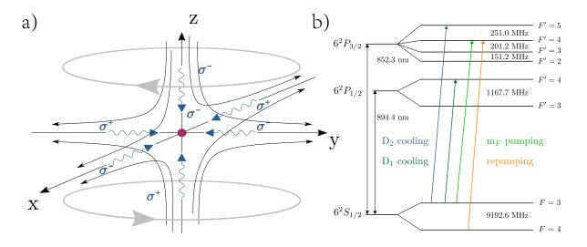
Figure 2.3: Three dimensional model of the MOT and optical transitions. (a) The grey circles indicate the current generating the quadrupole field. (b) The transitions used for cooling, imaging and state preparation.
