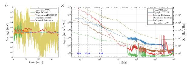
Figure 2.13: Voltage noise of the reference voltage. a) Drift of reference voltage. b) Relative intensity noise (RIN) power spectral density and the corresponding frequency noise PSD. The input noise of the M3300A ( $U_{Bias}$ ) is shown with and without an amplification of 20. Without amplification the coherence time is limited to 2 ms. The other components are so stable that the this limit improves 20-fold, after amplification.
