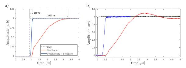
Figure 2.15: Step responses with and without additive feedforward control. Using feedforward control in conjunction with internal model control the modulation bandwidth can be increased from 230 kHz to above 3 MHz. The figures are adapted from [77, 78].
