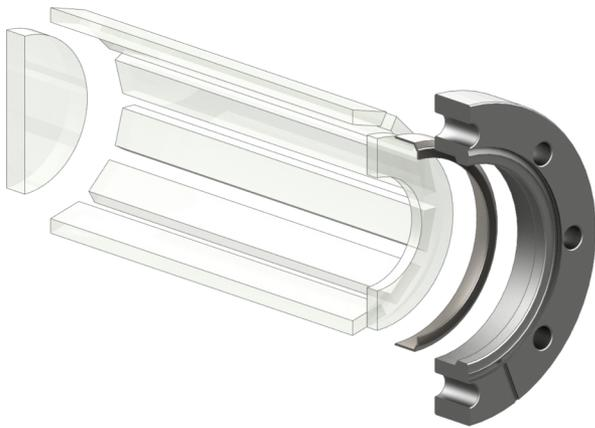
FIG. 1. Exploded view of half of the vacuum glass cell consisting of a round cover glass (thickness 9 mm, outer diameter 56 mm), 12 windows with a trapezoidal cross section (inner aperture size 13 mm  $\times$  150 mm, thickness 5 mm), a glass ring (thickness 5 mm, inner diameter 40 mm, outer diameter 68 mm), and a DN63CF stainless steel (316L) flange featuring a tantalum weld ring. The inner diameter is around 48.5 mm.
