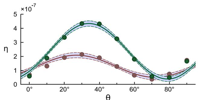
FIG. 3. Measured extinction ratio  $\eta$  as a function of the polariser angle  $\theta$  under atmospheric pressure (red) and vacuum (green). Data points refer to window no. 11, which exhibits the highest amount of birefringence (see Table I). Solid lines represent a fit of our model to the data. Instrumental uncertainty is below the marker's size. The vertical offset is caused by stray light from the 30 mW incoming probe laser beam. Dashed lines indicate the 68%-confidence region.
