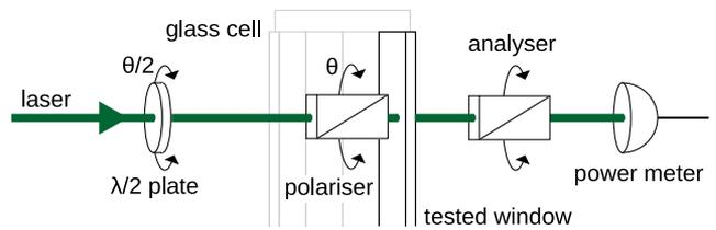
FIG. 2. A linearly polarised probe laser beam crosses a window. The linear polarisation angle  $\theta$  is set by the Glan-laser polariser (Thorlabs, Inc.) inside the glass cell. A power meter measures the minimum and maximum intensity after a second rotating Glan-laser polariser, which is used as an analyser. To suppress stray light, the power meter is placed at about 2 m distance.
