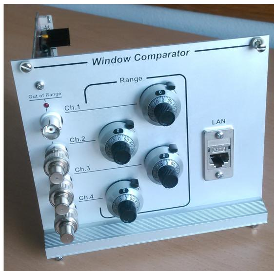
**Figure B.5.:** Front view of the window comparator device: The window sizes of four channels can be controlled by individual precision potentiometers. Out-of-Range conditions are indicated by light-emitting diodes and send to the lab computer via an Ethernet interface.
