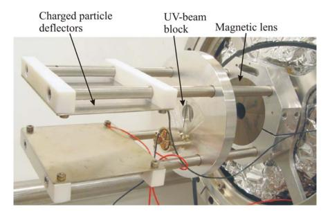
Figure 1.17: Experimental setup for UV-free He\* atom lithography.
