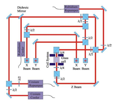
**Figure B.3:** Schematic diagram of the main experimental setup around the UHV-MOT. Cooling and repumping light at 852 nm are combined and superposed with the cooling light at 780 nm at a dichroic mirror. Laser beams at both frequencies are then split into six sub-beams, two for each dimension of the MOT. The x- and y- beams enter the glass cell at an angle of 45° from the vertical. (All beamsplitter cubes are polarizing.)
