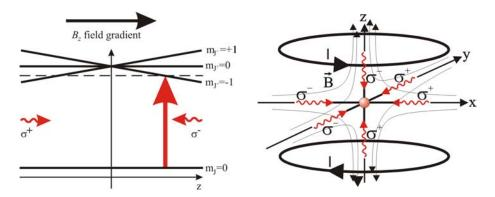
Figure 2.1: Magneto-optical trap (MOT). In the one dimensional picture (left), a magnetic field gradient lifts the degeneracy of the excited Zeeman sublevels. Therefore an atom travelling away from the magnetic minimum will move into resonance with a laser beam which applies a restoring force to the trap center. To apply this principle in three-dimensions (right), a pair of current-carrying coils in the anti-Helmholtz configuration provides the required linear field gradient.
