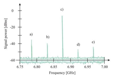
Figure 2.15: Spectral output of the microwave system for hyperfine evaporative cooling. Peaks (a)-(d) refer to the lower sideband, the carrier, the upper sideband, and the first and second harmonics respectively.
