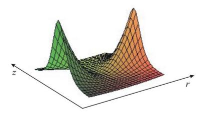
**Figure 1.15:** Equipotential surface of the hexapole magnetic lens for low-field-seeking atoms (Eq. 1.10). Due to the finite length of the lens the radially harmonic potential decays at both edges, which is here described by Eq. 1.14.
