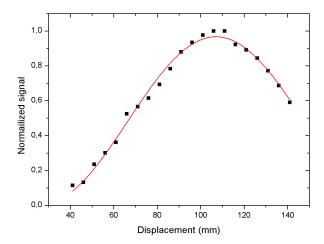
**Figure 1.9:** The transverse beam profile of the atomic beam as measured at a distance of 45 cm from the skimmer, at a source pressure of 15 mbar and a discharge voltage of 1200 V. Employing a cosine-squared fitting function, an angular beam spread of  $90 \pm 2$  mrad was obtained.
