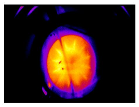
**Figure 1.18:** Atomic beam image after magnetic manipulation – the shadow of the UV-beam block runs diagonally across the center of the image. The scale is approximately 1:1.5.
