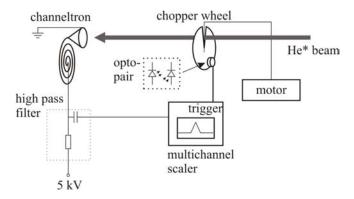
Figure 1.10: Experimental set-up for time-of-flight measurement.
