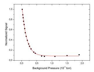
**Figure 1.13:** Determination of UV-photon contribution by quenching with argon gas, with an exponential decay fit, at a source pressure of 10 mbar and a discharge voltage of 1200 V. The residual signal at a background pressure of  $> 1 \times 10^{-3}$  torr is approximately 8 % of the total.
