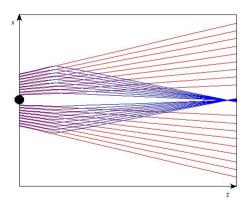
Figure 1.5: Schematic of proposed trajectories of He\* atoms (blue) and photons (red) in the UV-free experiment, in which the direct line-of-sight from the source to the exposure region is deliberately blocked. The lithographic exposure will take place at the position where the atomic beam is focussed into the shadow of the UV-radiation.
