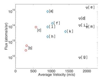
Figure 1.7: Comparison of the ANU liquid nitrogen-cooled He\* source (denoted as (a)) with other existing He\* sources. Triangles denote sources operated at room temperature (300 K), diamonds denote sources operated at liquid nitrogen temperature (77 K), and circles denote the new generation of He\* sources, operated at liquid helium temperatures (5 K). The labels (a)-(m) corresponds to References ([18]-[28]) respectively.
