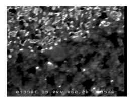
**Figure 1.3:** SEM images of a substrate exposed to a He\* beam at a source pressure of 11 mbar and a total discharge voltage of 1200 V, at  $1000\times$ ,  $6000\times$ , and  $60000\times$  magnification, respectively. In these images, gold appears as light and silicon as dark. The white perimeter in the second image denotes the region of interest for the last and highest level of magnification.
