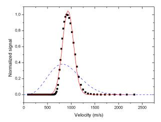
**Figure 1.11:** Velocity distribution of the He\* atomic beam for a source pressure of 11 mbar, normalized to a peak value of unity and fitted with a supersonic (solid line), and effusive (dashed line) velocity distribution, respectively.
