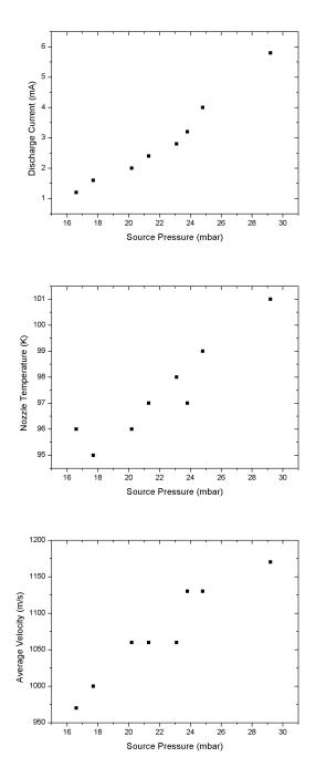
Figure 1.12: The dependence of discharge current, nozzle temperature, and average atom velocity respectively on the source pressure.
