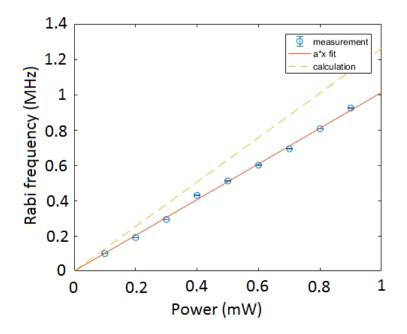
Figure 4.7: Rabi Frequency depending on the laser power
