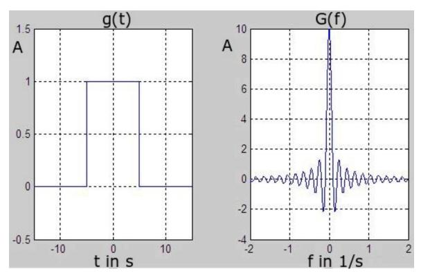
Figure 4.1: Box function g(t) and Fourier transform G(f) [34]
