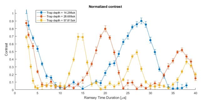
Figure 4.19: Combined plot of the quantum speed limit measurements at different trap depths
