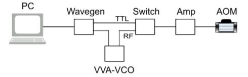
Figure 3.7: Schematic control circuit for the AOM; Amplifier: Mini Circuits (MC) ZHL-1-2W-S+, VCO: MC ZX95-78+, VVA: MC ZX73-2500+, Switch: MC ZASWA-2-50DRA+, Wavegen: Agilent 33522A
