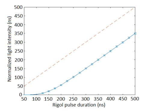
Figure 3.20: Integrated light intensity against programmed pulse length
