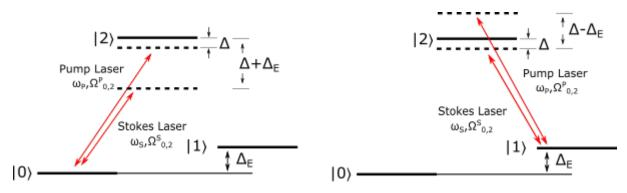
Figure 3.3: Cross coupling of the Pump and Stokes beams
