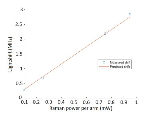
Figure 3.19: Comparison of calculated and measured light shift
