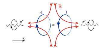
Figure 2.2: Field and laser beam configuration for a MOT [12]
