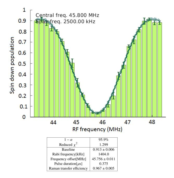
Figure 4.3: Raman spectrum with 375ns pulse length and 1.19mW of power per beam
