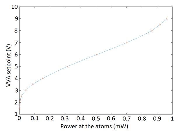
Figure 3.18: Calibration plot for the Raman beams
