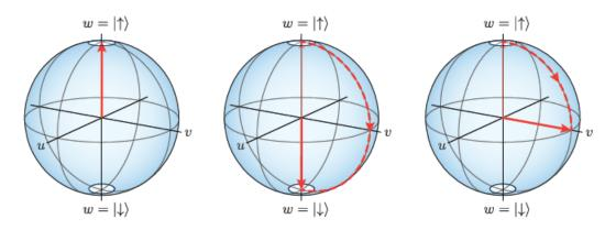
Figure 2.5: In the first picture, on the left, the atom is completely in the  $|\uparrow\rangle$  state. The middle picture shows a transfer to the  $|\downarrow\rangle$  state via a  $\pi$ -pulse and the picture on the right the transfer to the superposition state, the equatorial plane on the Bloch sphere via a  $\pi/2$  pulse. [14]
