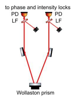
Figure 3.13: Removing Raman light before phase and intensity locks
