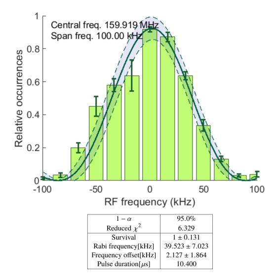
Figure 3.14: Microwave spectrum to measure light shift, without Raman beams
