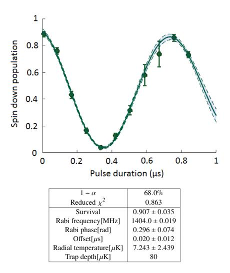
Figure 4.4: Rabi oscillation for Raman beams at 1.19mW
