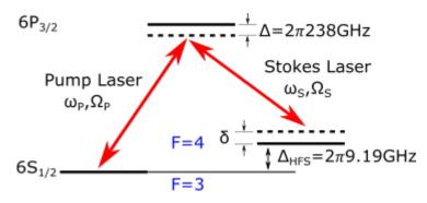
Figure 3.4: Laser settings and Caesium level scheme of Raman setup
