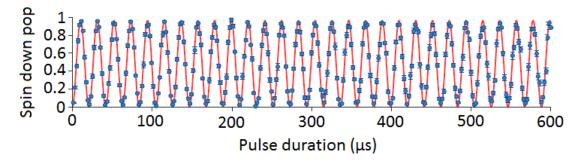
Figure 4.5: Microwave induced Rabi oscillations with  $\Omega_R = 48$ kHz
