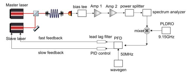
Figure 3.8: Optical phase lock loop as used in our system; Photo diode: Hamamatsu G4176-03, Bias tee: Mini-Circuits® ZX85-12G+, Amp 1: Kuhne Electronics KU LNA 922A, Amp 2: Miteq AFS5-08001200-40-10P-5, PLDRO: Resotech Inc, phase frequency detector: MC100EP140
