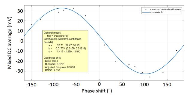
Figure 3.16: Phase noise measurement of the OPLL with fitting data
