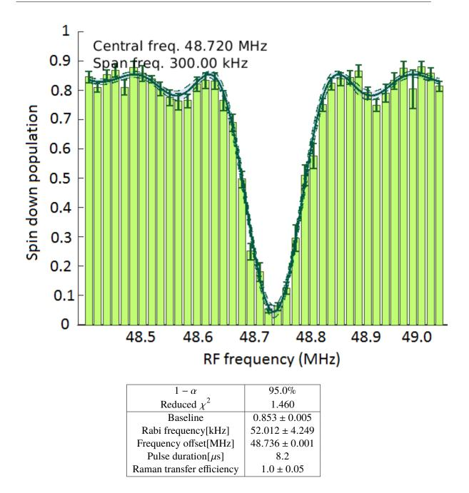
Figure 4.2: Raman spectrum with 8.2 $\mu$ s pulse length and 50 $\mu$ W of power per beam
