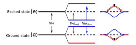
Figure 2.1: Light shifts of two-level atom interacting with an off resonant electromagnetic field
