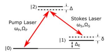
Figure 3.1: Lambda level scheme for Raman transitions
