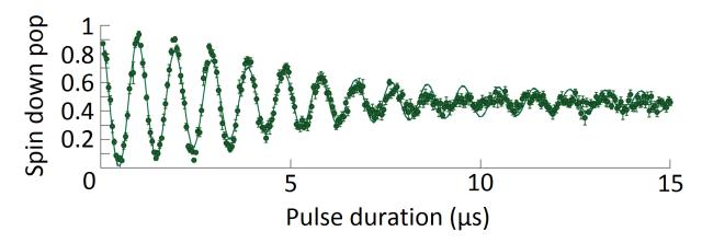
Figure 4.6: Rabi Oscillations induced by Raman beams at 1.1mW per beam
