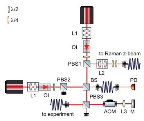
Figure 3.5: Optical components of the Raman setup
