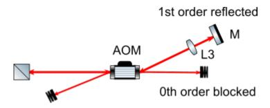
Figure 3.6: AOM in double pass configuration
