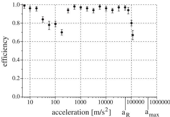
**FIGURE 7** Transportation efficiency for a displacement of 1 mm as a function of the acceleration. The transportation efficiency for a displacement of 1 mm remains well above 90% when the acceleration is varied over several orders of magnitude
