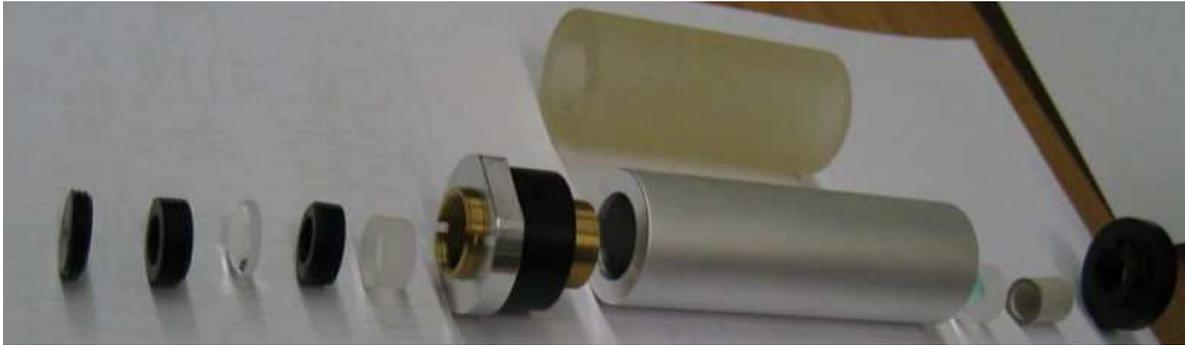
Figure 6.6: Components for building the cavity. From left to right: Pinhole, spacer, lens, spacer, mirror, brass screw thread, aluminum- e.g. zerodur rod, PIEZO tube, end cap.
