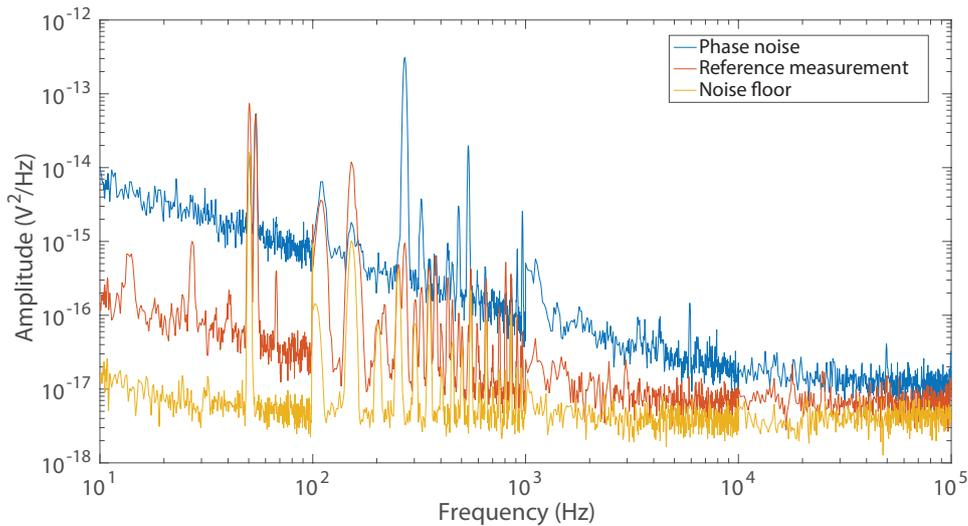
Figure 4.6: This figure shows the noise floor of our measurement setup in comparison to the phase noise measured and the reference measurement.
