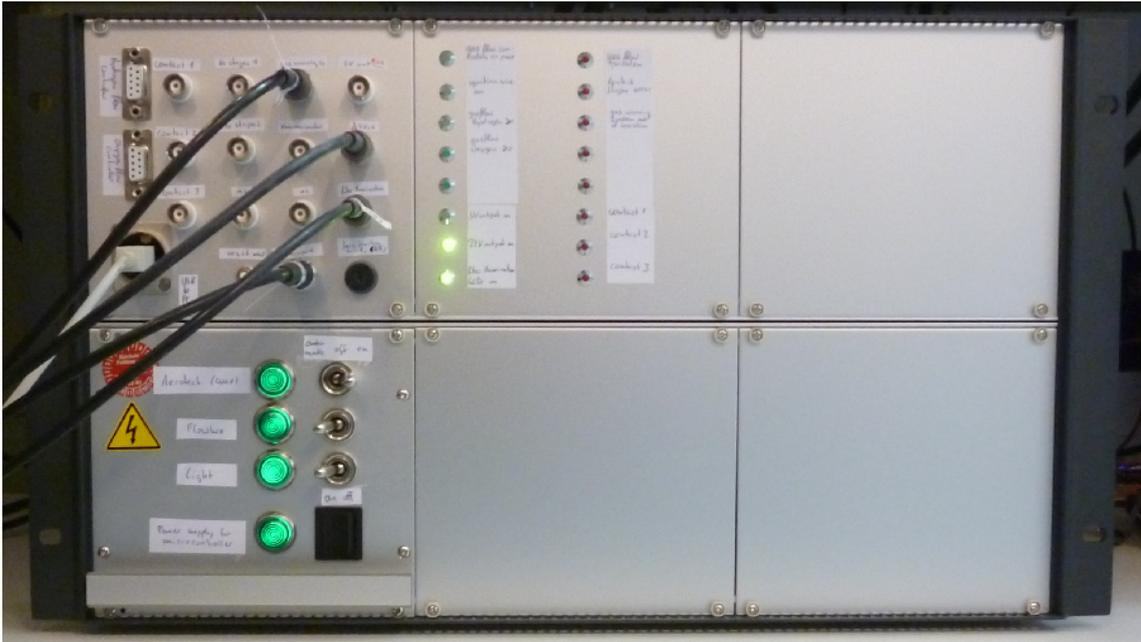
Figure 3.13. Central controller with power supplies and circuit boards. The front panel includes switches, connectors and indicators.
