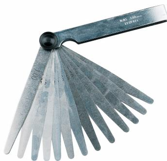
FIGURE 3.10: A typical feeler gauge, A simple and underrated tool but very helpful in assembling the components to have even tightenings.
