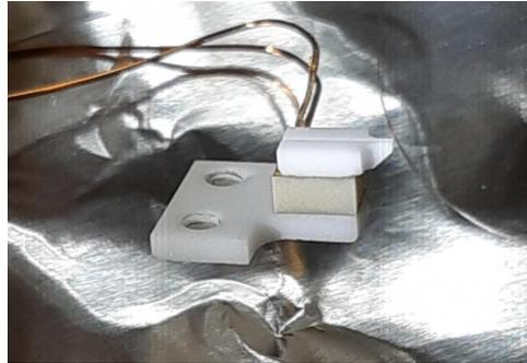
Figure 4.6: This figure shows the construction of the T-piece (below), the shear piezo (middle) and the V-groove (top), in which the fiber is placed for the cavity assembly.
