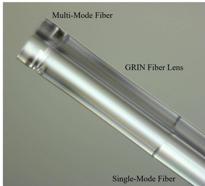
Figure 5.8: This figure shows a fiber assembly with a 780HP single-mode, a GIF625 GRIN and an FG105LCA multi-mode fiber.
