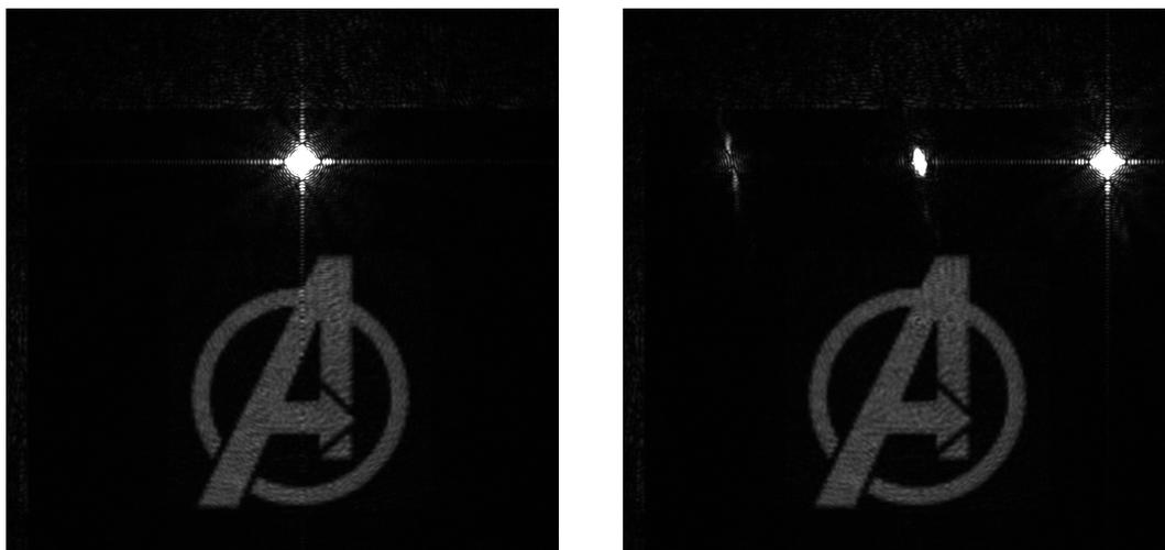
Fig. 5.1: Demo pattern "Averengers" with the zeroth-order spot untouched (left) and with attenuated zeroth-order spot (right). If the zeroth-order spot is too strong, its fringes affect the target pattern. The measured demo pattern has a size of  $1.2 \text{ mm} \times 1.2 \text{ mm}$ .
