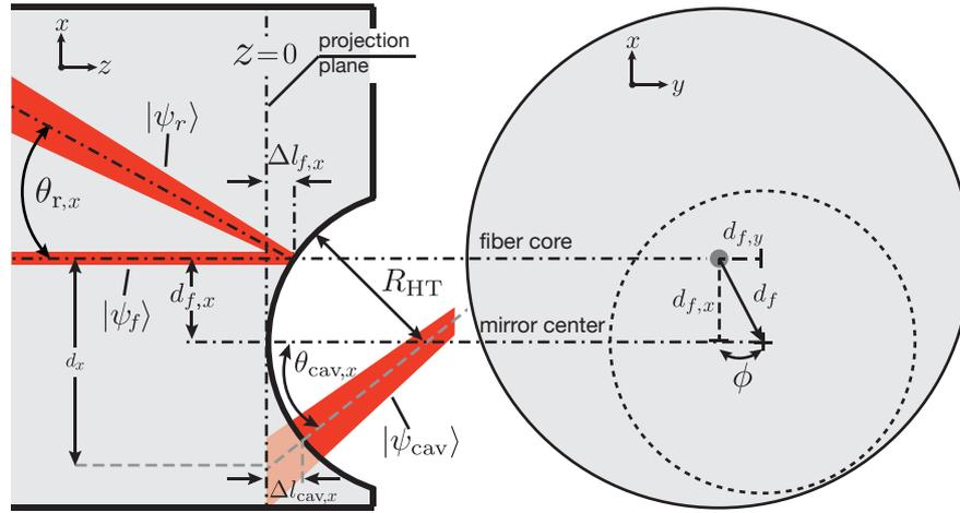
Figure B.1: Geometrical and optical considerations for the calculations of the overlap integrals. Black dotted lines represent fixed geometrical axes or planes, gray dashed lines represent axes that depend on the cavity-mode angle  $\theta_{\text{cav},x}$ . Displacements and angles have been exaggerated for a better clarity of the sketch.
