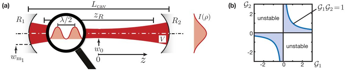
Figure 2.2: **(a)** Geometry of the fundamental  $\text{TEM}_{00}$  cavity mode. The radius of the Gaussian intensity profile diverges from the waist  $w_0$  and reaches a value  $w_m$  at the position of the mirrors. A standing-wave is formed due to the interference between counter-propagating circulating fields. **(b)** Stability diagram of an FP resonator. The colored region represents cavity geometries that allow the hosting of a stable mode.
