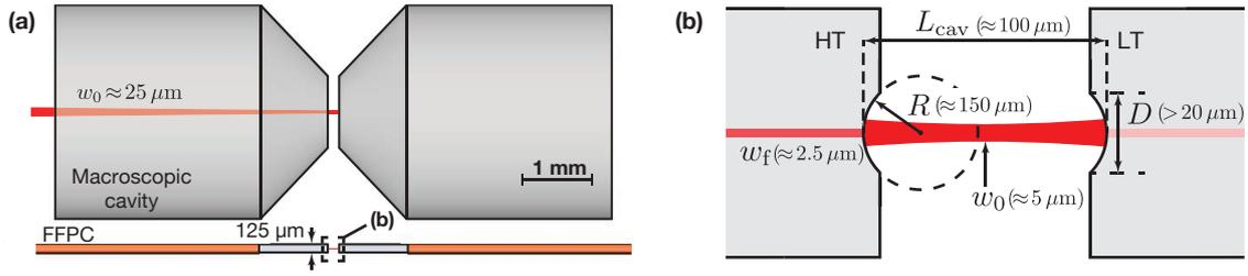
Figure 2.3: Fiber-based Fabry-Pérot Cavities (FFPCs). **(a)** Drawing to scale comparing standard macroscopic cavities (top) with fiber-based resonators (bottom). The latter provide a smaller waist, more optical access, intrinsic miniaturization and direct fiber coupling of the input/output without the need of external mode-matching optics. **(b)** Summary of the typical characteristics and requirements for our FFPC (not drawn to scale). HT: High Transmission mirror, LT: Low Transmission mirror.
