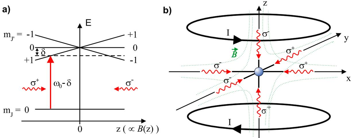
**Figure 4.1:** Principle of a Magneto-optical trap (MOT). a) The one-dimensional picture. Due to the Zeeman shifts of the atomic transitions in the inhomogeneous magnetic field, atoms at  $z < 0$  are closer to resonance with the  $\sigma^+$  laser beam than with the  $\sigma^-$  laser beam and are pushed toward the center of the trap. b) Extension to the three dimensional case. A quadrupole magnetic field is generated by coils in anti-Helmholtz configuration.
