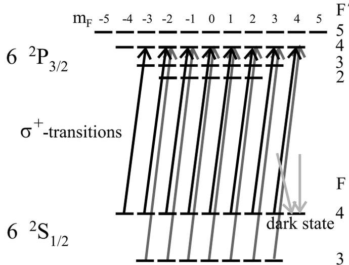
**Figure 3.2:** Optical pumping principle of the Cs atom in the dark state  $|F = +4, m_F = +4\rangle$ . The  $\sigma^+$  laser beams provide a polarized atomic beam.
