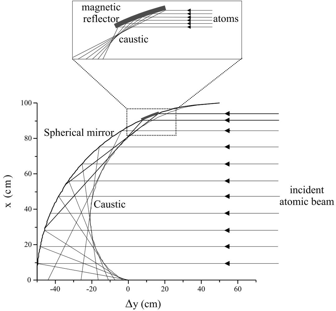
**Figure 5.2:** Aberrations of a spherical reflector with  $R = 100$  cm. The inset shows the caustic formation for small angle of incidence.
