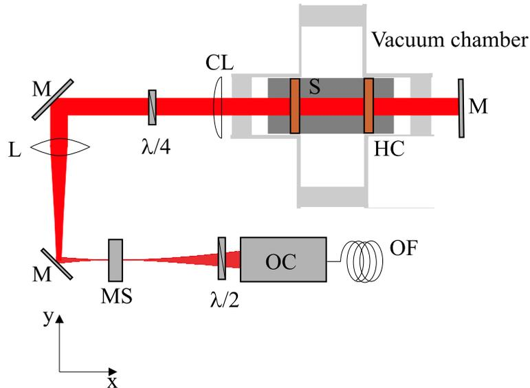
**Figure 4.12:** Optical pumping of the atomic beam in the dark state  $|F = 4, m_F = +4\rangle$ . MS: mechanical shutter, OF: optical fiber, OC: fiber out coupler, M: mirror, L: lens, CL: cylindrical convergent lens,  $\lambda/2$ : half-wave plate,  $\lambda/4$ : quarter-wave plate, HC: Helmholtz coils, S:  $\mu$ -metal shielding.
