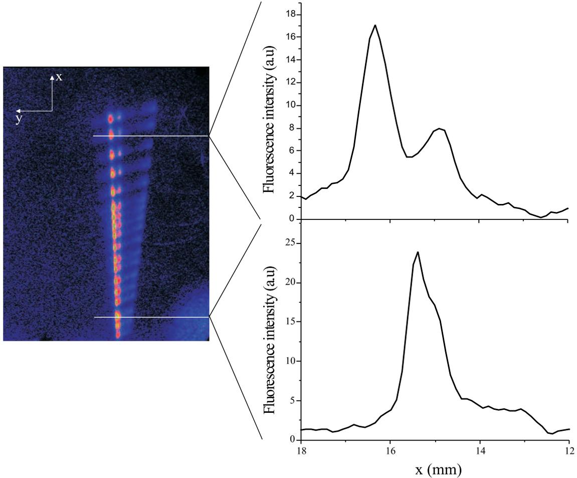
**Figure 5.13:** Behavior of the atomic beam width after two bounces on the magnetic videotape. Some atoms are bouncing twice whereas others bounce once. Atomic beam profiles located at  $37 \pm 6$  mm and  $67 \pm 6$  mm from the turning point.
