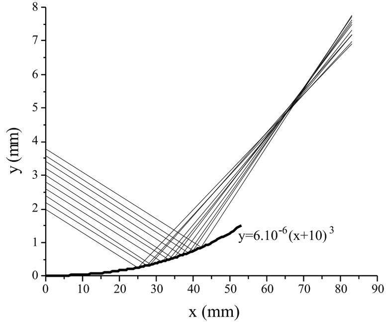
**Figure 5.20:** Atomic beam simulation of the focus realized after reflecting on the reflector given by Eq. (5.8). The atoms are deflected at  $\alpha_{defl} = 12^\circ$  and focus at  $f = 33$  mm.
