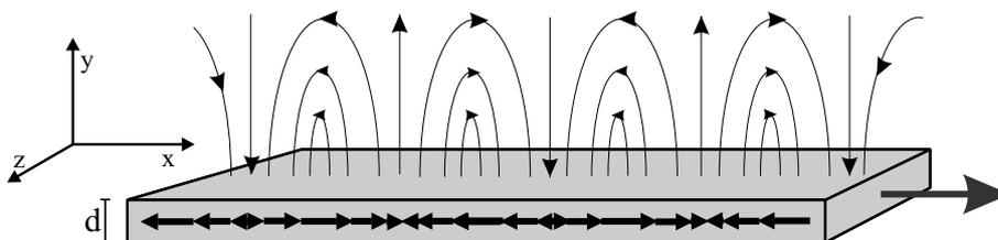
Figure 2.4: Sinusoidal magnetization along the  $x$ -axis in a videotape.
