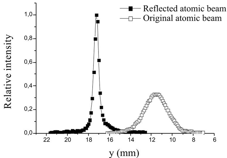
**Figure 5.10:** Lateral spatial compression of the trajectory of reflected atoms leading to an increase in the fluorescence intensity up to a factor 3. The atomic beam is deflected at  $\alpha_{defl} = (6.4 \pm 1.1)^\circ$ .
