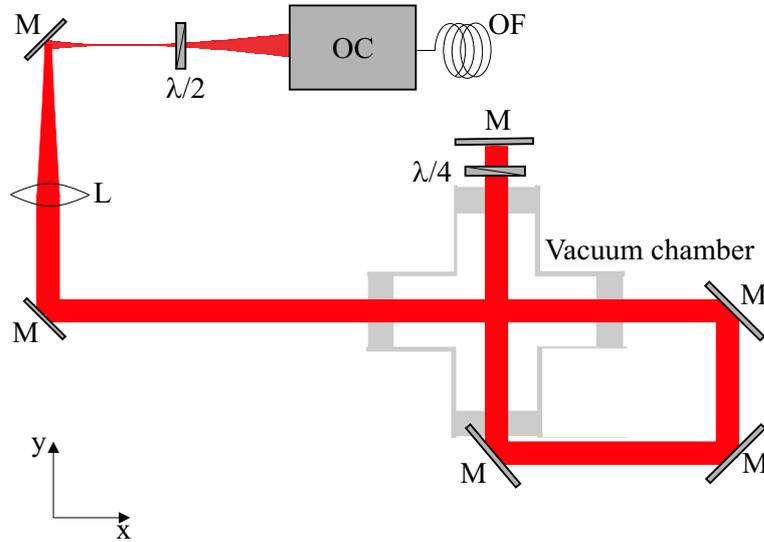
**Figure 4.9:** Two dimensional transverse collimation of the atomic beam. OF: optical fiber, OC: fiber out coupler, M: mirror, L: lens, PBS: polarized beam splitter, L: convergent lens,  $\lambda/2$ : half-wave plate,  $\lambda/4$ : quarter-wave plate.
