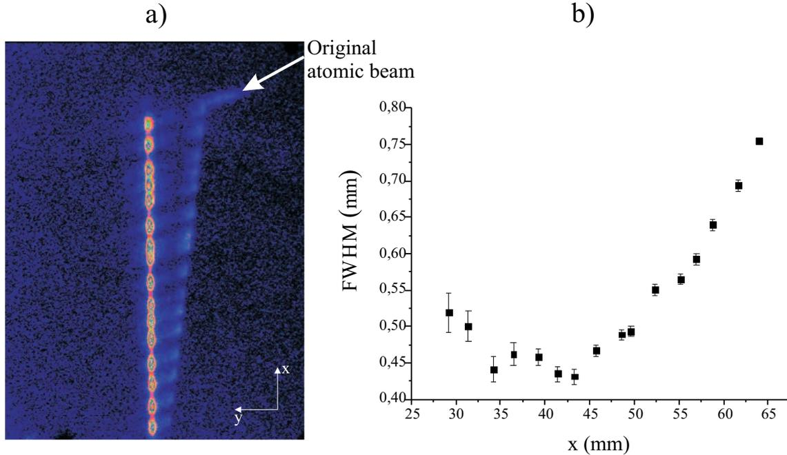
**Figure 5.9:** Focusing of the atomic beam. a) Added images of the reflected atomic beam and original atomic beam. b) Beam diameter of the reflected and focused atomic beam. The waist is clearly visible.
