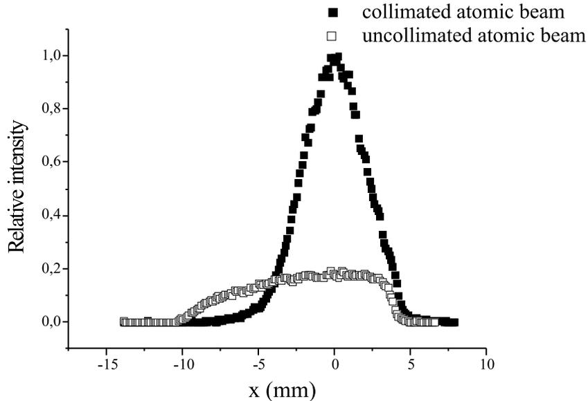
**Figure 4.10:** Relative intensity of atoms that have been transversely collimated. The uncollimated atomic beam is truncated by the hole in the  $\mu$ -metal shielding (see Section 4.5 and by the holder of the atomic mirror).
