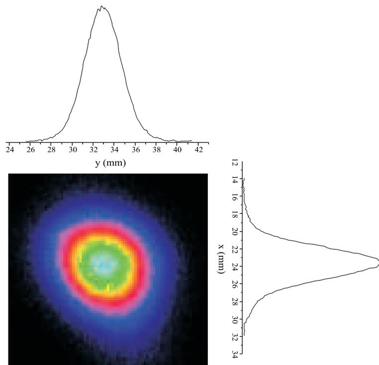
**Figure 4.11:** 2D-fluorescence profile of the collimated atomic beam.
