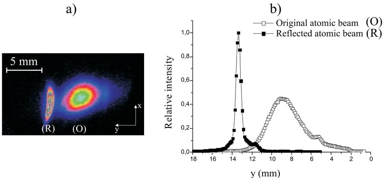
**Figure 5.8:** Enhancement of the atomic density in the atomic beam. a) Added images of the reflected atomic beam and original atomic beam. The label (R) is made for the reflected beam whereas (O) is for the original beam. b) Cross section along the  $y$ -axis showing the fluorescence intensity enhancement of the reflected atomic beam. The atoms are deflected at  $\alpha_{defl} = 7.8^\circ$ .
