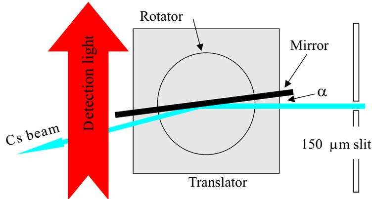
**Figure 3.5:** Experimental set-up for investigating reflection of atoms.
