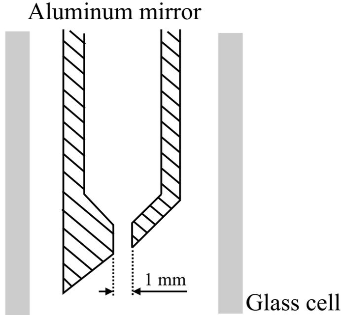
**Figure 4.5:** Aluminum mirror which reflects the plug beam at the center of the glass cell and enables to observe the atoms in the 2D-MOT. Without the plug beam, atoms leave the glass cell through the 1 mm hole.
