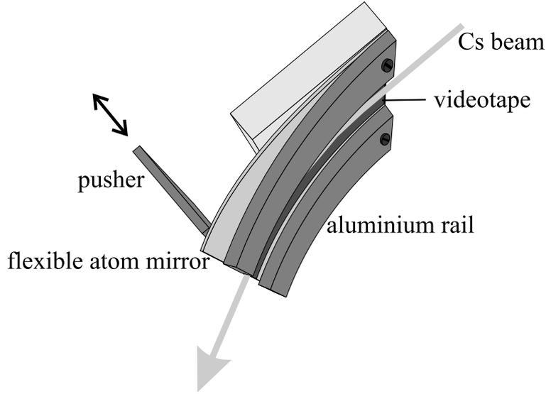
**Figure 3.11:** The sinusoidally recorded tape is glued to a metal strip that can be bent into a curve by pushing on the end as shown. The slow atomic beam can be deflected by multiple bounces through angles as large as  $23^\circ$ .
