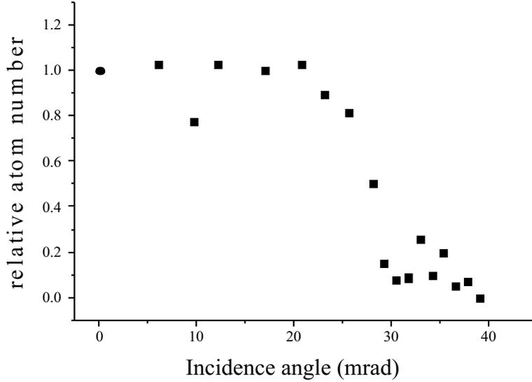
**Figure 3.6:** Relative flux of atoms that have been reflected from the tape as function of the angle of incidence at longitudinal velocity of 75 m/s. The reflectivity starts to decrease for angles larger than  $\sim 20^\circ$ . This provides information on the magnetic field at the surface.
