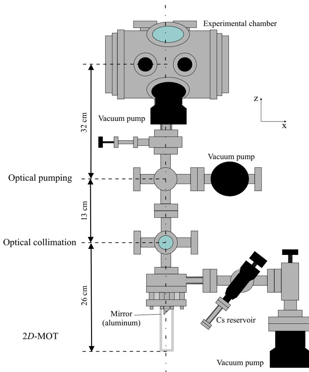
**Figure 4.4:** Mechanical assembly providing a low pressure environment. The differential pumping system at the bottom protects the rest of the apparatus from the Cs background pressure in the glass cell.
