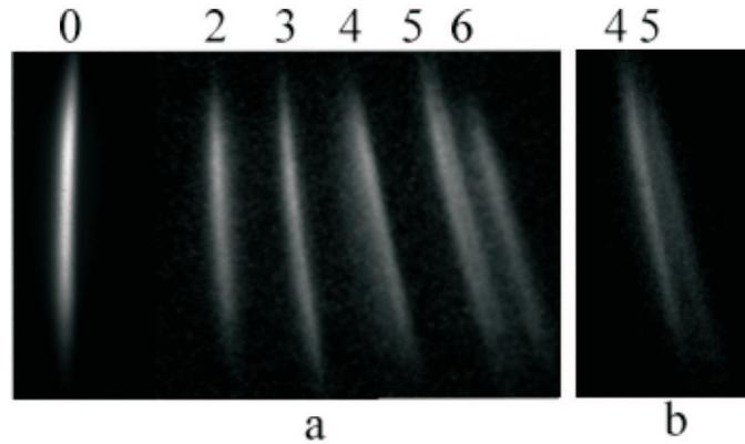
**Figure 3.12:** (a) Superimposed images of the deflected atomic beam for two, three, four, five and six reflections from the curved tape. The track labeled 0 is made by undeflected atoms. (b) A single image showing the double beam produced when some atoms have four reflections while others have five.
