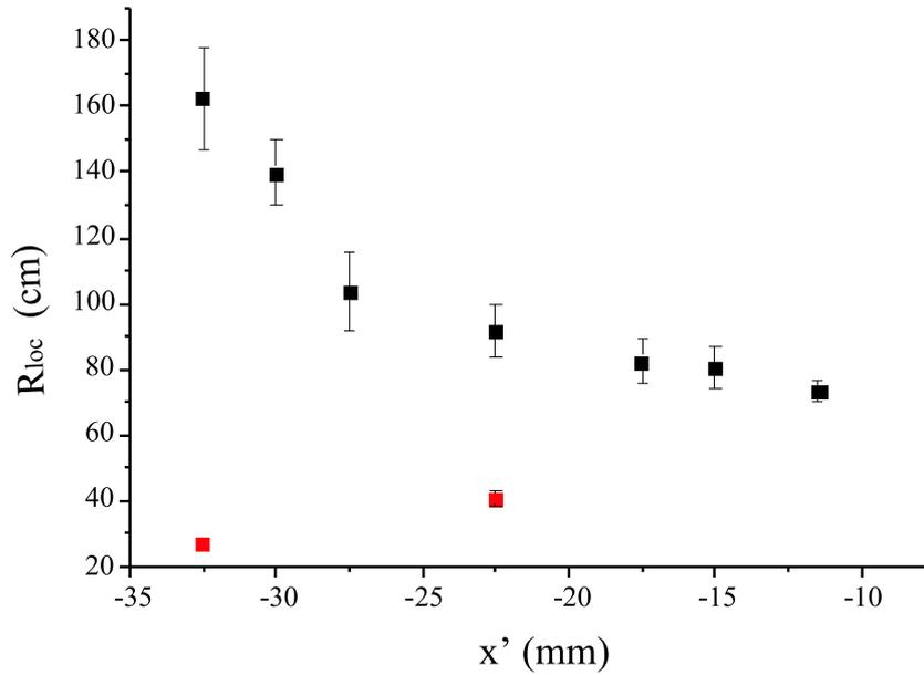
**Figure 5.18:** Determination of the radius of curvature  $R_{loc}$  of the videotape by shining at normal incidence a red laser diode onto its surface. The points at 27.4 cm and 40.5 cm correspond to reflections with the mechanical pusher for the points 5 and 8 of Figure 5.16.
