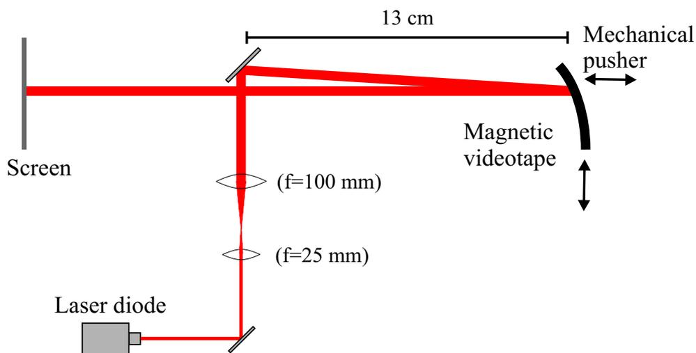
**Figure 5.17:** Investigation of the radius of curvature of the videotape.
