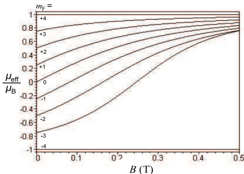
**Figure 2.1:** Effective magnetic moment for the  $|F = +4\rangle$  ground state of Cs according to Breit-Rabi formula.
