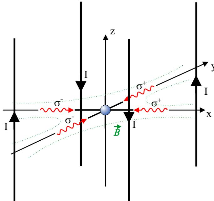
**Figure 4.2:** Scheme of the two dimensional MOT (2D-MOT). Alternating currents produce a two dimensional magnetic field in the  $x - y$  plane. Atoms are free to move along the  $z$ -direction since they are not subject to a restoring force.
