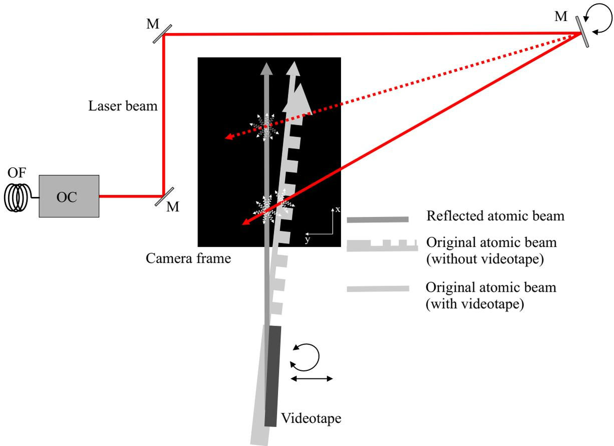
**Figure 5.7:** Principle of detection. We have represented the photon emission from the reflected and original atomic beams induced by the probe laser beam for two different positions of the mirror (M).
