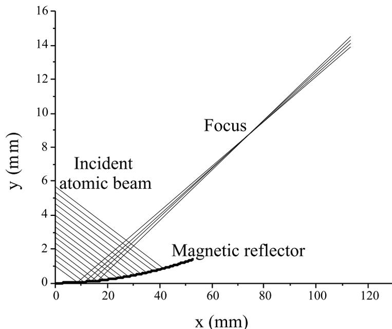
**Figure 5.3:** Focus of a reflected atomic beam on a spherical reflector with  $R = 101.2$  cm and an angle of incidence  $\alpha = 6.6^\circ$  with respect to the  $x$ -axis. Atoms with  $v_t > 2.1$  m/s stick on the mirror and are lost.
