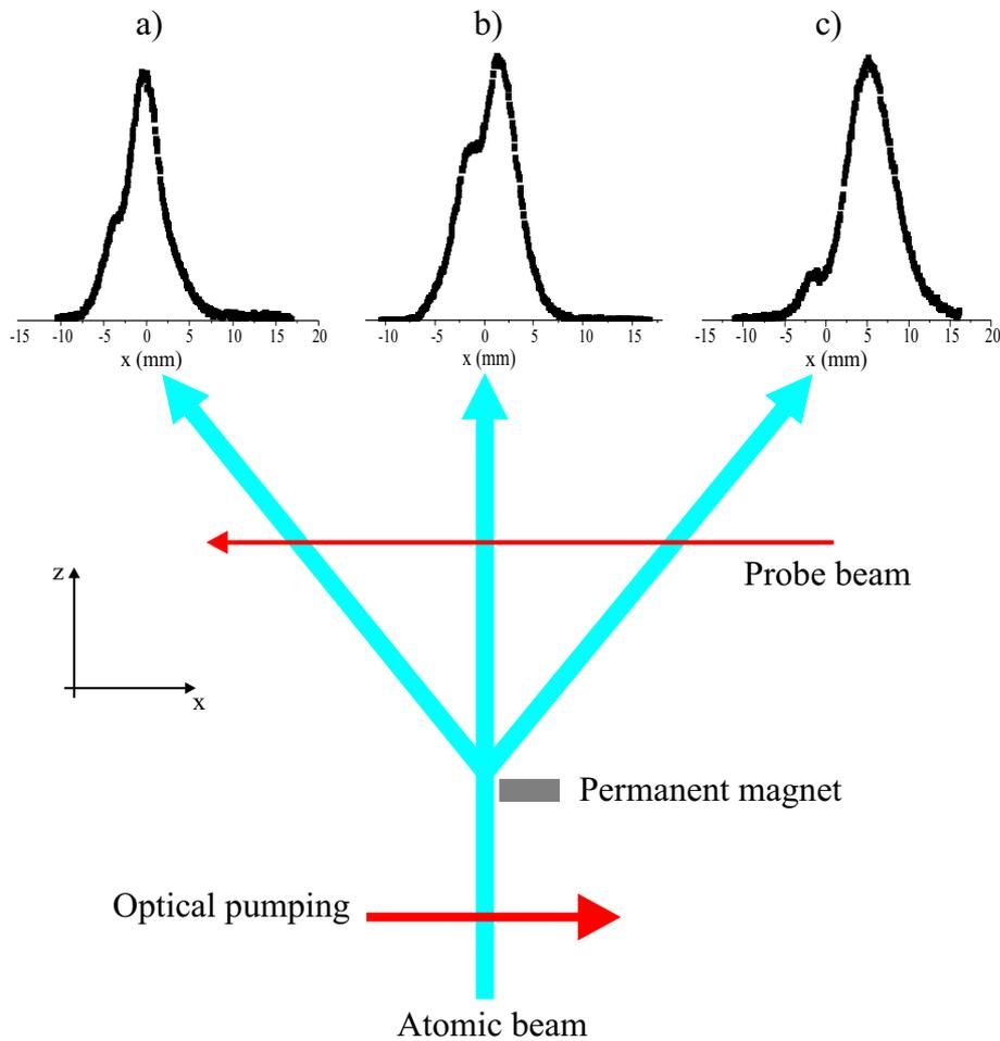
**Figure 4.13:** Plot of the relative flux of atoms depending on their position. a)  $\sigma^+$ -polarization. The atoms undergo a repulsive force. b) without optical pumping laser. The atomic beam is broadened due to the magnet. c)  $\sigma^-$ -polarization. The atomic beam is attracted by the permanent magnet.
