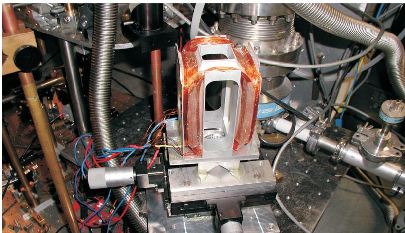
**Figure 4.7:** Picture of the racetrack-shaped magnetic field coil wound in the aluminum holder. The current flowing through the coil drives the resulting magnetic field on each side.
