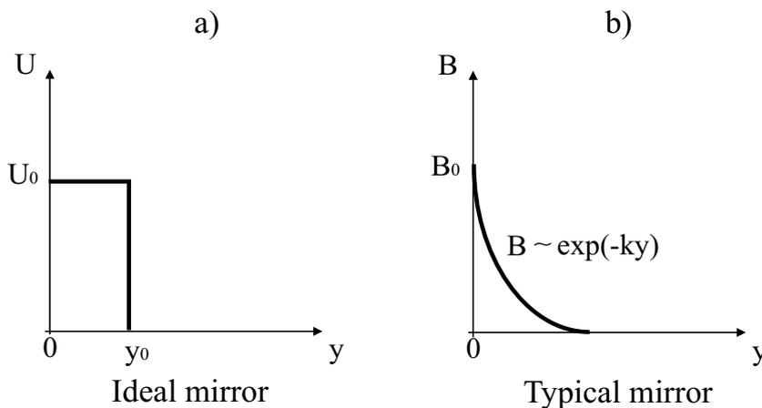
**Figure 2.2:** Magnetic potential for retro-reflecting atoms.
