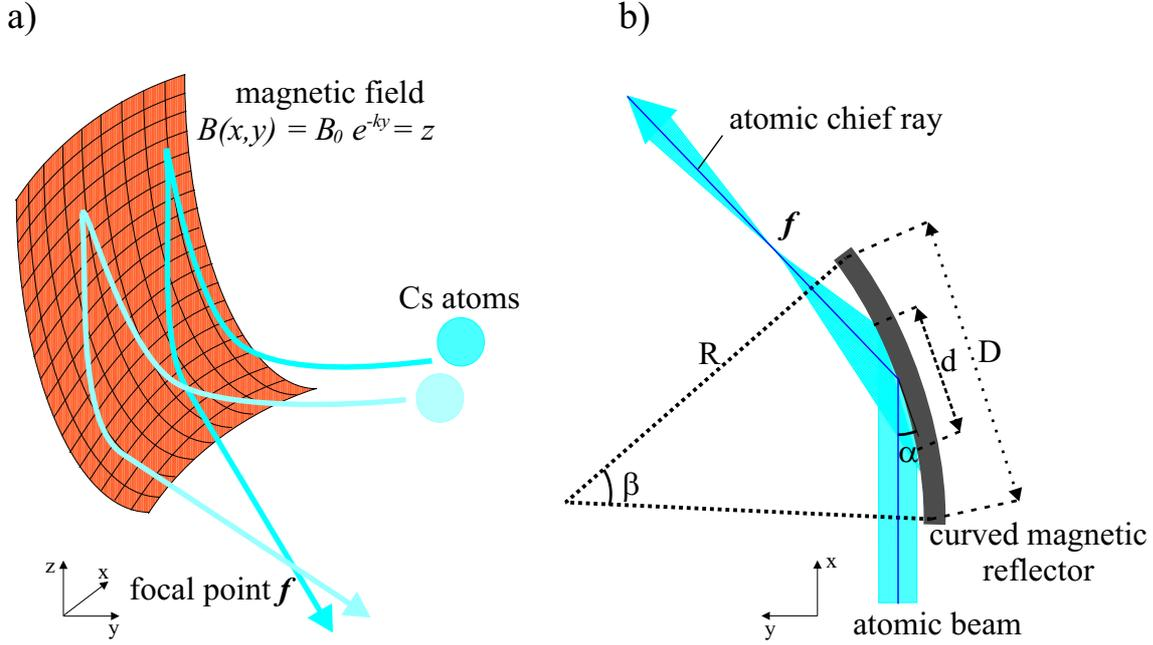
**Figure 5.1:** Focusing of atoms with a curved magnetic reflector. a) Atom trajectories of 2 atoms undergoing the repulsive magnetic force which cause them to cross at the point  $f$ . b) The atomic beam incident at an angle  $\alpha$  is reflected on a mirror and focused at a distance  $f$  from the turning point on the reflector.
