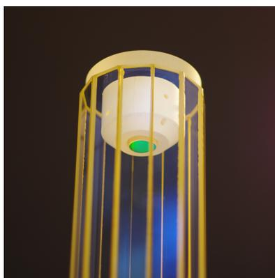
Photograph of the vacuum cell holding a large-numerical-aperture objective lens in its interior.
