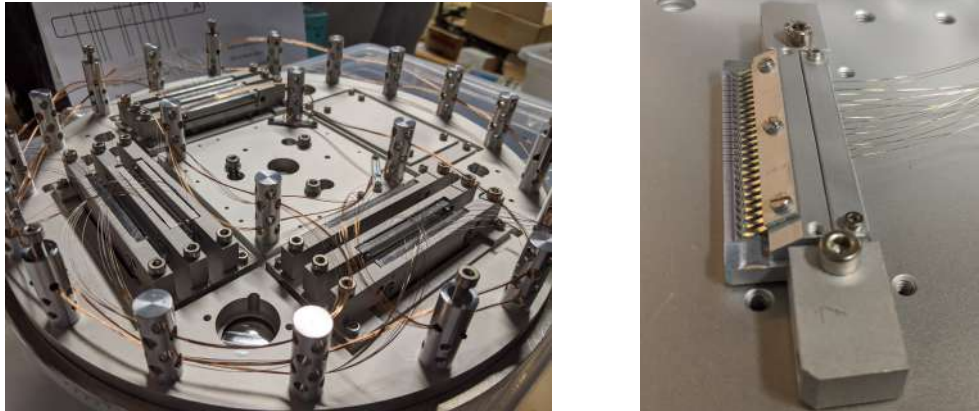
Figure 5.1: a) is an image of one of the coating disks used for coating dielectric mirrors on fibers, several fiber holders placed perpendicular to the coating disks and the fiber tails are fiddled around the disk and are clamped. b) is an image of one of the home built fiber holder that can store the fiber assemblies produced. The fibers are held in place by the clamping springs in each groove.
